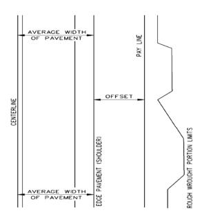
FIGURE 2-3 — Establishing a Pay Line Offset for Wrought Portion Highways
