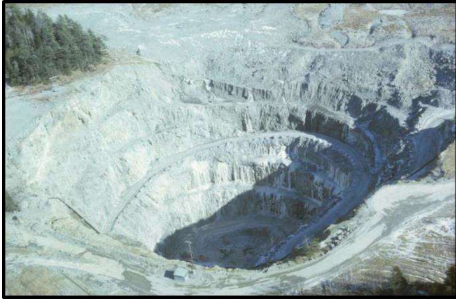
Small open pit, Callahan Mine, Maine, 1972. The pit was 360 feet deep, about 500 feet across. 800,000 tons of ore were mined from this site from 1968-1972.
