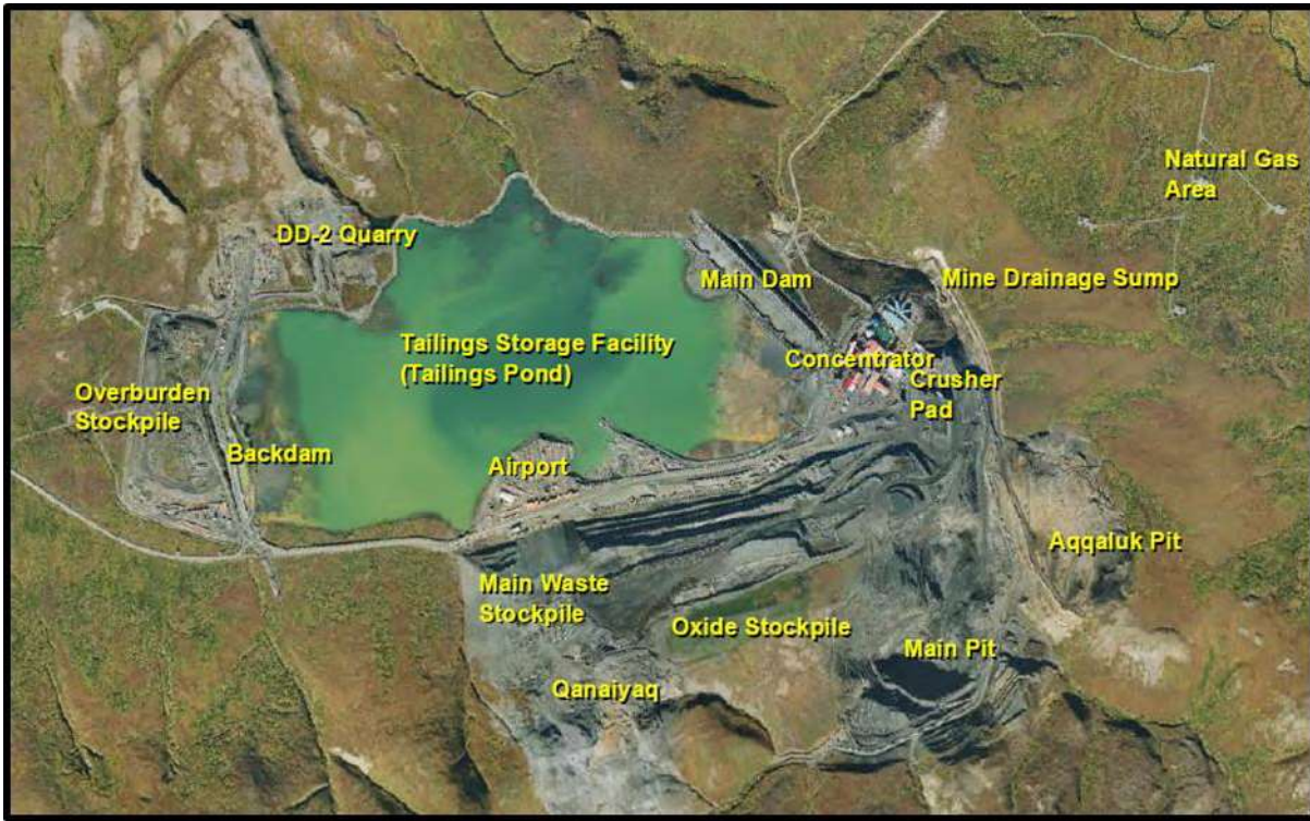
Components of a mine. Aerial view, showing ore extraction sites (pits), processing area (crusher, concentrator), waste storage areas (tailings and main waste), stockpiles, and water management facilities. This example is of a large open pit mine. ( Red Dog Mine, Alaska )
