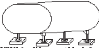
Figure 8-1 Tank footing & support for horizontal tanks of 350 gallons or less outside of buildings.
