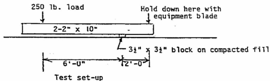
Place a 24" long straight edge or level on fill beside block. Center the straight edge on the block.
