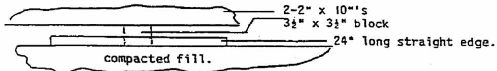
If the block sinks more than 3/8" with respect to the straight edge when the 250 lb. load is applied, more compaction is required
