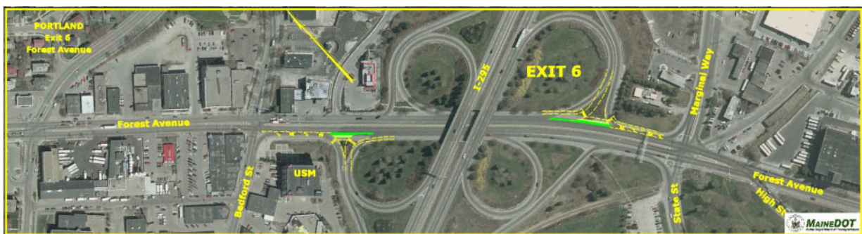
Figure 4.10: Exit 6 Forest Ave. Improvement Concept (enlarged in Appendix 23)
