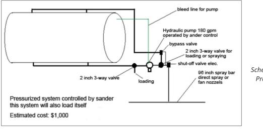
Schematic of a Typical Pressurized System For both systems, holding tanks, ball valves, fittings and piping will need to be made of UV resistant polyethylene similar in type to what is used in agriculture to prevent corrosion. Corrosion is a problem for electrical systems as well, so weatherize them as much as possible.
