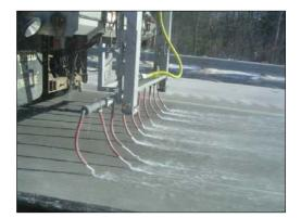
**How does it work?** Liquid application equipment disperses liquid chloride solutions directly to the pavement surface. This is accomplished by either spraying the solution on to the pavement surface with a pressurized system or allowing it to gravity feed to a piping manifold which distributes it across the traveled lane.
