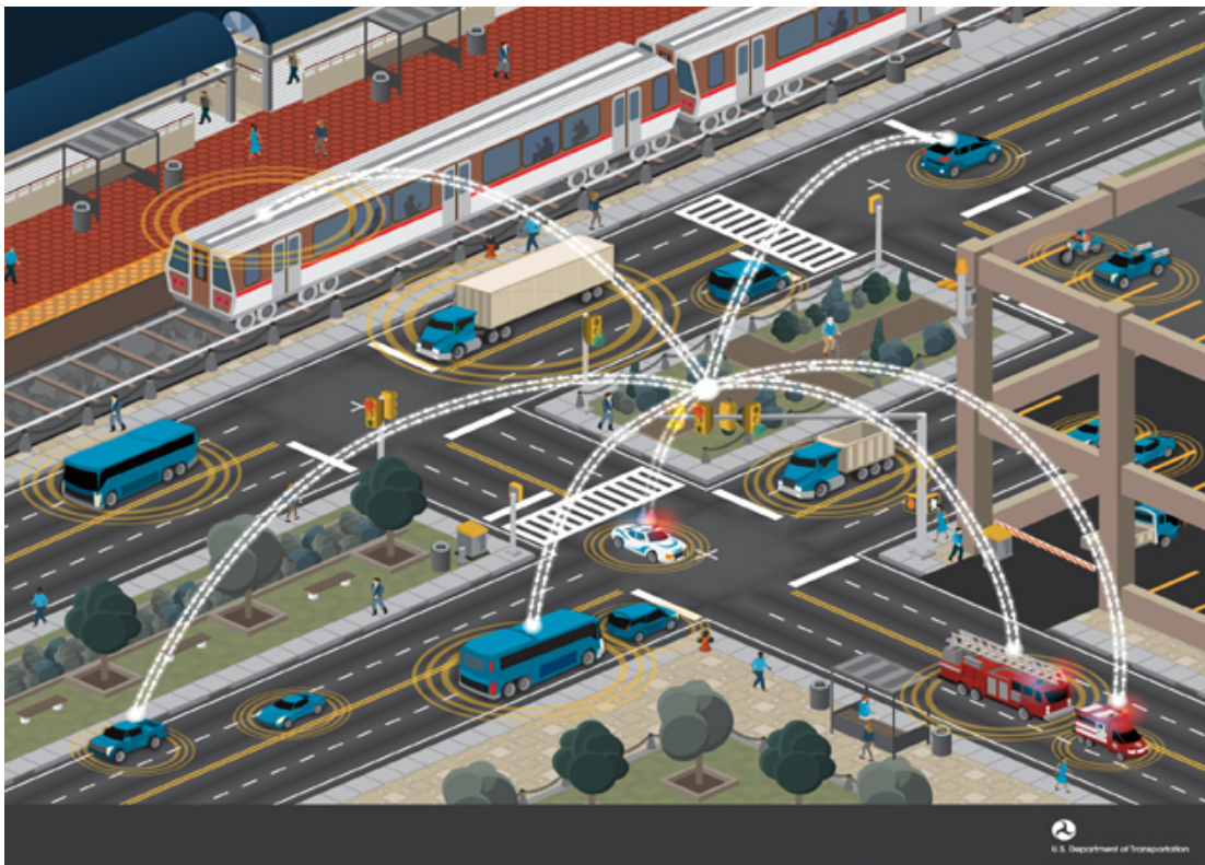
Figure 12. Connected Vehicles of All Types Communicating at a Traffic Signal
