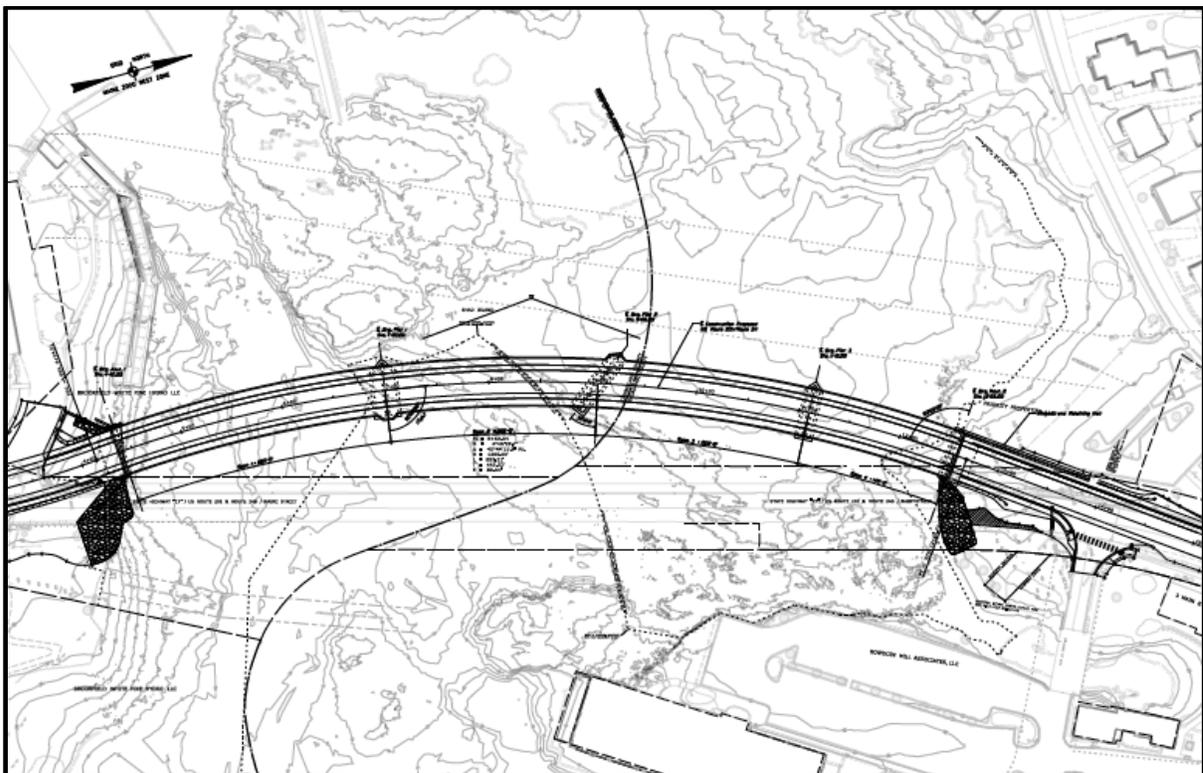
Figure 2-2. Proposed replacement Brunswick-Topsham Bridge showing locations of the three in-water concrete support piers.
