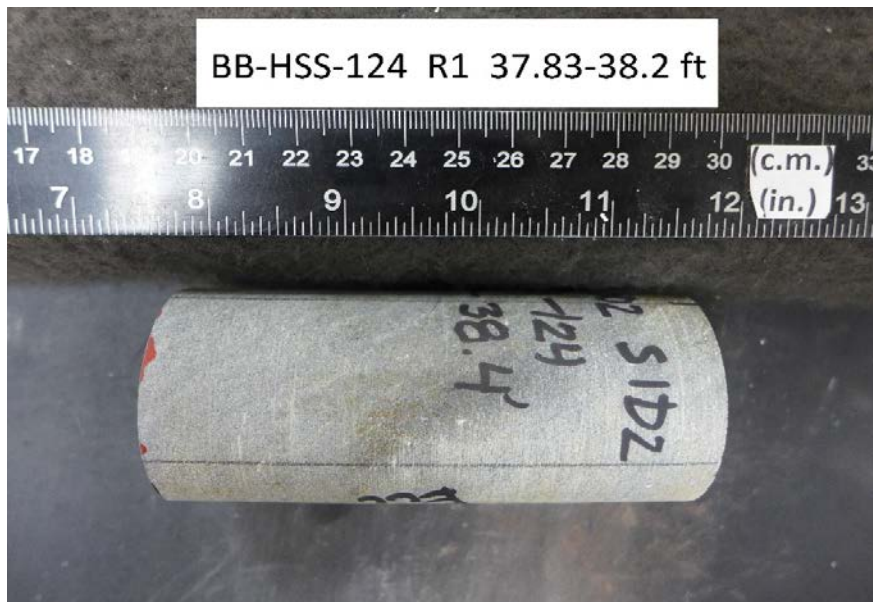
After cutting and grinding
