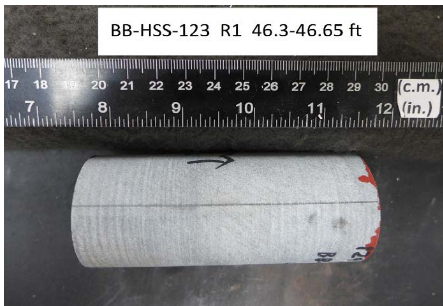
After cutting and grinding
