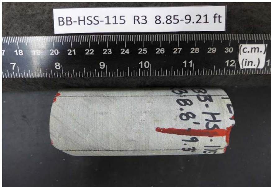
After cutting and grinding
