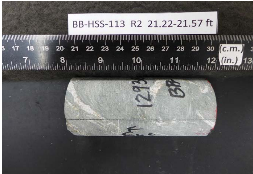
After cutting and grinding
