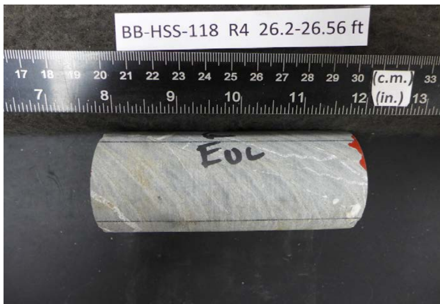
After cutting and grinding
