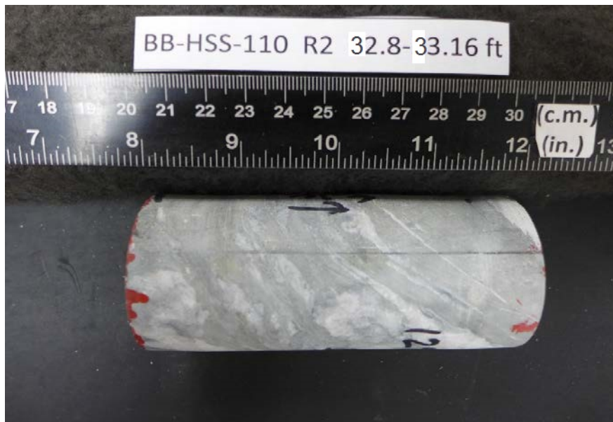
After cutting and grinding
