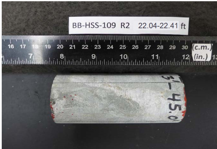
After cutting and grinding
