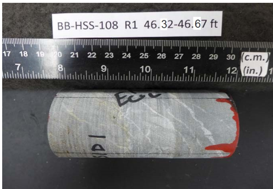
After cutting and grinding
