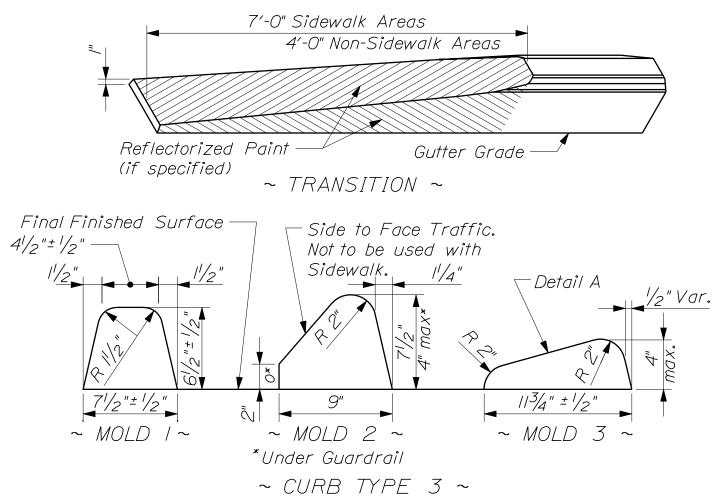
Curb Mold 2 or 3 shall be used in all situations except for where the curb forms the edge of the sidewalk. Mold I shall be used in conjunction with sidewalks or where there is a potential for sidewalks. Mold 3 shall be used in situations where the design speed exceeds 45 mph.
