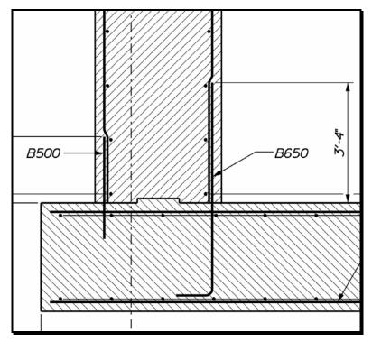
Figure 8-3 Unenclosed Hook
