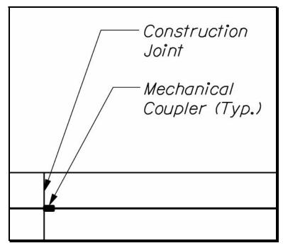
Figure 8-6 Mechanical Coupler
