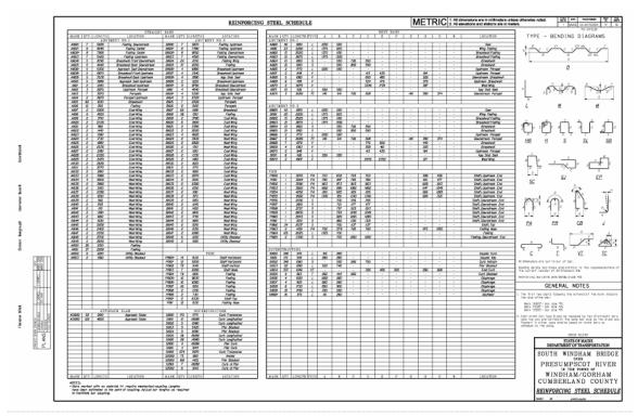
Figure 8-28 Reinforcing Steel Schedule
