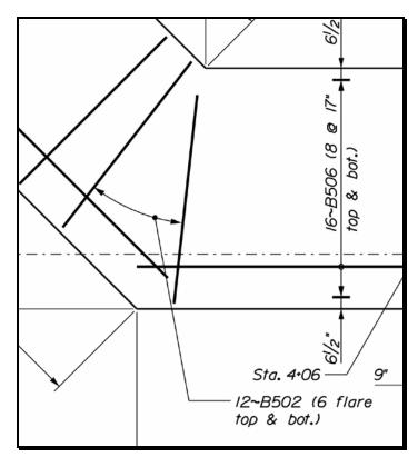
Figure 8-20 Flare Bars in Footing
