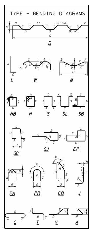
Figure 8-21 Bent Types
