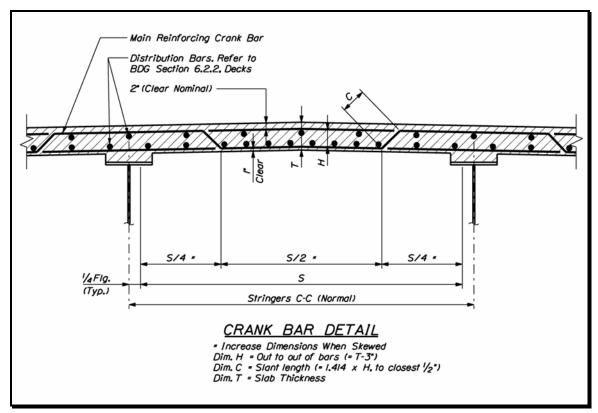
Figure 8-18 Crank Bar Detail
