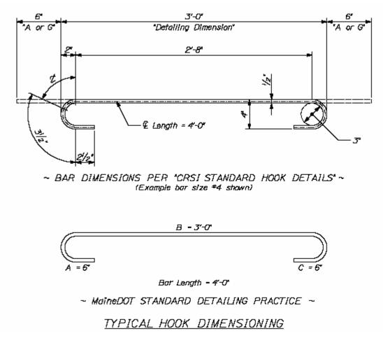
What if there is no bent type that matches your bar? First, ask a second opinion: there may be a way of cleverly using an existing bar type to show your bar – think of using a bar type with more legs than you need and setting some leg lengths to zero. If you do need a new bent type, simply give it a name and draw it on the rebar sheet. Label the legs, always starting with leg A, and ending with leg G. Use "R" for any radius, "H" for a height and "O" for an overall dimension.
