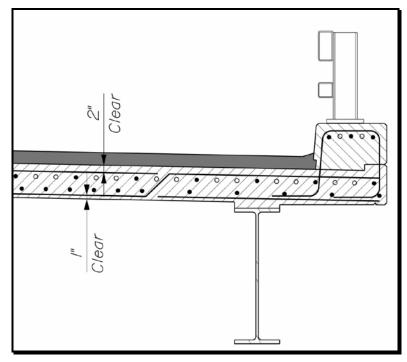
Figure 8-1 Cover Requirements in Superstructure
