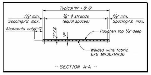
Figure 8-19 Welded Wire Fabric
