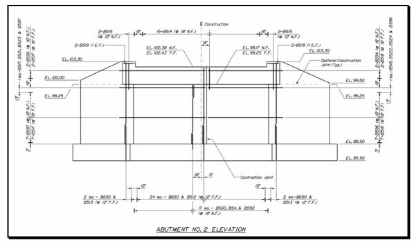
Figure 8-25 Spliced Sets at Multiple Locations
