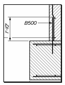
**Figure 8-7 Dowel Projection**
