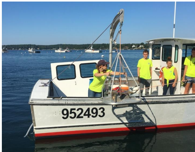
The Maine Coastal Mapping Initiative benthic ecologist, Ivy Ozmon, readies the sediment sampling apparatus for seafloor sampling. A Ponar dredge takes a sediment sample that is processed in the lab.
