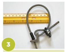
Measure the loop to insure the closing diameter is no less than 21/2".
