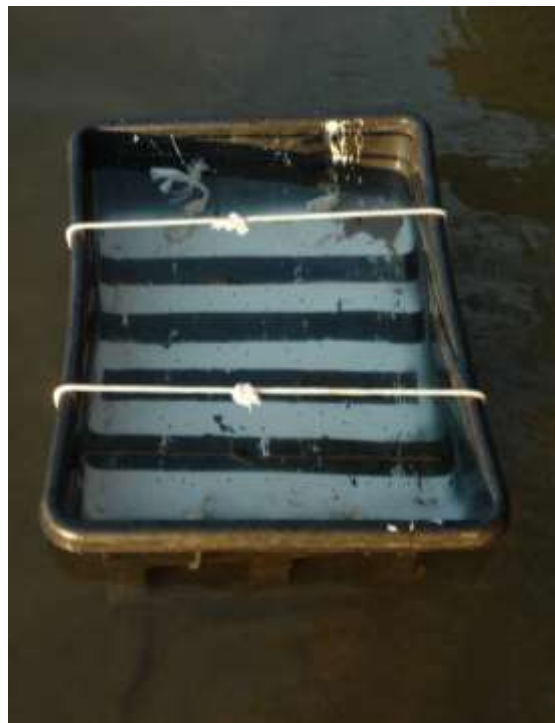
Figure 1. This bin also has a second set of ropes that run perpendicular to the ropes that are strung through the cinder block holes. Extra fastenings or weight should be used in wave-prone areas.
