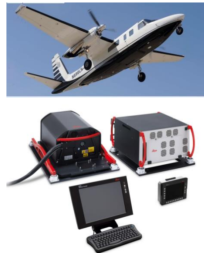
Figure 52: One of Quantum Spatial twin-aircraft and a Leica ALS sensor.
