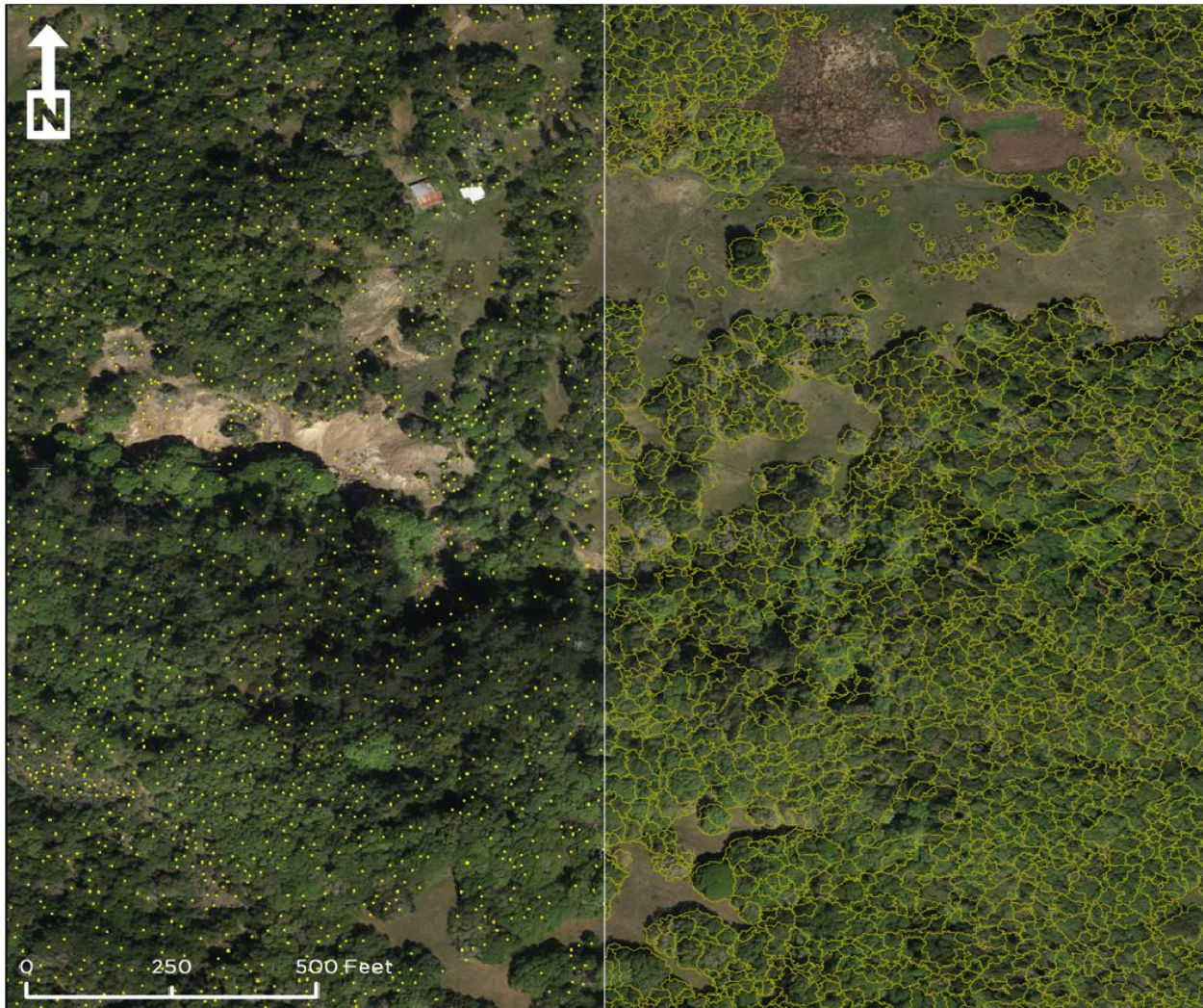
Figure 32: Map of tree top points (left) and vegetation and tree top polygons (right) overlying 3 inch orthophotos within the SSU Osborn Preserve Study Area.
