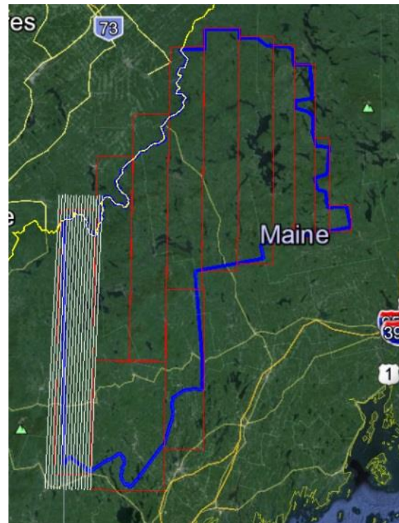
Figure 43: Geiger flight plan. Collection bricks in red and sample flight lines (white) within each brick.
