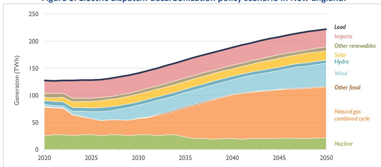
Combined cycle combustion technology uses both turbine technology and a steam generator to maximize the production of electricity from natural gas combustion. The “other renewables” category includes biomass, municipal solid waste, demand response, landfill gas, and other miscellaneous resources.
