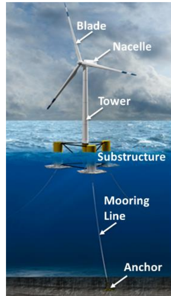
Parts of a Floating Offshore Wind Turbine
