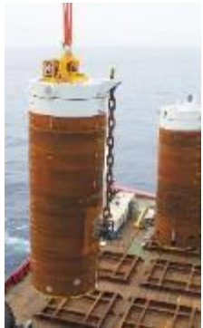
Uplift at anchor requires suction piles or similar
