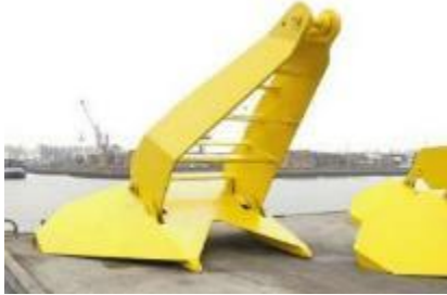
Line on seabed allows drag embedment anchors
