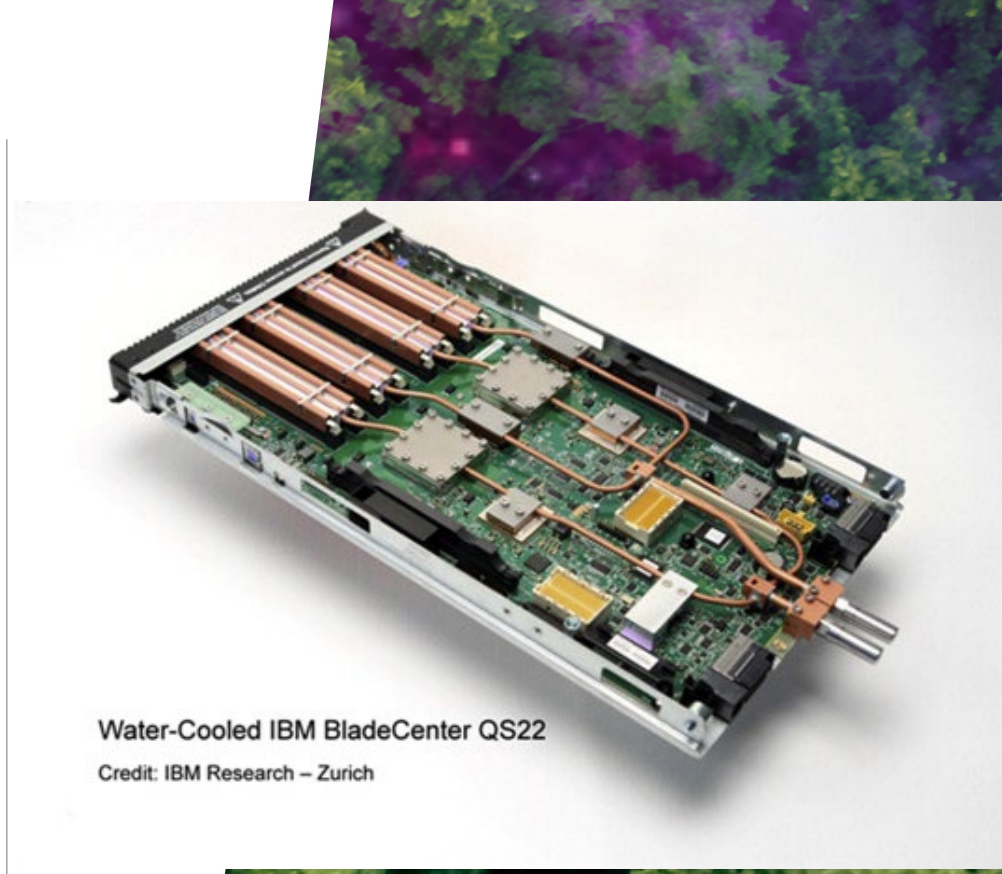
Fig. 9: Water-cooled IBM BladeCenter QS22. Source: Zimmerman et al. (2012) .
