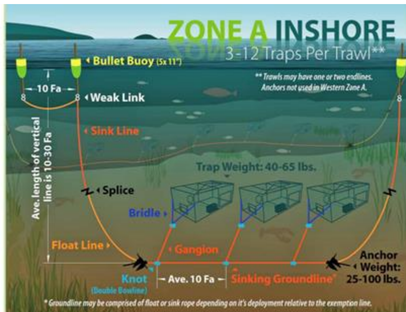
Figure 5. Zone A inshore trawl configuration
