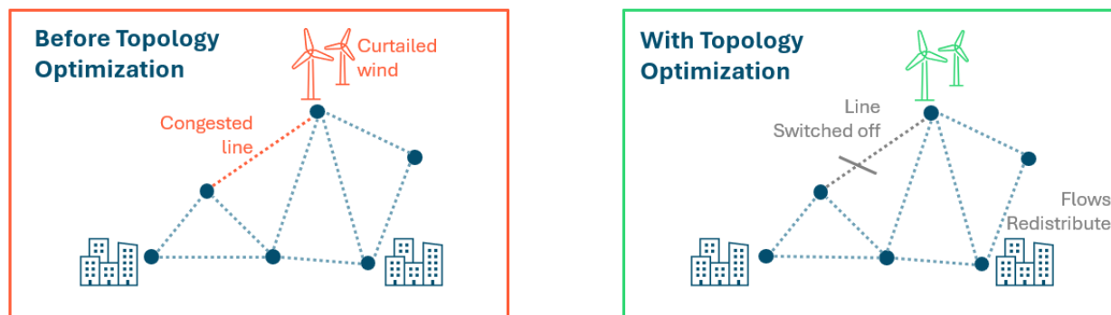
Figure 24. Illustration of Topology Optimization Impact
