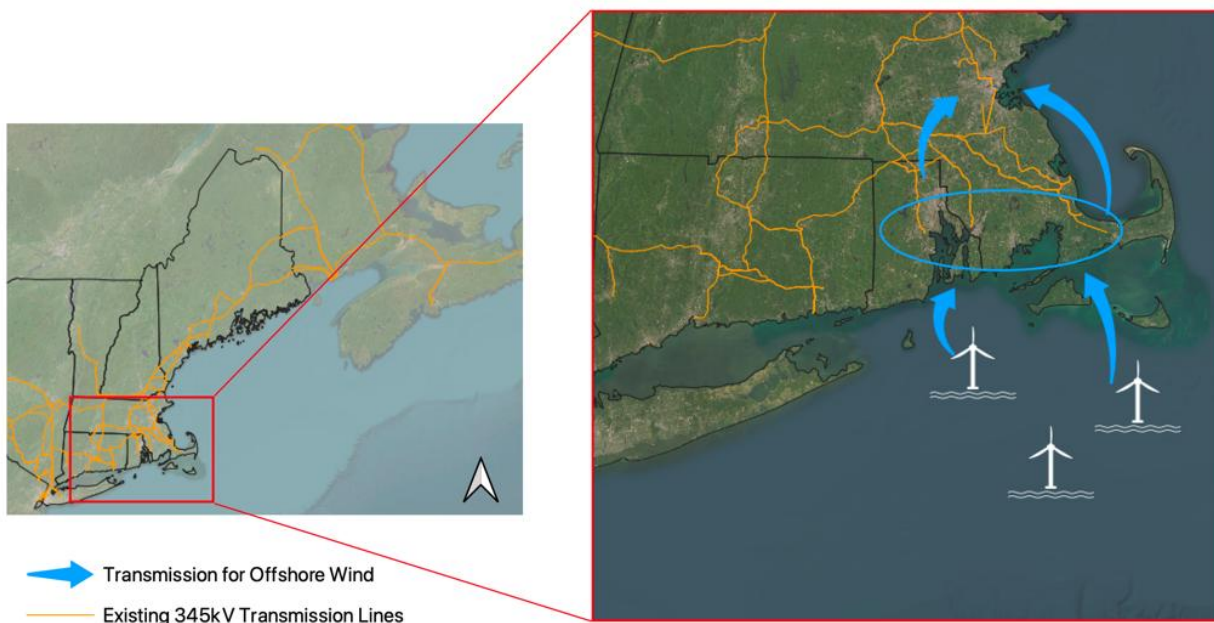
Figure 5: Illustrative Upgrades to Enable Offshore Wind Integration
