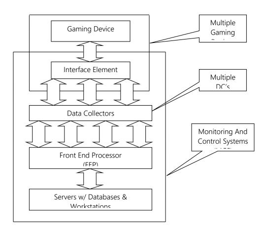
In the illustration above, this standard applies to all components referenced other than the Gaming Device. The requirements for the Gaming Device are defined in GLI-11. This document will only concern communications from the Gaming Device to the MCS, and not in the reverse order, with the exception of the Ticket/Voucher Validation System Requirements that are incorporated within Chapter 4.
