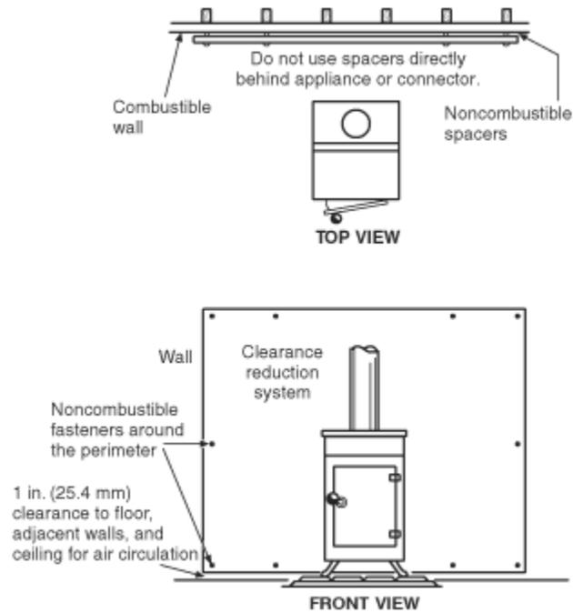
FIGURE 12.6.2.1(a) Clearance Reduction System — Fastener Location.
