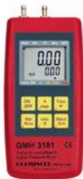
Figure 32. Photograph of Greisinger model GMH 3181-01 handheld manometer.
