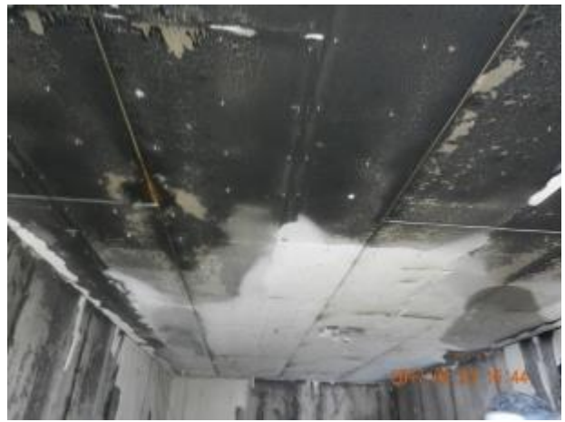
(f) after Test 1-2 – gypsum board remained: 1 layer on ceiling; 2 layers on walls
