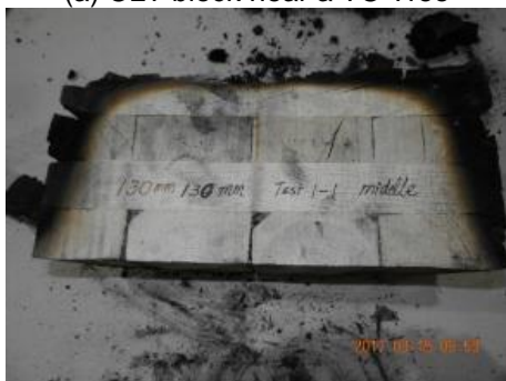
(c) middle block near TC Tree 6 charred 45 mm
