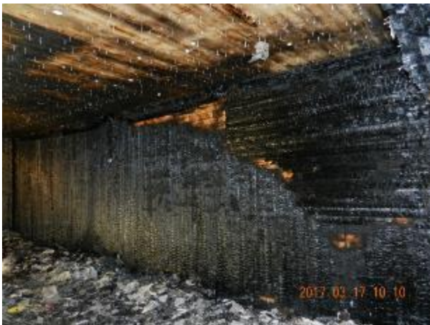
(c) W1 and ceiling after Test 1-3.
