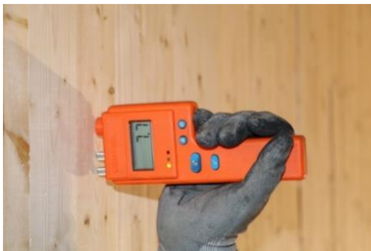
Figure 10. Measurement of panel moisture content using Delmhorst (BD-2100) meter.
