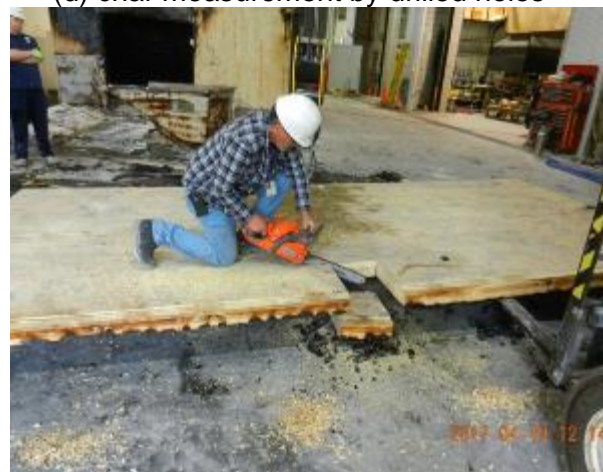
(f) cutting sample for char measurement
