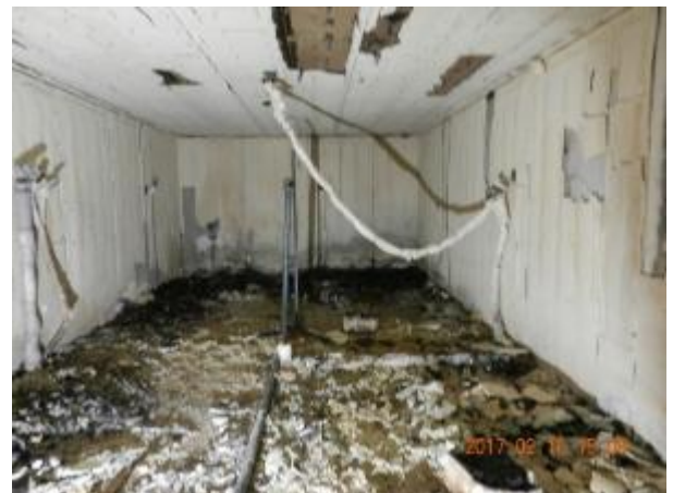
(f) after Test 1-1 – gypsum board remained: 2 layers on ceiling; 3 layers on walls
