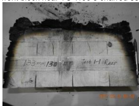
(d) rear block near TC Tree 4 charred 42 mm
