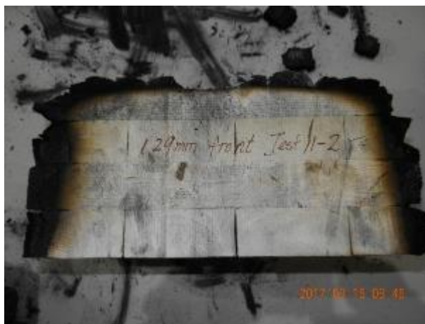
(b) front block near TC Tree 3 charred 46 mm
