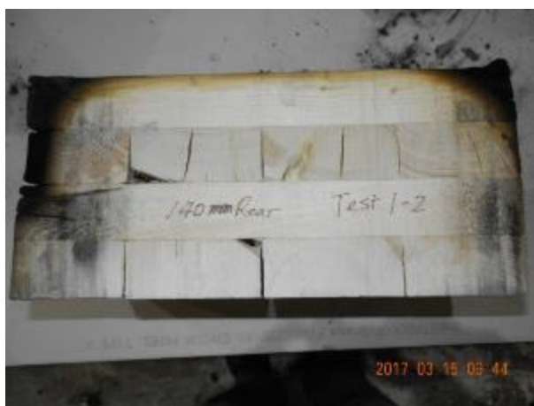
(d) rear block near TC Tree 4 charred 35 mm
