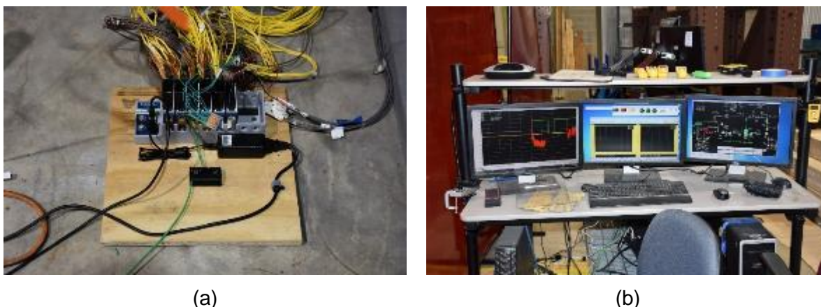
Figure 28. Photographs of (a) cDAQ-9188 chassis populated with I/O-modules and (b) setup used to control the NFRL calorimeter and data acquisition.
