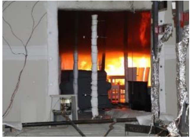
(b) W1 wall ignited at 9 min.
