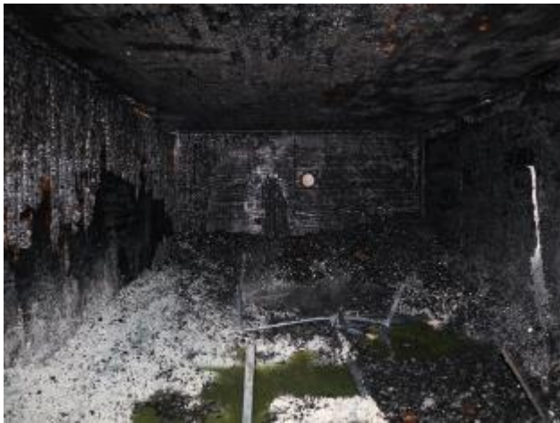
(a) interior of CLT compartment after Test 1-5
