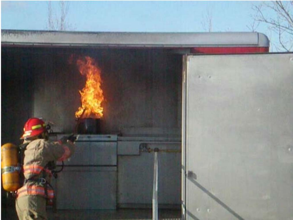
**Figure 18: Results After Cup of Water Is Poured Over Cooking Oil Fire**
