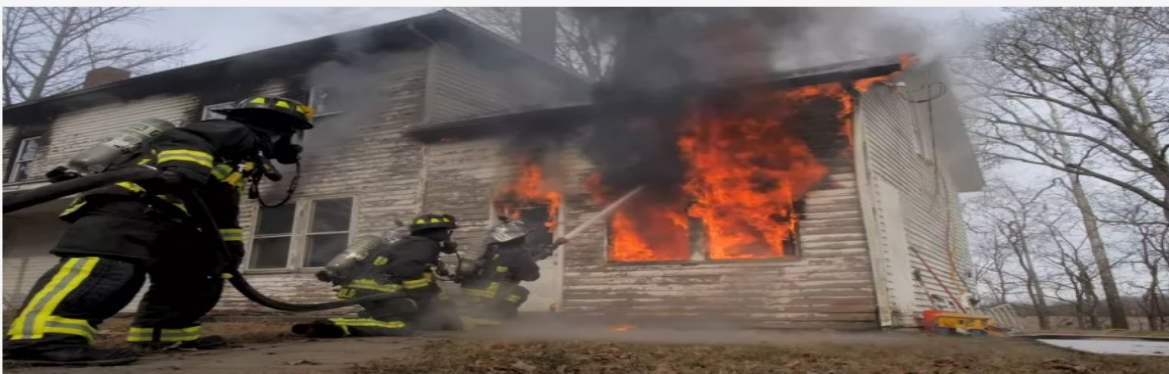
Firefighters battle an experimental home fire in 2018, as part of a study conducted by UL's Fire Safety Research Institute. FSRI research has shown that furniture foam and other oil-based synthetic products burn so quickly and produce so much toxic smoke that home fires can turn deadly well before firefighters arrive. FSRI is part of UL Research Institutes, an independent safety science organization.
