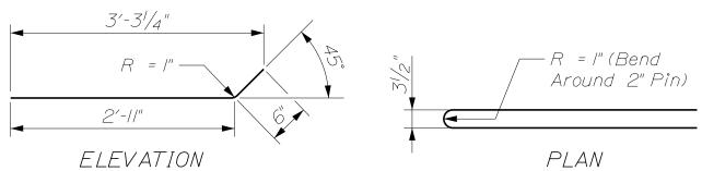
3⁄4" ♦ A36 Loop Bar (Hot Dip Galvanized After Fabrication Per ASTM AI23 or AASHTO M III)
