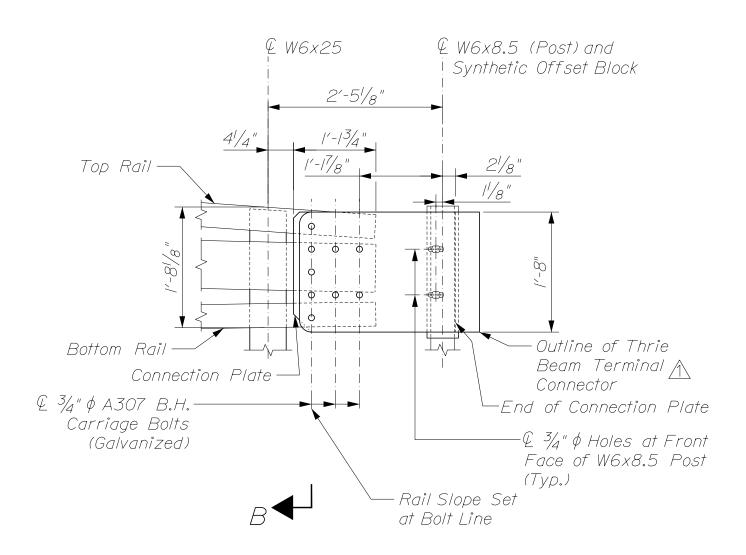
~ DETAIL "A" ~ (Overlapping of Double Nested Thrie-Beam not Shown for Clarity)
