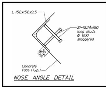
**Figure 3-33 Solid Pier Nose Angle Detail****Intro:** Cross section through structural steel nose angle**Sheet up:** Belongs below to the right of the Pier Section**Scale:** 1½”.**Draw:**
