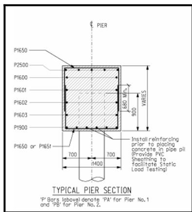
**Intro:** Cross section through pier.**Sheet up:** Belongs to the right of the pier plan**Scale:** 1/2" or 3/8" (Typically 2x the plan/elevation scale.)**Draw:**
