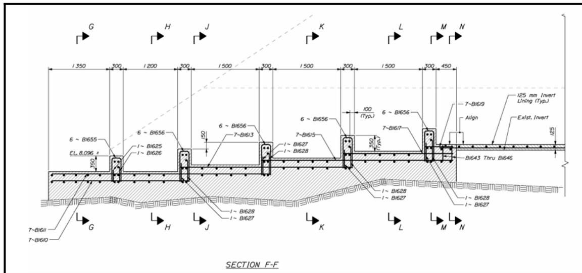
Figure 7-22 Weir Elevation 2
