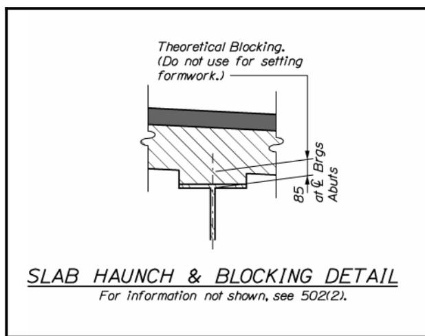
Figure 4-9 Steel Girder Slab Haunch and Blocking Detail
