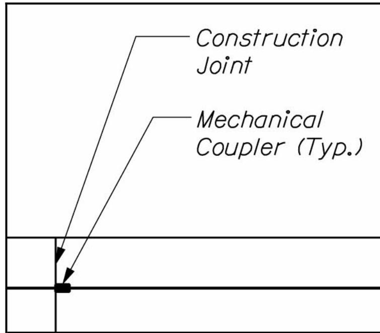
Figure 8-6 Mechanical Coupler
