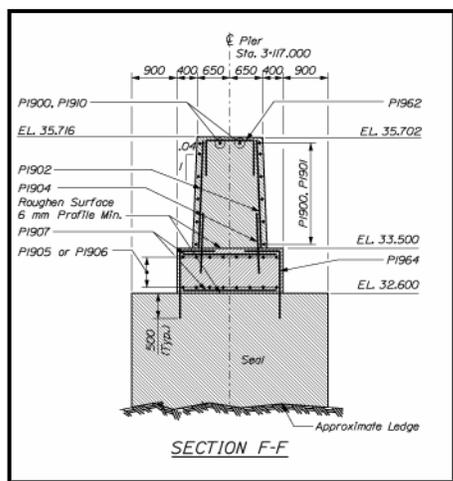
**Figure 3-32 Solid Pier Section**
