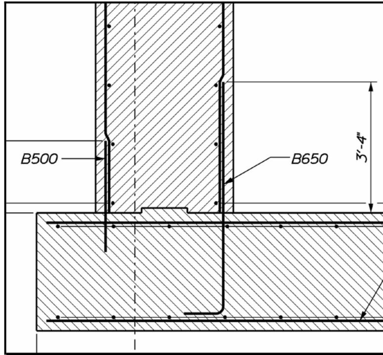
Figure 8-3 Unenclosed Hook
