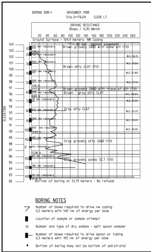
Figure 7-7 Boring Logs
