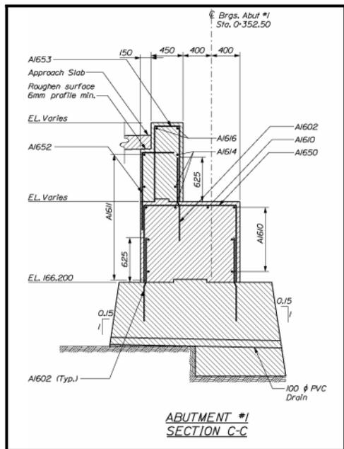
**Figure 3-19 Abutment Section**
