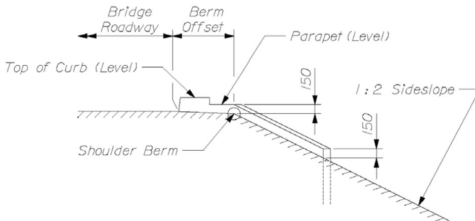
(Elevation at Back of Abutment)
