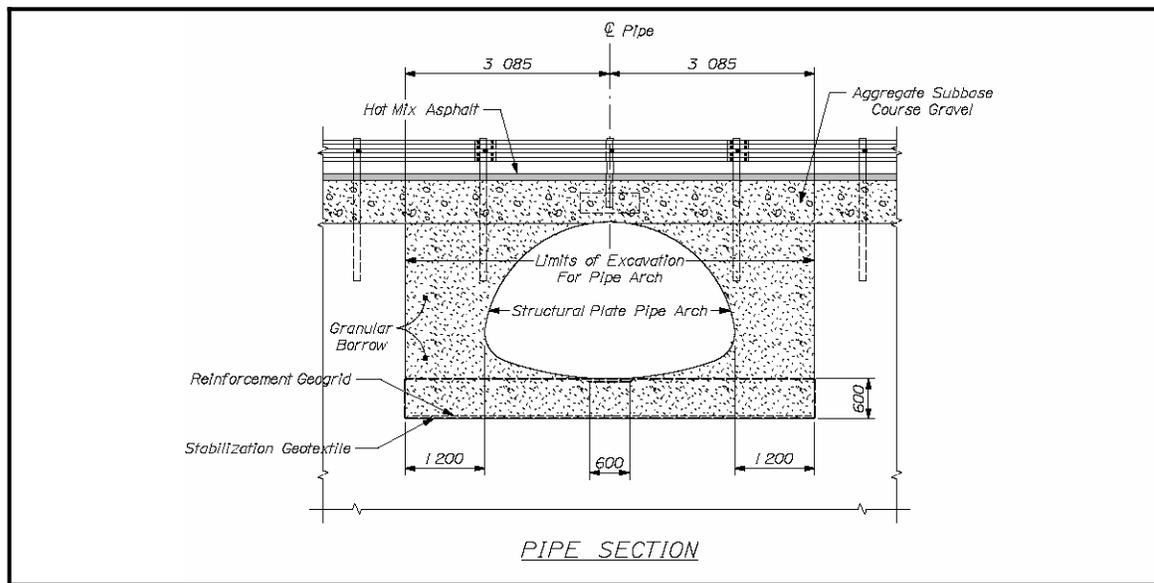
**Figure 5-5 Structural Plate Pipe Arch Typical Section**
