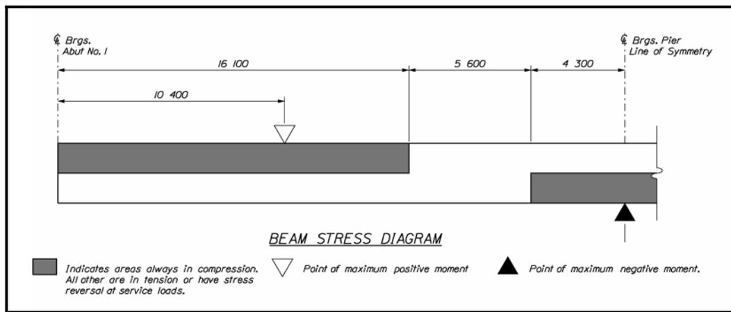
**Figure 4-14 Steel Girder Beam Stress Type Diagram**
