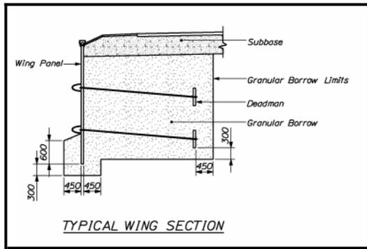
**Figure 5-16 Structural Plate Box Culvert Typical Wing Section**
