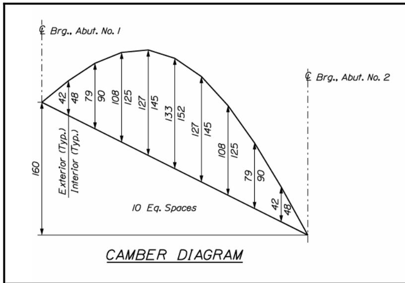
Figure 4-8 Camber Diagram
