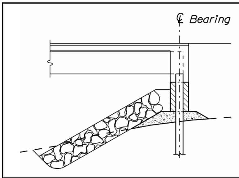
Figure 3-1 Integral Abutment
