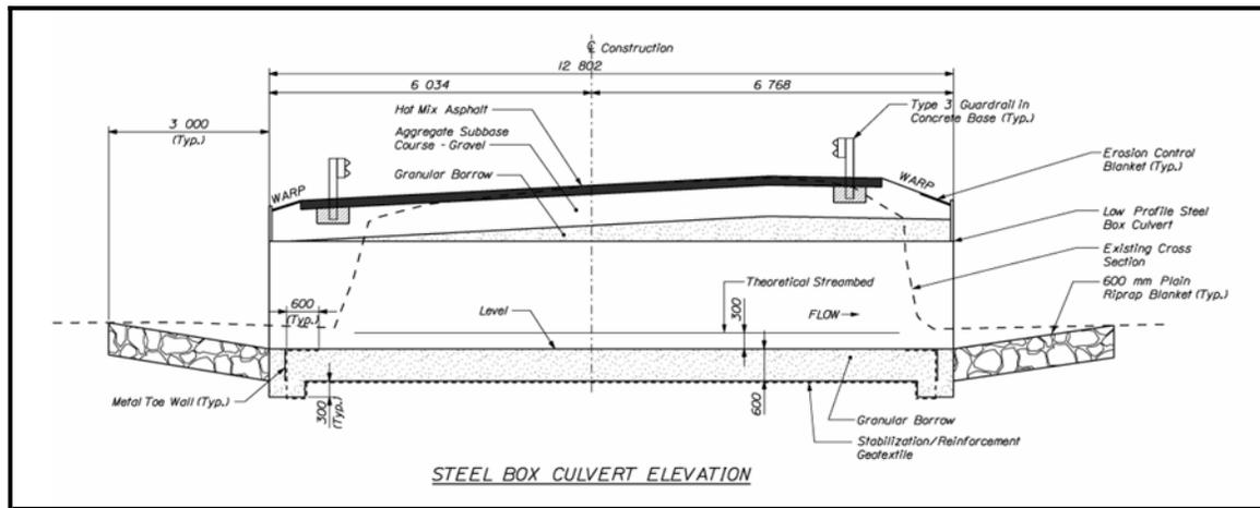
**Figure 5-13 Structural Plate Box Culvert Longitudinal Section**
