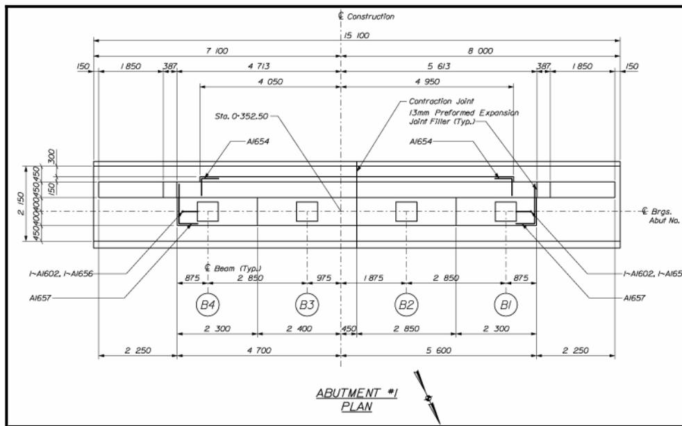
**Figure 3-17 Abutment Plan**
