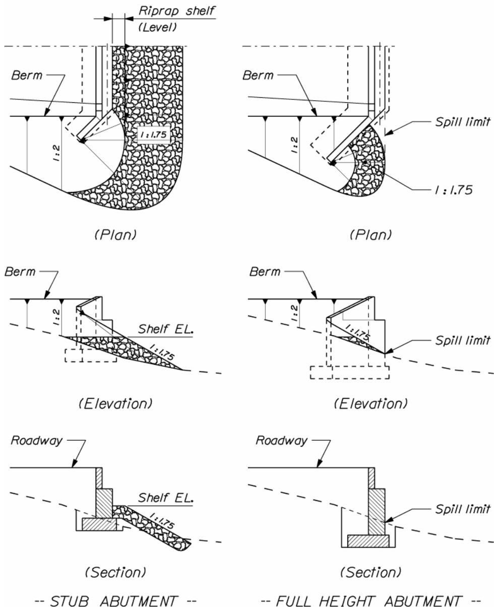
Note: All other conditions being equal, a stub abutment will have shorter wings than a full height abutment
