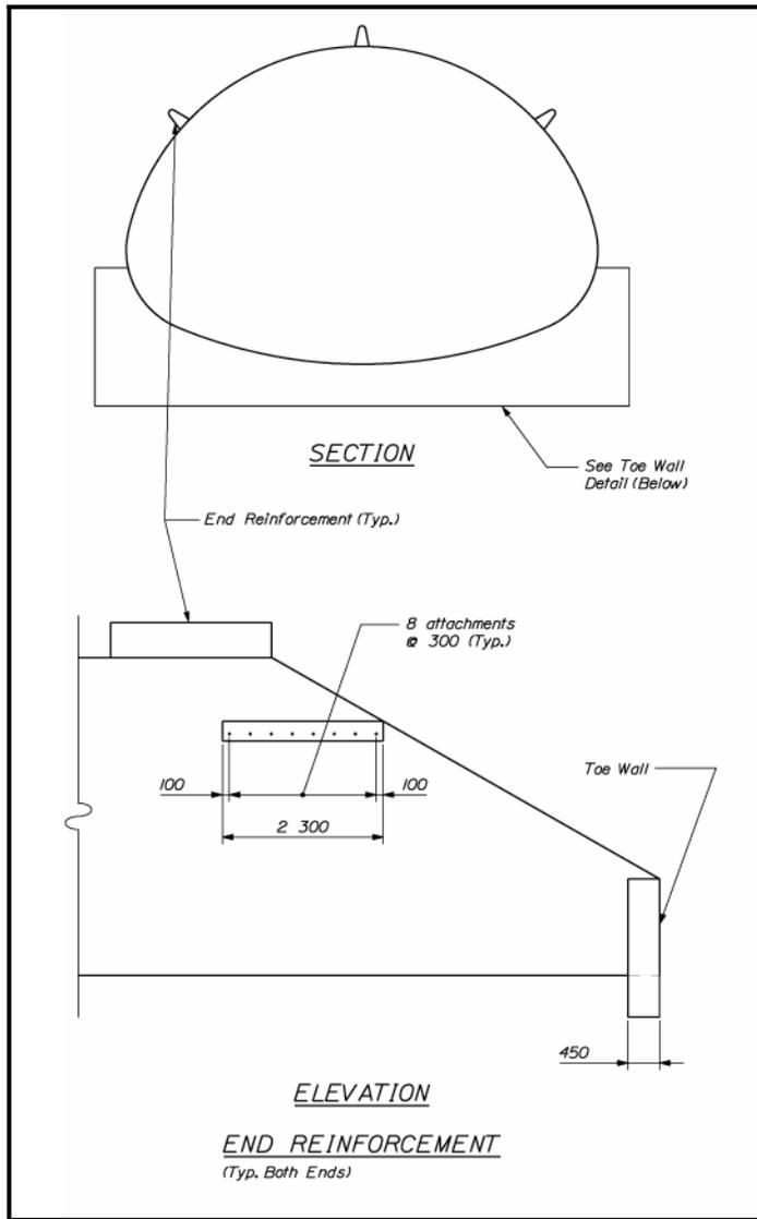
**Figure 5-6 Structural Plate Pipe Arch End Reinforcing**
