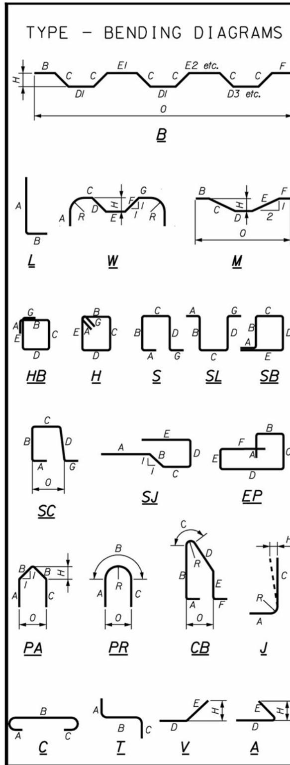
Figure 8-21 Bent Types
