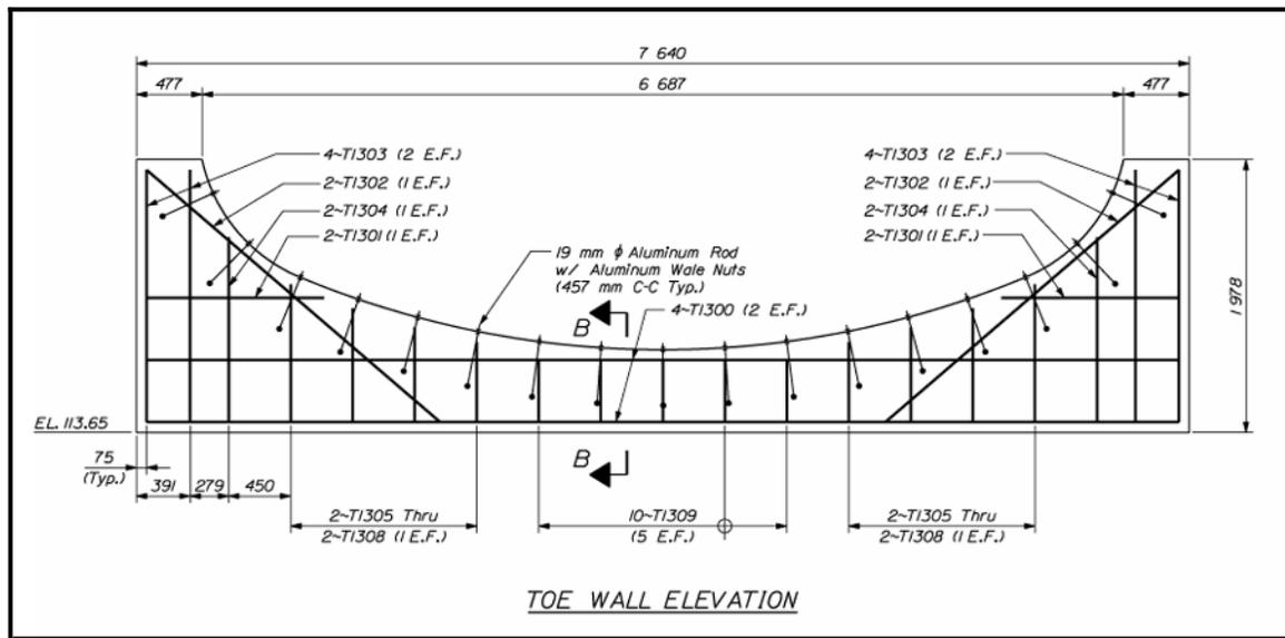
Figure 5-7 Structural Plate Pipe Toe Wall Elevation
