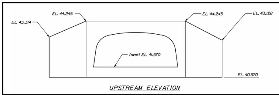
**Figure 5-15 Structural Plate Box Culvert Headwall and Wing Elevation**
