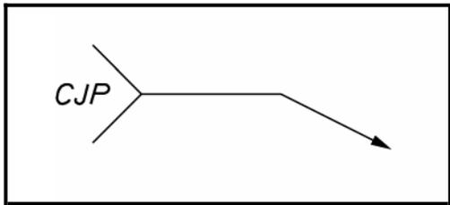
**Figure 9-5 Complete Joint Penetration Callout**
