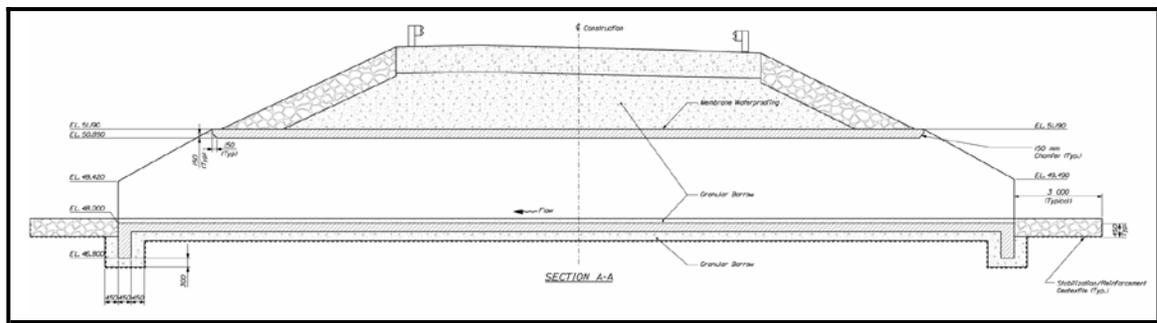
**Figure 5-19 Precast Concrete Box Culvert Longitudinal Section**
