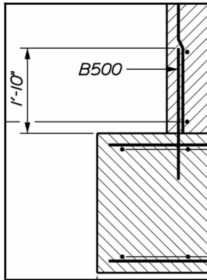
Figure 8-7 Dowel Projection
