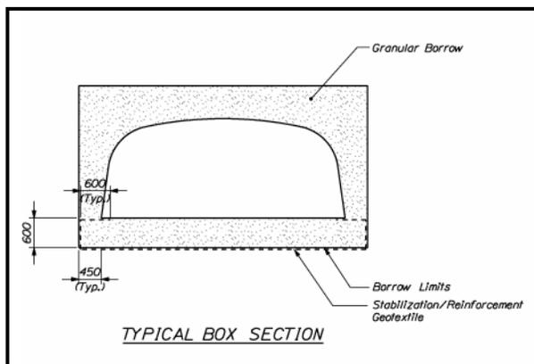
**Figure 5-14 Structural Plate Box Culvert Typical Section**
