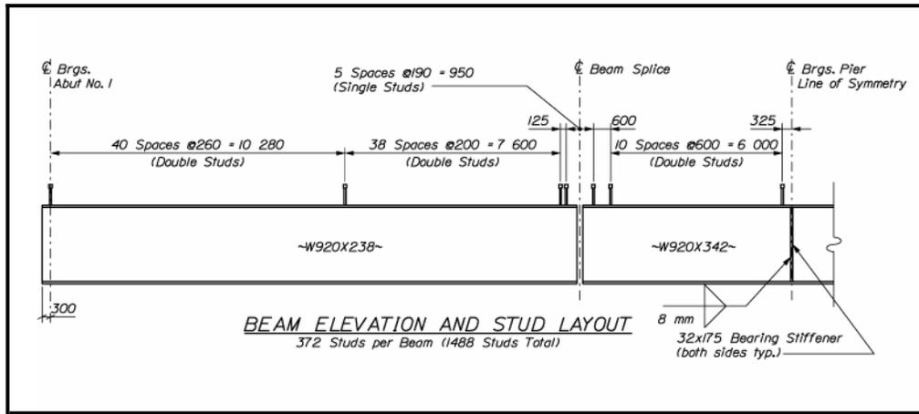
Figure 4-12 Steel Girder Beam Elevation and Stud Layout
