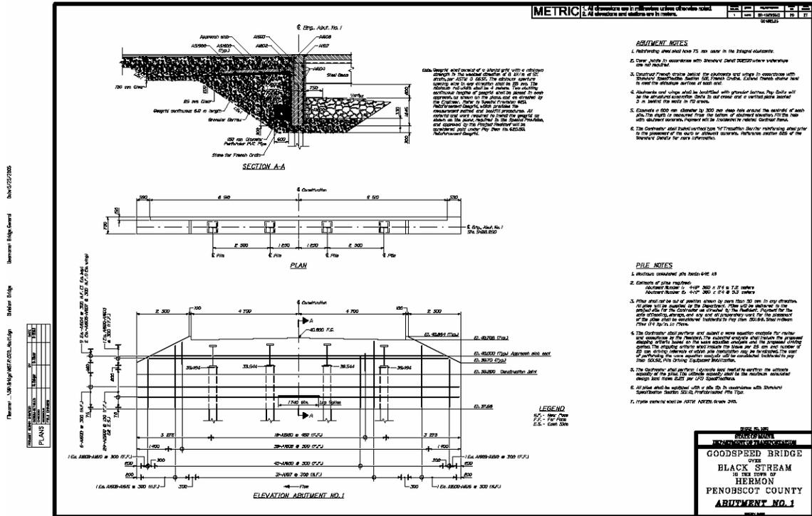
Figure 3-13 Abutment Sheet
