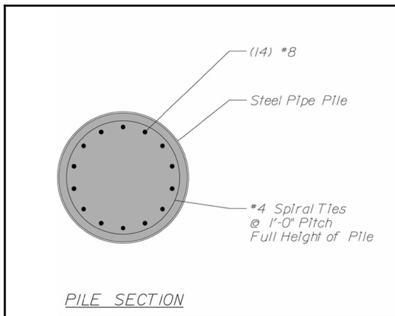
**Figure 3-28 Pile Bent Pier Typical Pile Section****Intro:** Cross section through concrete-filled pipe pile.**Sheet up:** Belongs below pier section or pier elevation**Scale:** 1". Larger scale is acceptable if there is room.**Draw:**
