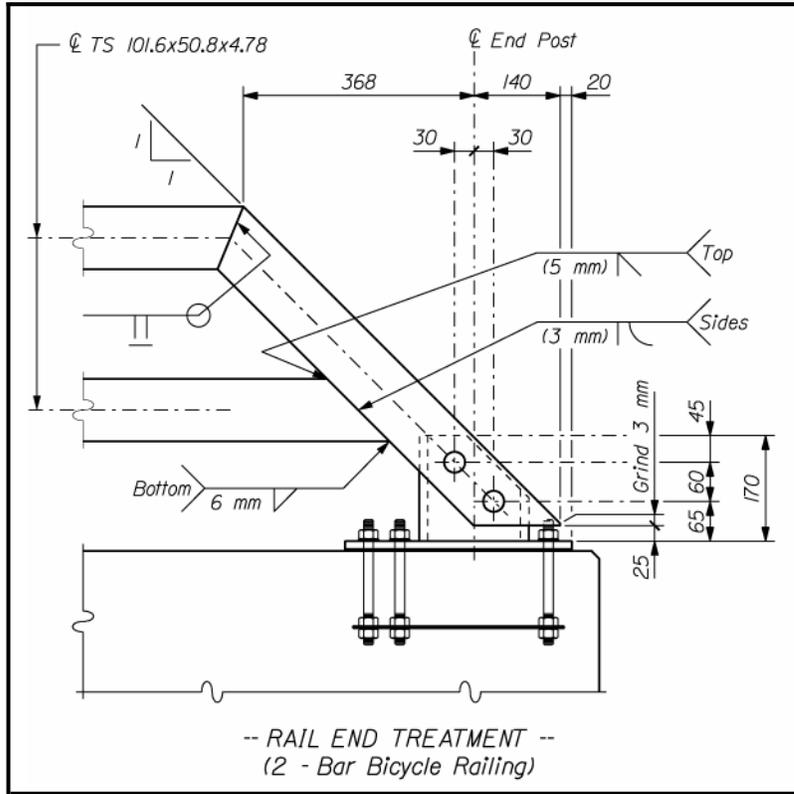
Figure 9-10 Rail End Treatment Weld Example
