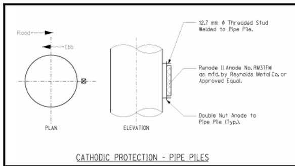
**Figure 3-29 Pile Bent Pier Cathodic Protection – Pipe Piles**
