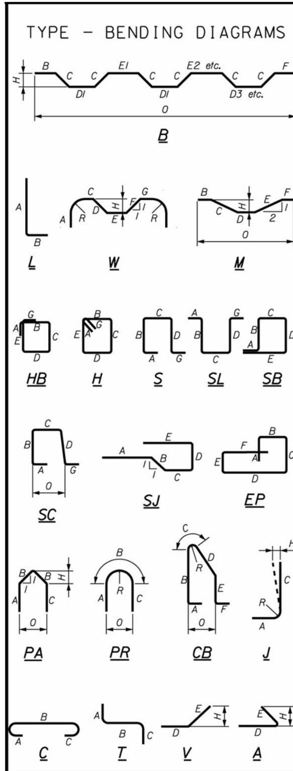
Figure 8-21 Bent Types
