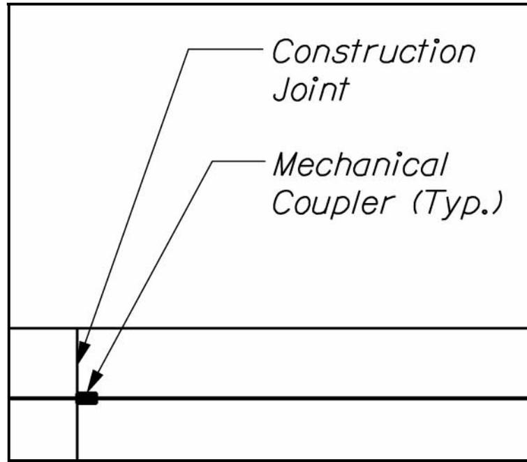
Figure 8-6 Mechanical Coupler
