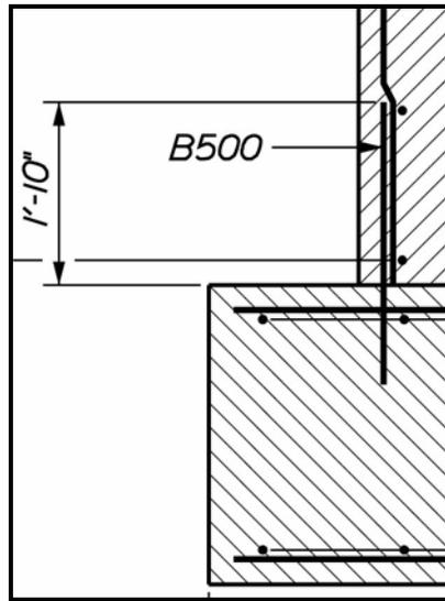
Figure 8-7 Dowel Projection
