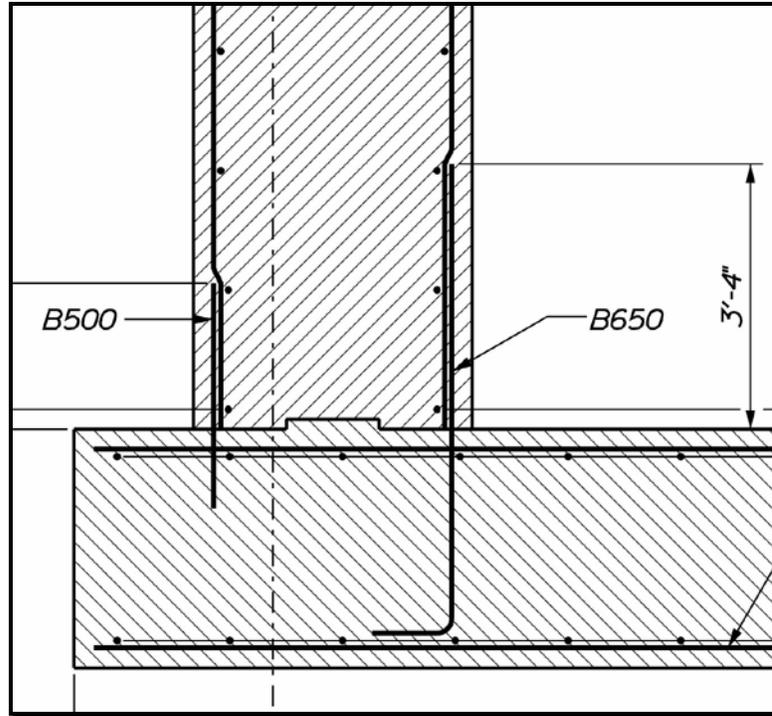
Figure 8-3 Unenclosed Hook
