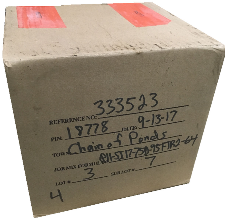
Properly sealed HMA sample.
