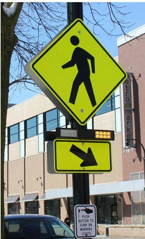
Rectangular Rapid Flashing Beacons (RRFBs) are push-button activated flashing crosswalk signs. They are extremely bright and can be seen for miles. They help convey the message that the area is built up and has pedestrian activity. RRFBs have been shown to have a significant compliance rate (88 % +/-).
