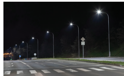
Figure 2-18. Photo. Example of surround light adjacent to a pedestrian crosswalk.
