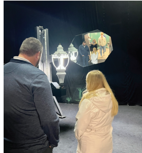
Figure 2-12. Photo. A luminaire being prepared for testing using a goniophotometer. (Photo courtesy of Shayna Bramley)
