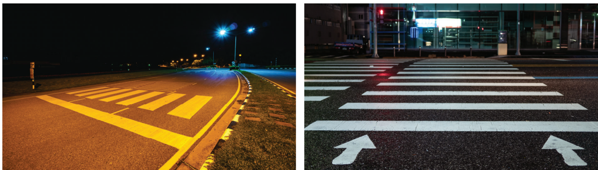
Figure 3-24. Photos. Example of crosswalk with different Kelvin Temperatures. (Left) 2700K HID and (Right) 4000K LEDs.
