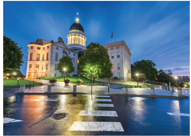
Figure 3-29. Photo. A pedestrian crosswalk near the Maine Capitol building in Augusta. The black and white striping in the crosswalks struggles for contrast due to the reflection of other lighting in the roadway.
