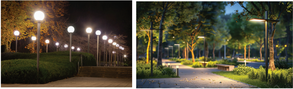
Figure 3-9. Photos. (Left) Example of non-cutoff pedestrian luminaires that cause glare, sky glow, and fail to provide adequate light on their intended target, the ground. (Right) Example of full-cutoff pedestrian luminaires that minimize glare, sky glow, and properly lights the pedestrian path.
