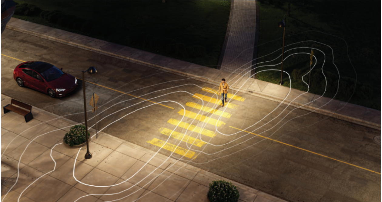
Figure 3-16. Rendering. Example of a mid-block pedestrian crosswalk that is lit by a luminaire with new pedestrian crosswalk optics that have been specifically designed to enhance both the horizontal and vertical illuminance within the crosswalk. The luminaire's iso-footcandle lines are also shown. (Image courtesy of the Cyclone Lighting, Inc, an Acuity Brand.)
