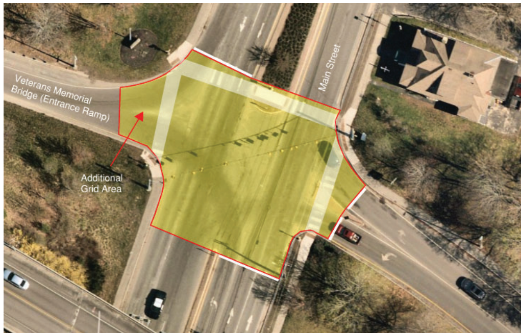
Figure 8-5. Illustration. Intersection of Main Street and Veterans Memorial Bridge Entrance Ramp in Lewiston, Maine. For Full Intersection lighting the horizontal calculation grid include the intersection, crosswalks, and all area up to the stop bars. If there is no stop bar present on an approach leg, engineering judgement shall be used to identify the intersection's boundary and any additional area to ensure the safety of pedestrians.
