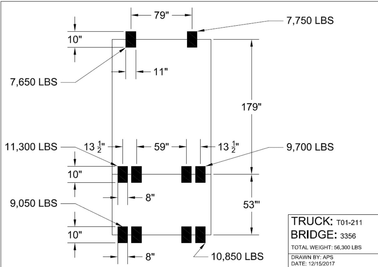
Figure 16: Canton No. 3356 Truck T01-211 loading
