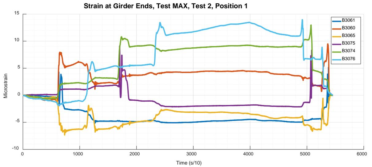
Figure 25: Canton No. 3356- MAX\_1\_2 strains – Ends
