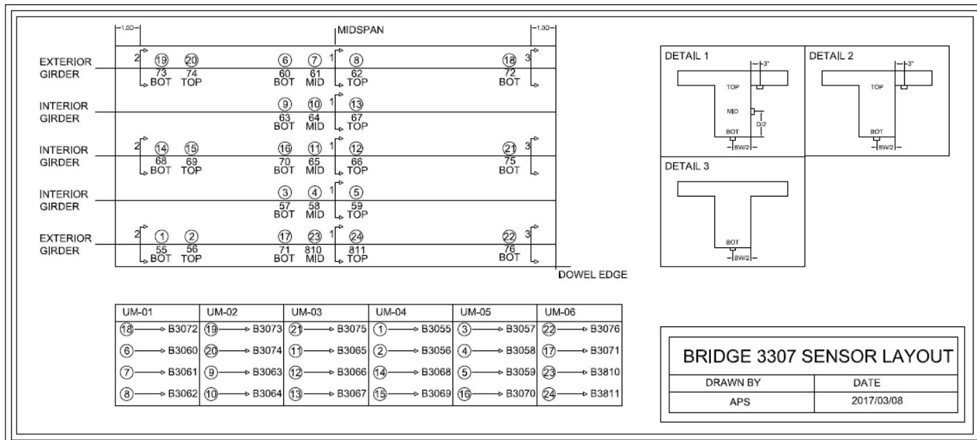
Figure 71: Franklin No. 3307 sensor layout
