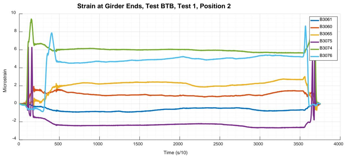
Figure 21: Canton No. 3356- BTB\_2\_1 strains - Ends
