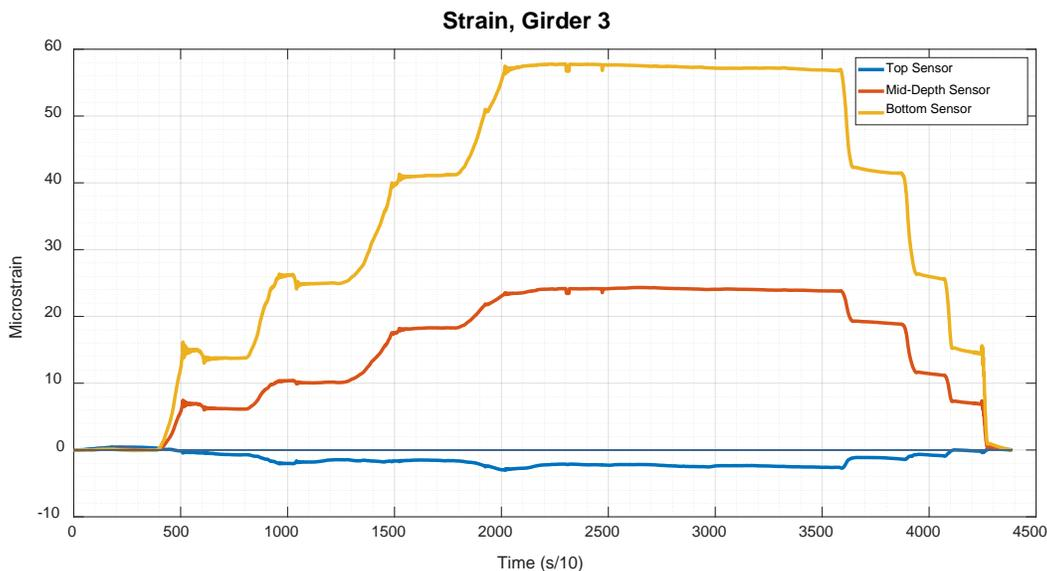
Figure 6: Jackson No. 3776 – MAX\_2\_1, center girder strains at midspan
