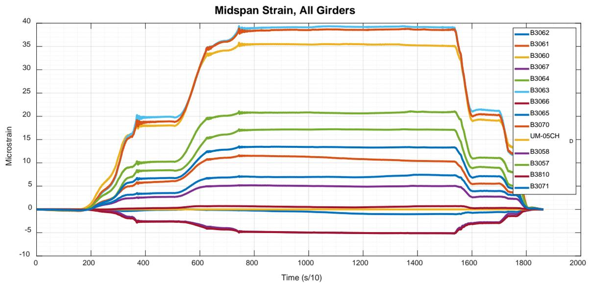
Figure 82: Franklin No. 3307 – BTB\_2\_1 strains - Midspan
