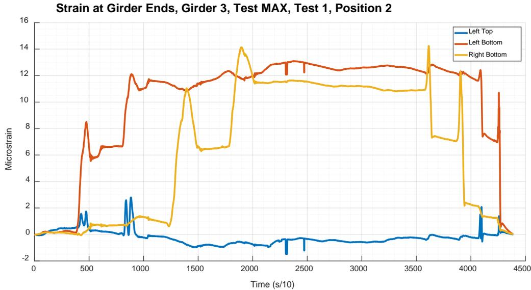
Figure 7: Jackson No. 3776 – MAX\_2\_1, center girder strains at ends
