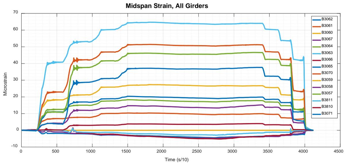
Figure 54: Jackson No. 3776 – ALT\_2\_1 strains - Midspan
