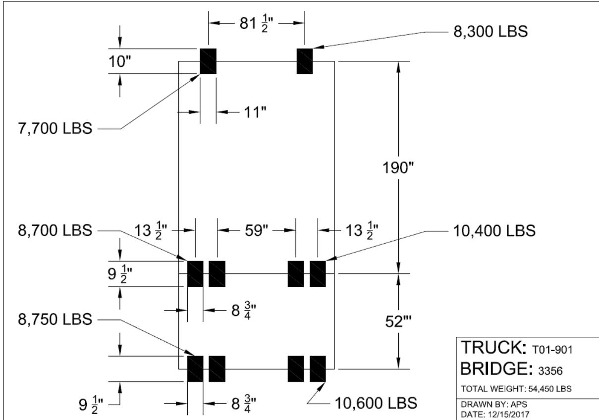
Figure 18: Canton No. 3356 Truck T01-901 loading
