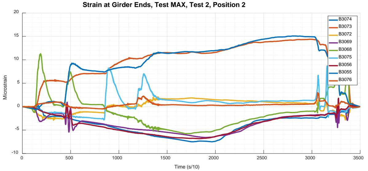
Figure 39: Peru No. 5432 – MAX\_2\_1 - Ends
