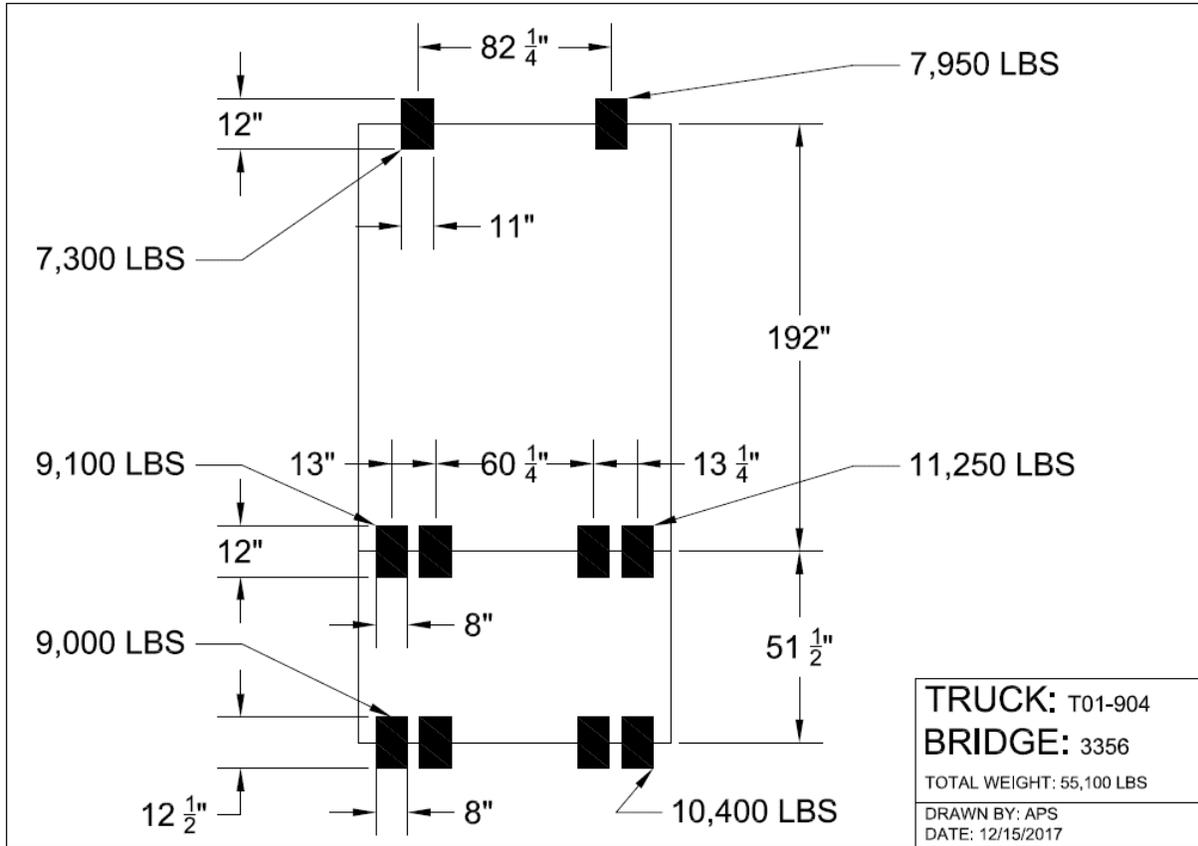
Figure 19: Canton No. 3356 Truck T01-904 loading
