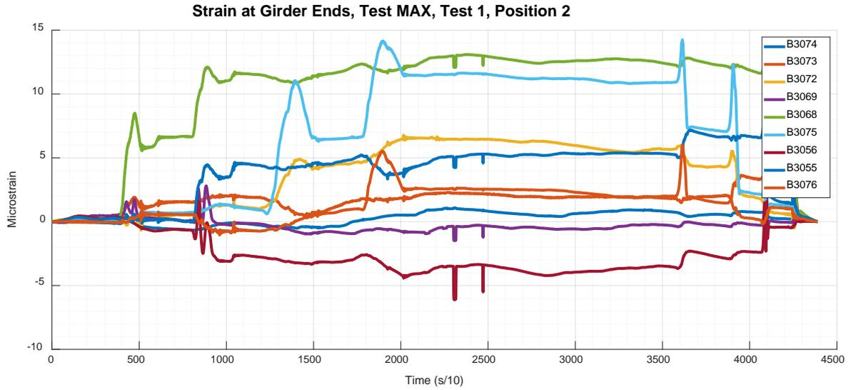
Figure 53: Jackson No. 3776 – MAX\_2\_1 strains - Ends
