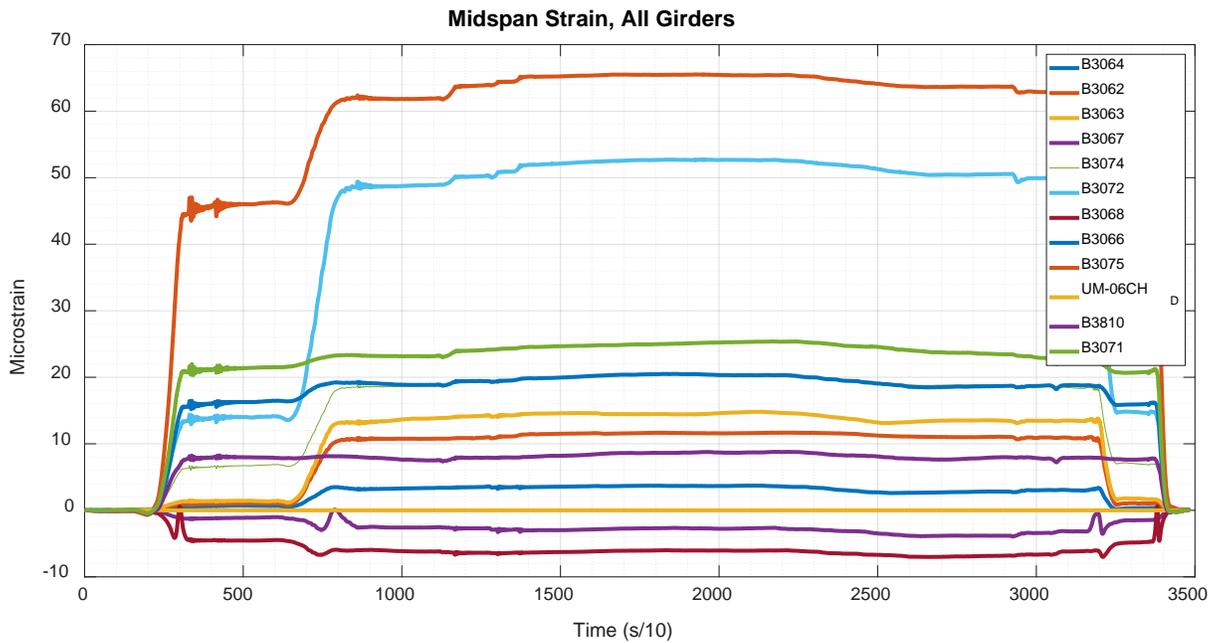
Figure 68: Alna No. 2130 – ALT\_2\_1 strains - Midspan
