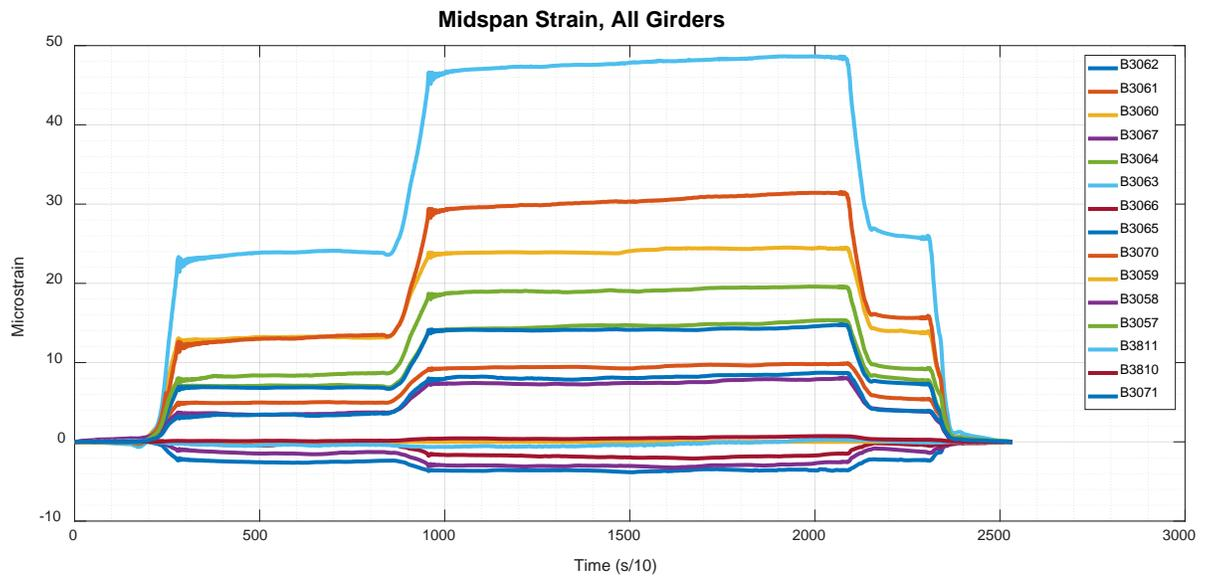
Figure 48: Jackson No. 3776 – BTB\_2\_1 strains - Midspan
