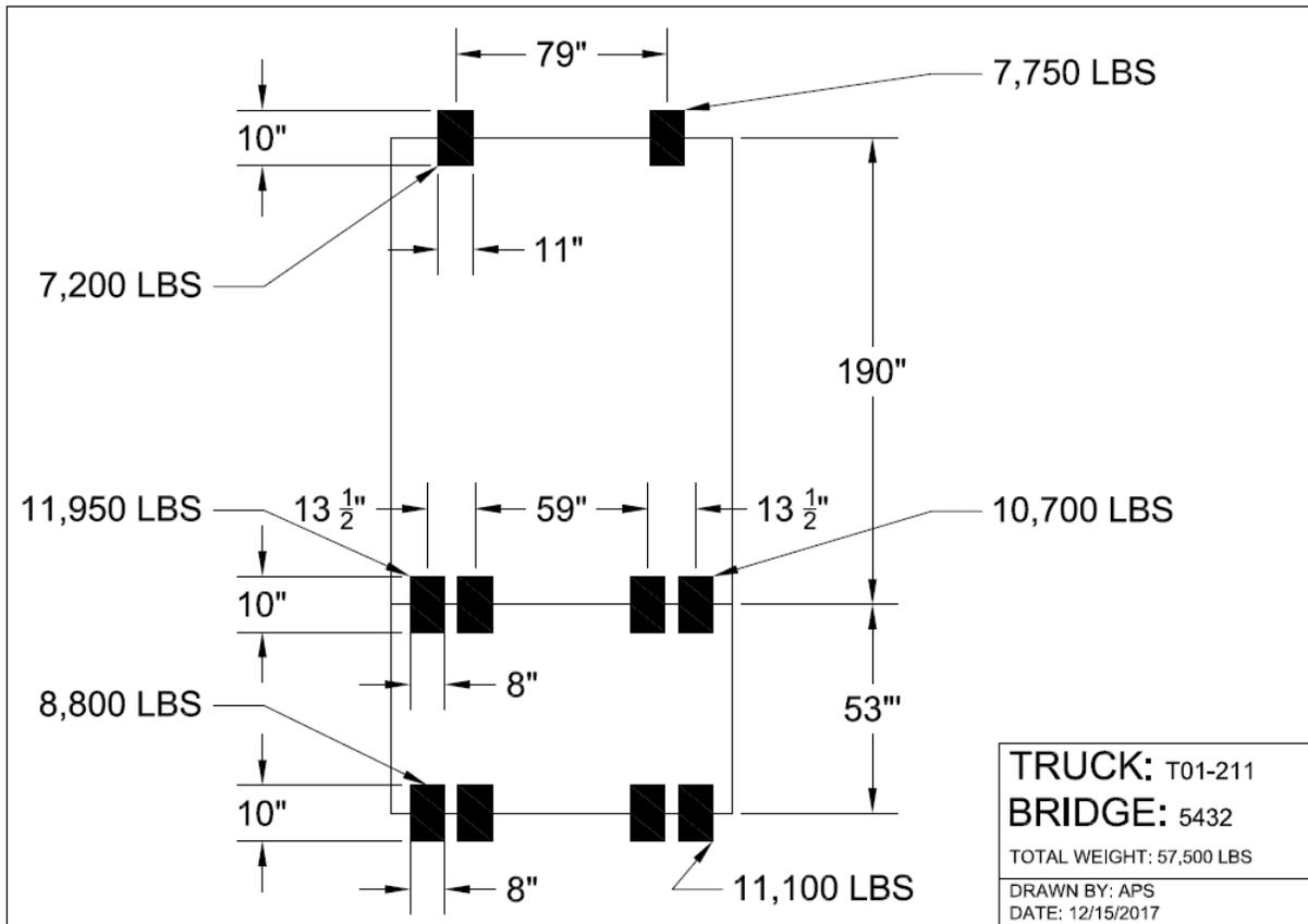
Figure 30: Peru No. 5432 Truck T01-211 loading
