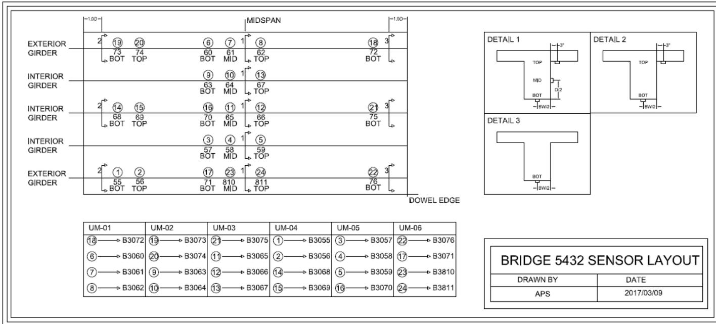
Figure 29: Peru No. 5432 sensor layout
