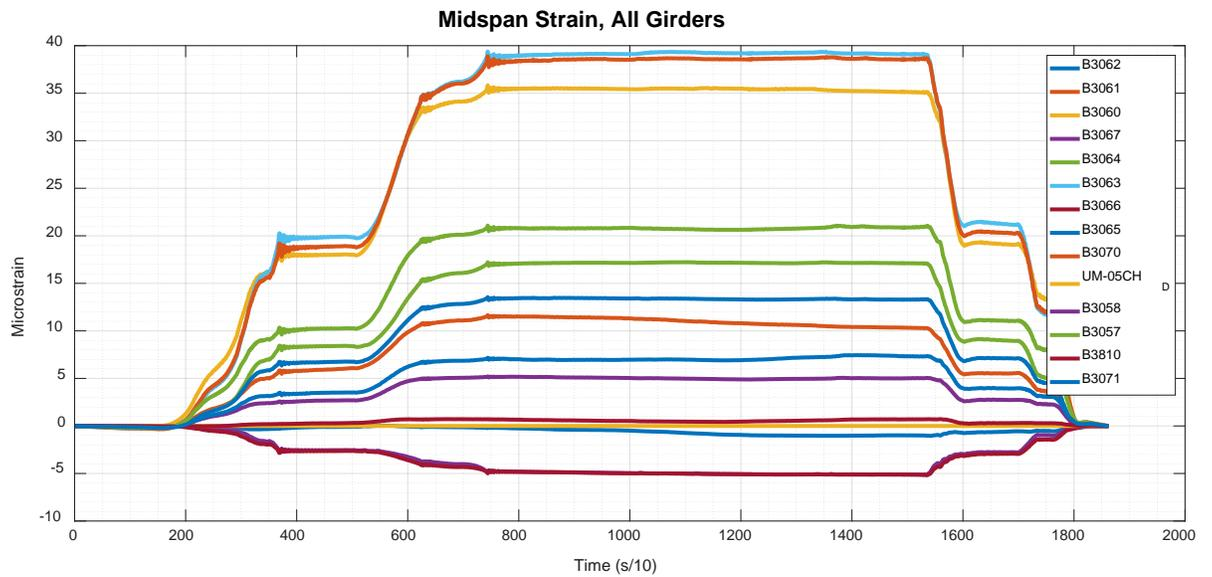
Figure 76: Franklin No. 3307 – BTB\_2\_1 strains - Midspan
