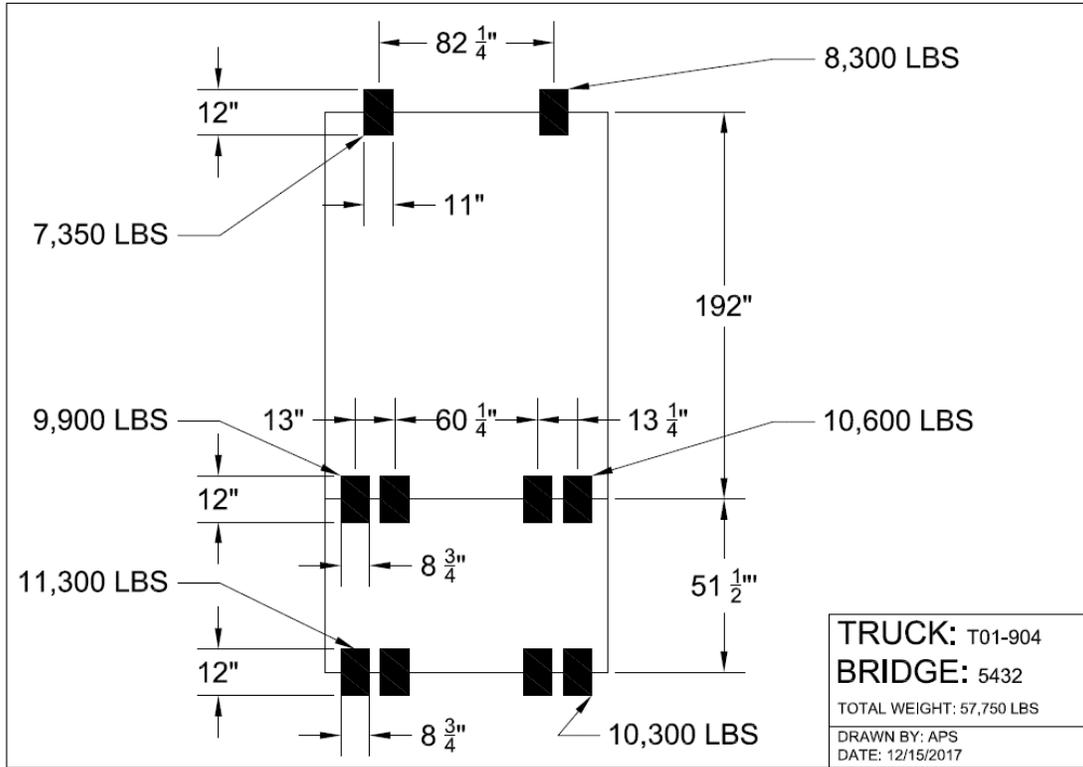
Figure 33: Peru No. 5432 Truck T01-904 loading
