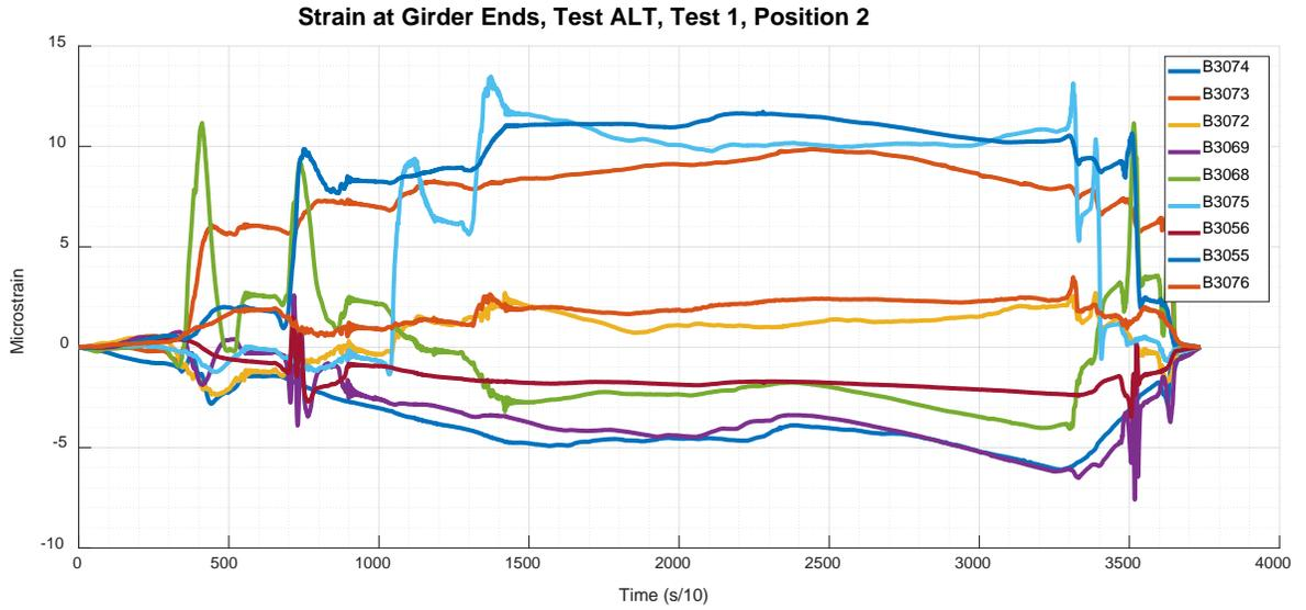
Figure 41: Peru No. 5432 – ALT\_2\_1 - Ends
