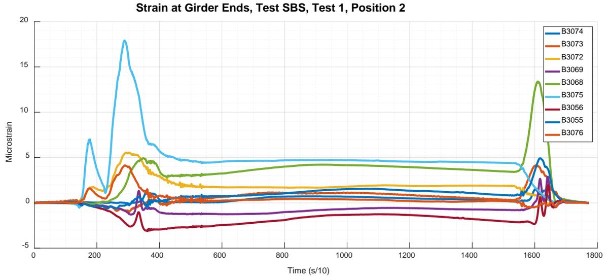
Figure 51: Jackson No. 3776 – SBS\_2\_1 strains – Ends
