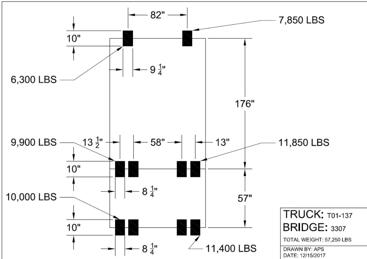
Figure 72: Franklin No. 3307 Truck T01-137 loading
