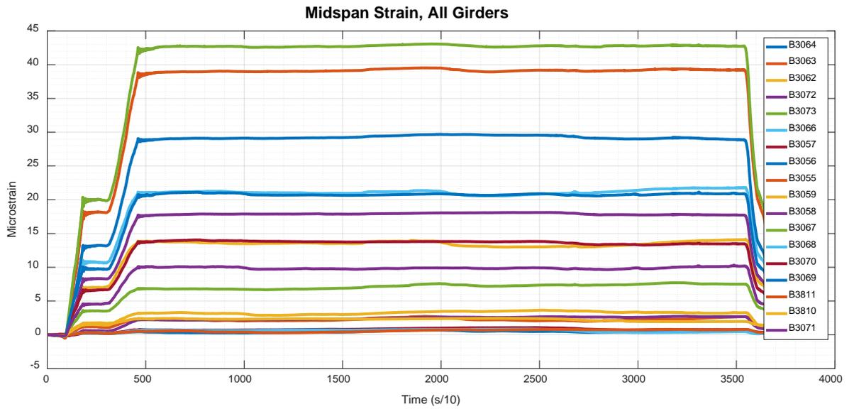
Figure 20: Canton No. 3356- BTB\_2\_1 strains - Midspan
