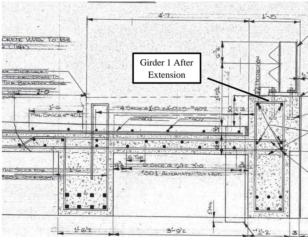
Figure 10: Canton No. 3356 redesigned cross section
