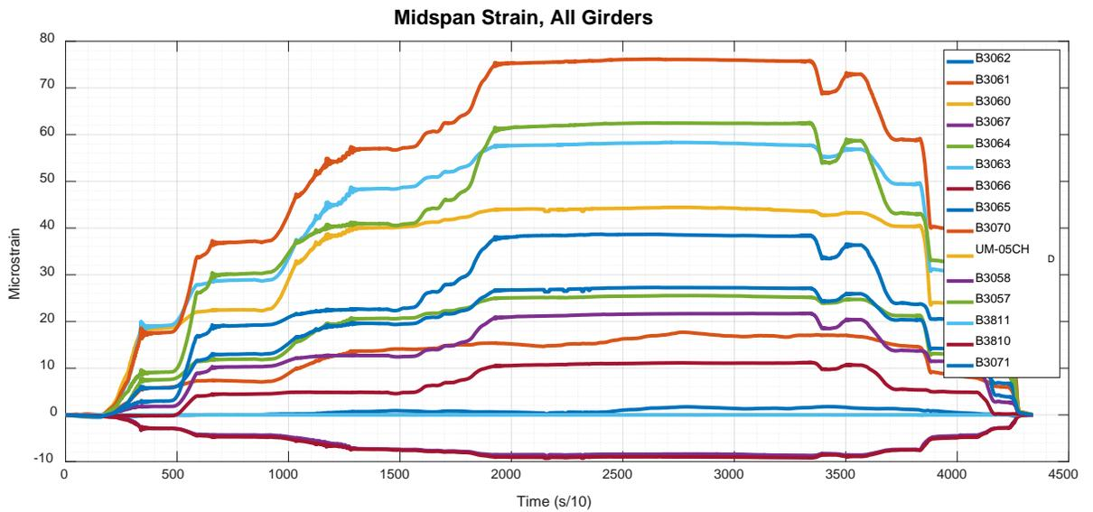
Figure 80: Franklin No. 3307 – MAX\_2\_1 strains - Midspan
