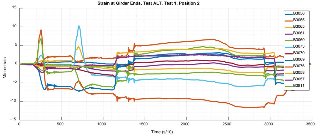
Figure 69: Alna No. 2130 – ALT\_2\_1 strains - Ends
