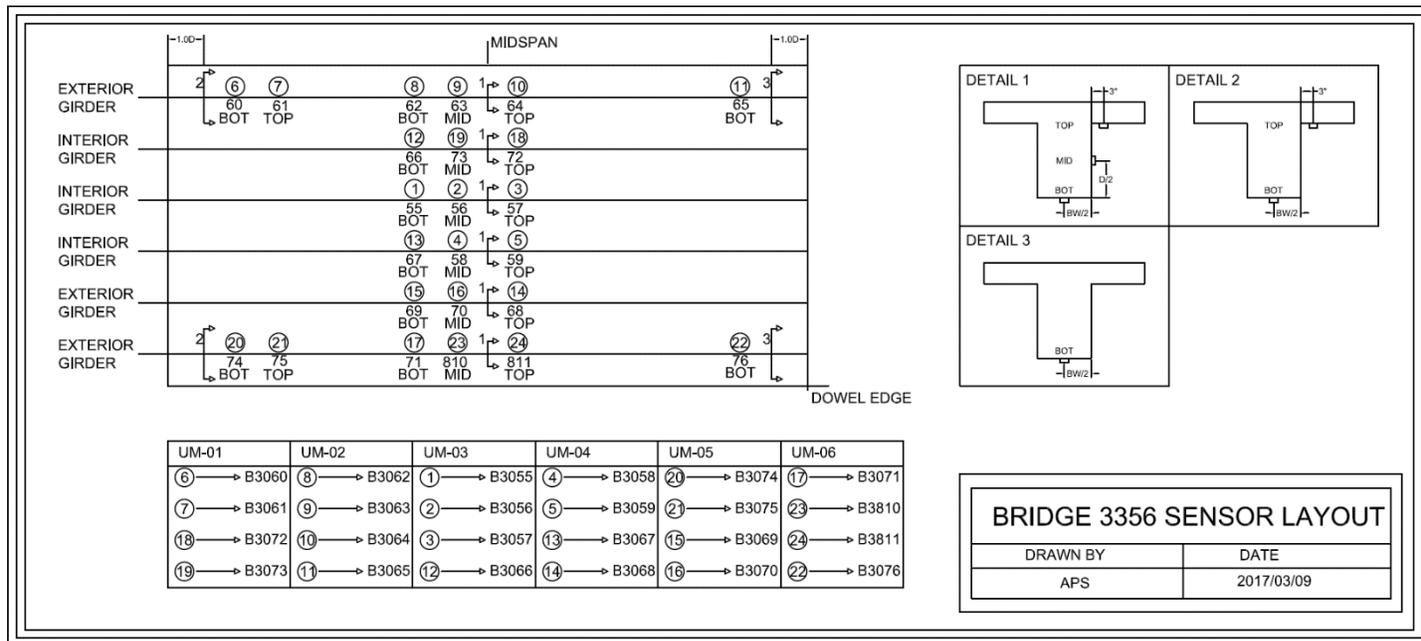
Figure 15: Canton No. 3356 sensor layout
