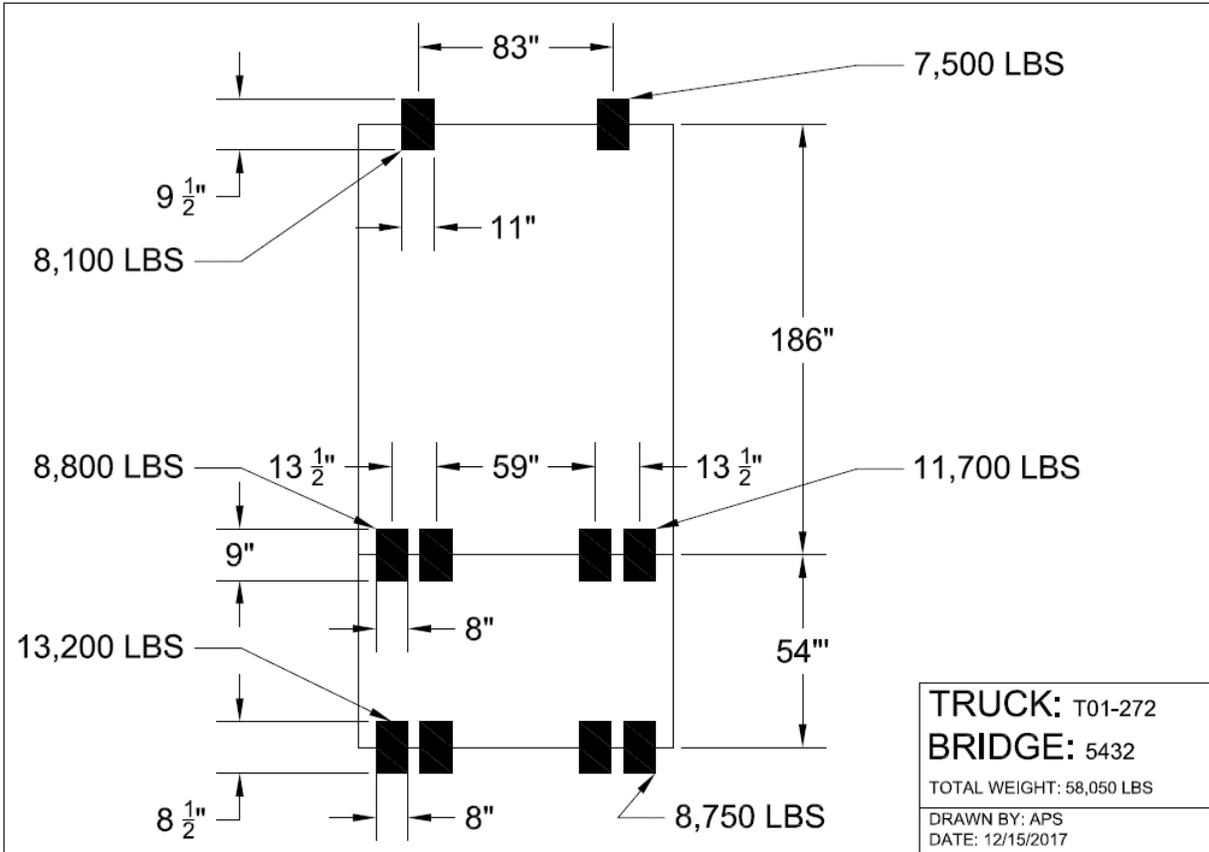
Figure 31: Peru No. 5432 Truck T01-272 loading
