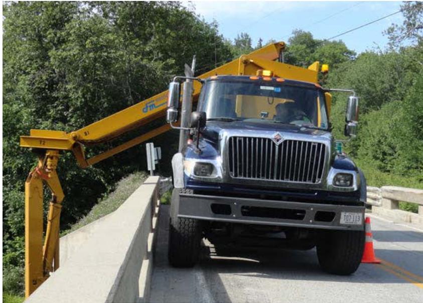
Figure 3: MaineDOT UBIT used to install sensors
