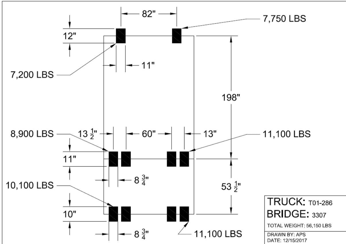
Figure 75: Franklin No. 3307 Truck T01-286 loading
