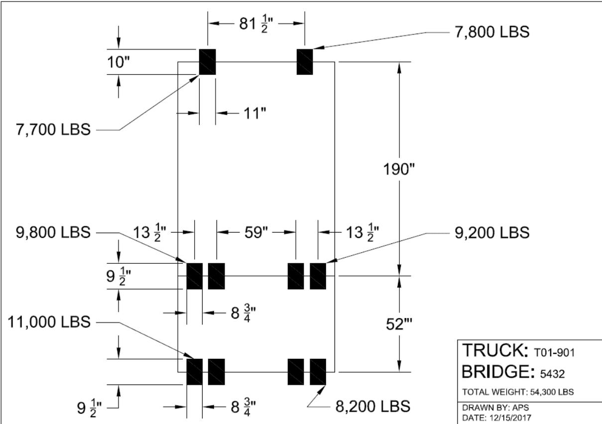
Figure 32: Peru No. 5432 Truck T01-901 loading
