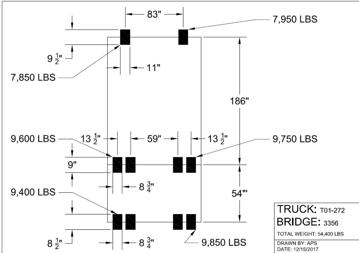
Figure 17: Canton No. 3356 Truck T01-272 loading
