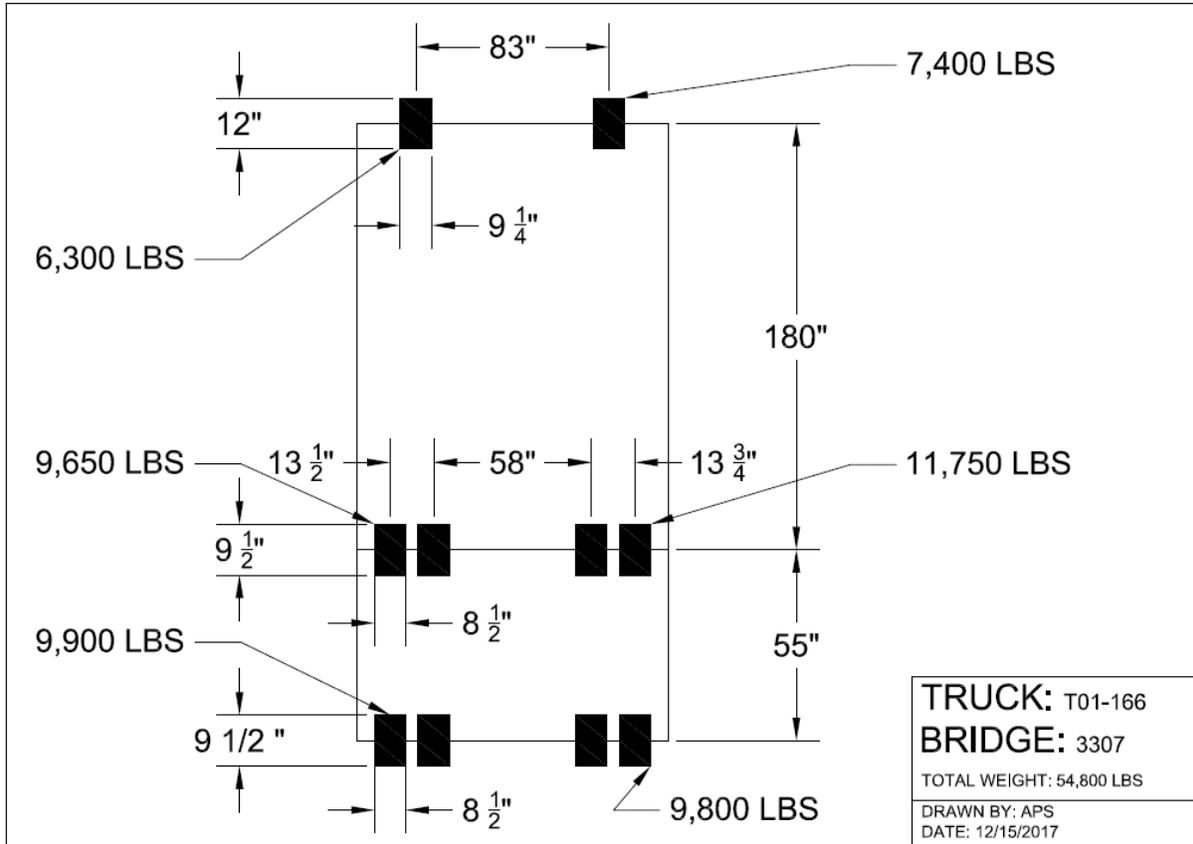
Figure 73: Franklin No. 3307 Truck T01-166 loading
