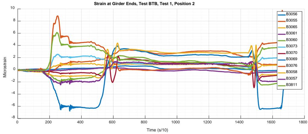
Figure 83: Franklin No. 3307 – BTB\_2\_1 strains - Ends
