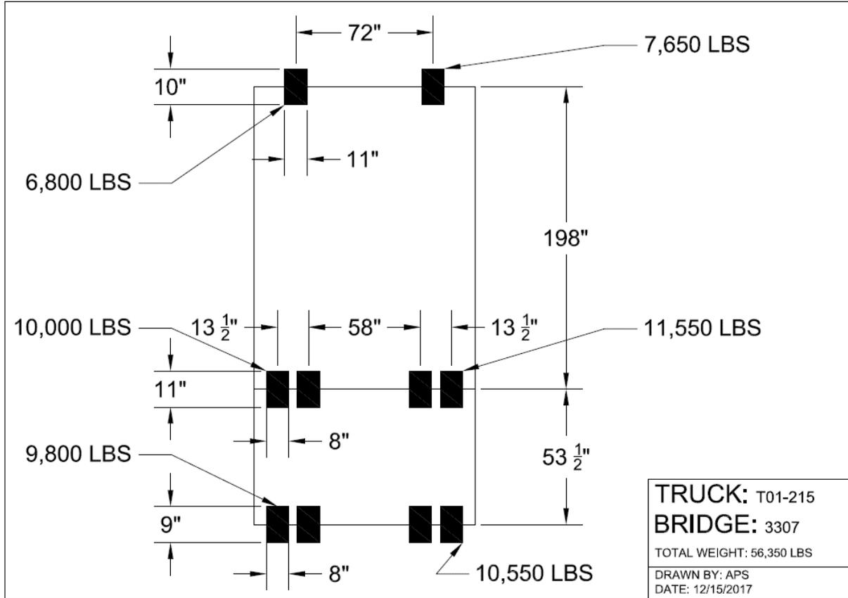
Figure 74: Franklin No. 3307 Truck T01-215 loading
