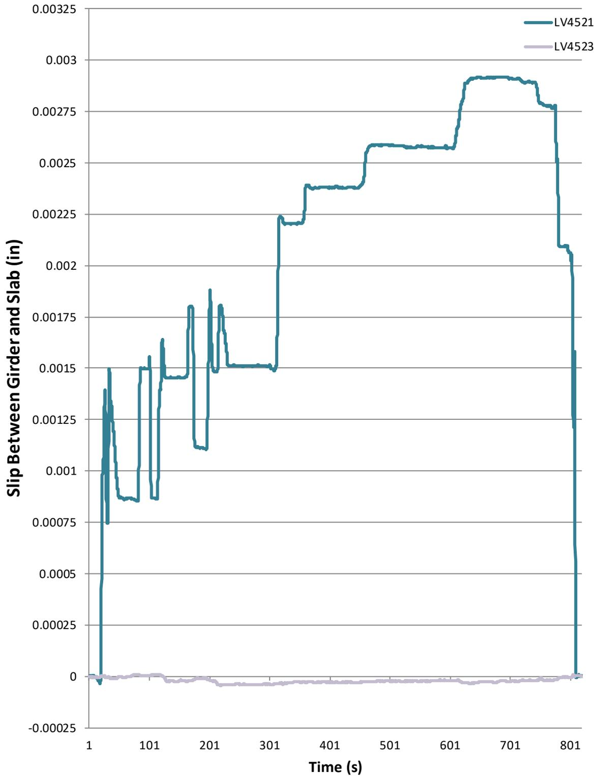
Figure 26: Steuben No. 3067- 4 trucks 2 lanes test 2 shear slip
