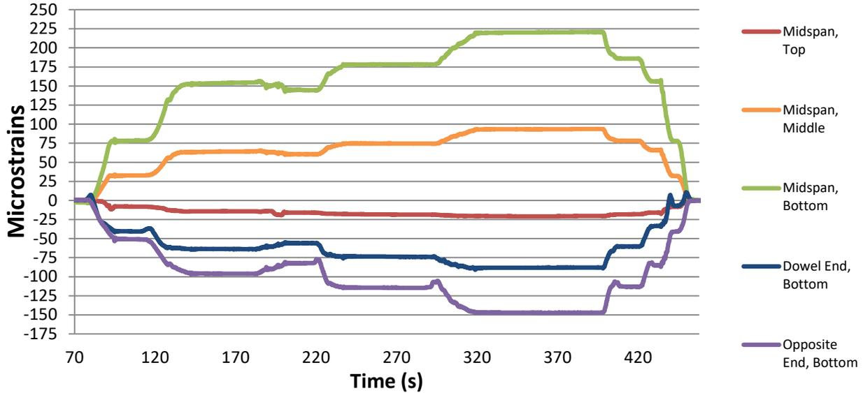
Figure 6: Pembroke No. 3884 – 4 trucks, 2 lanes, test 2, strains in center girder
