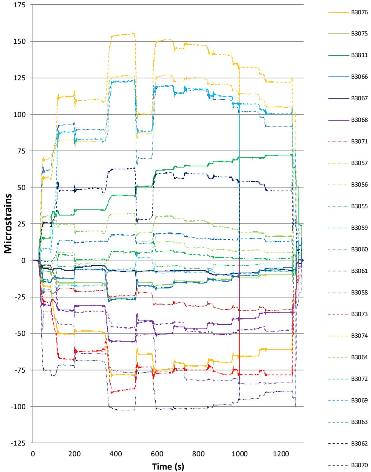
Figure 55: Windham No. 5298 - 4 trucks 2 lanes test 2 strains
