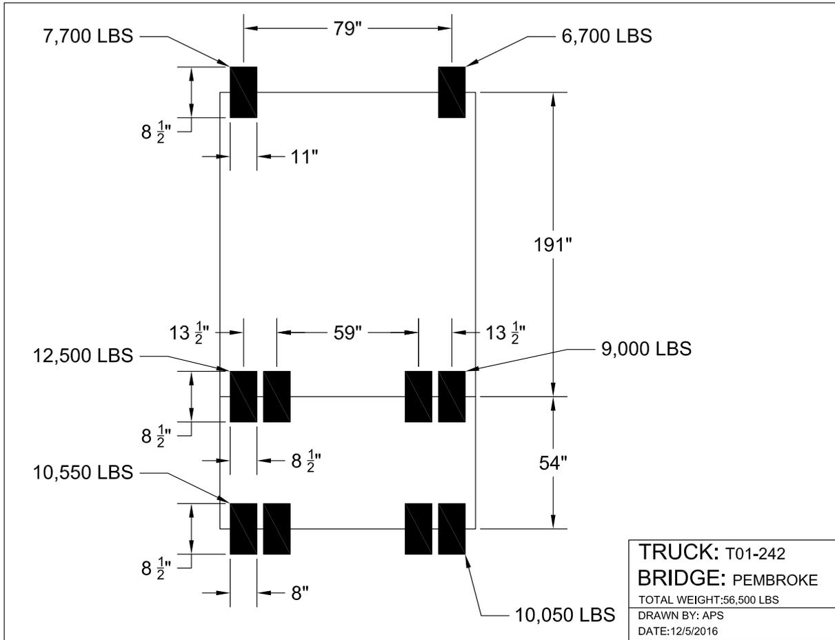
Figure 41: Pembroke No. 3884 Truck T01-242 loading
