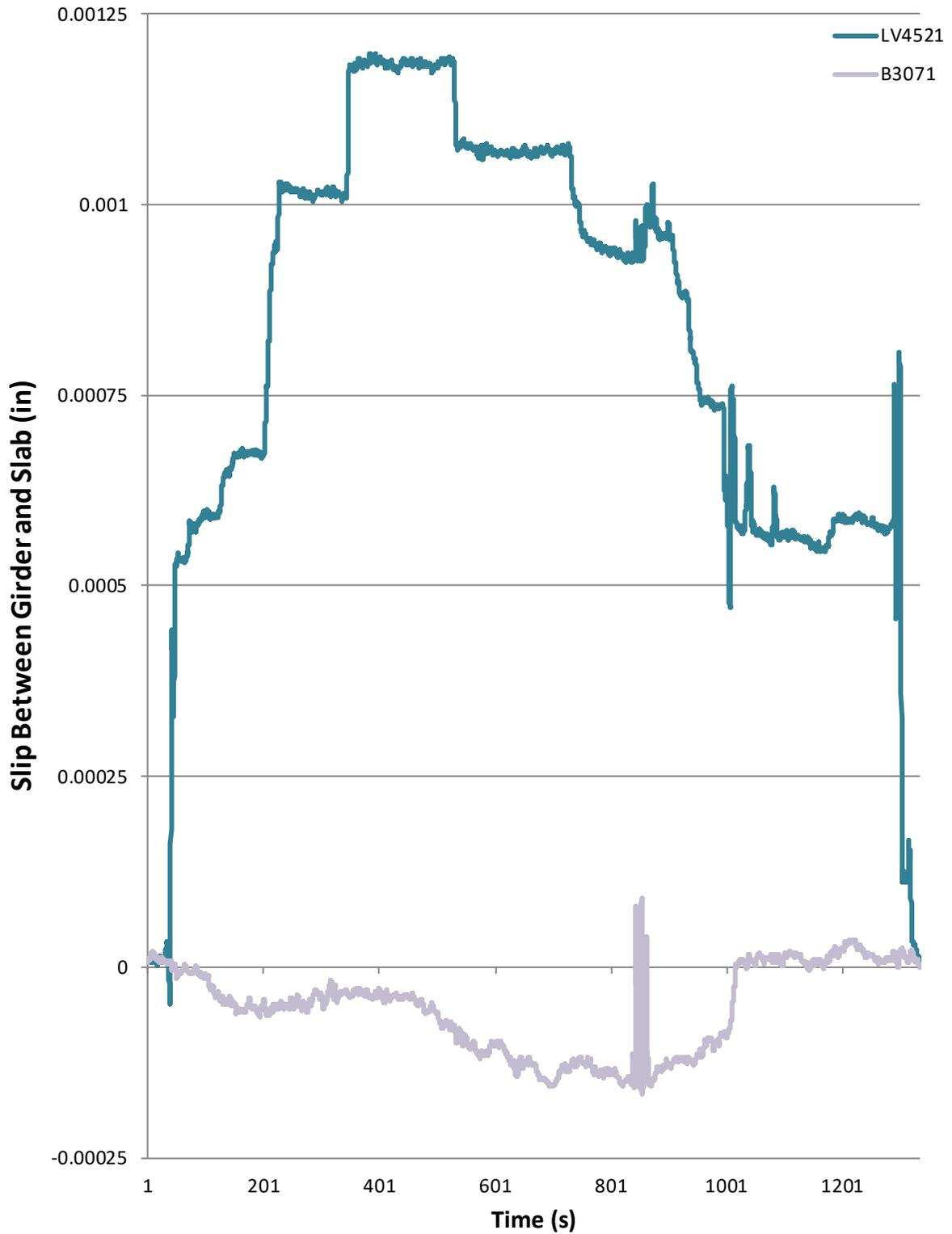
Figure 36: Waltham No. 3238 - 4 trucks 2 lanes test 1 shear slip
