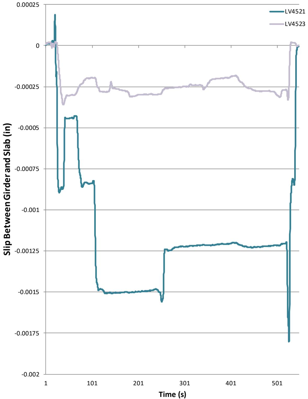
Figure 44: Pembroke No. 3884 - 4 trucks 2 lanes test 1 shear slip
