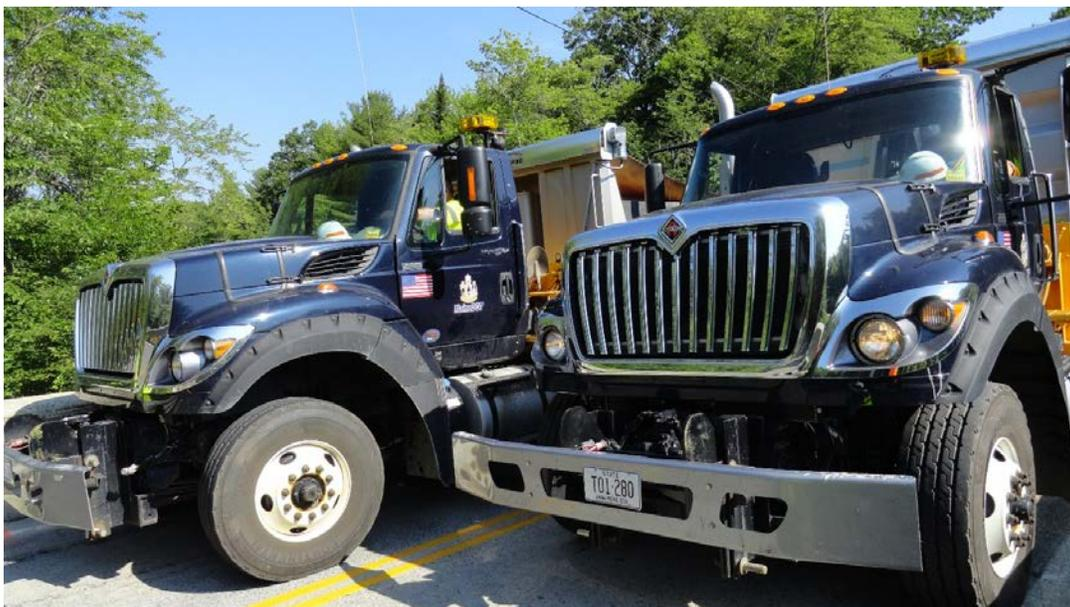
Figure 4: Maine DOT trucks used for bridge loading
