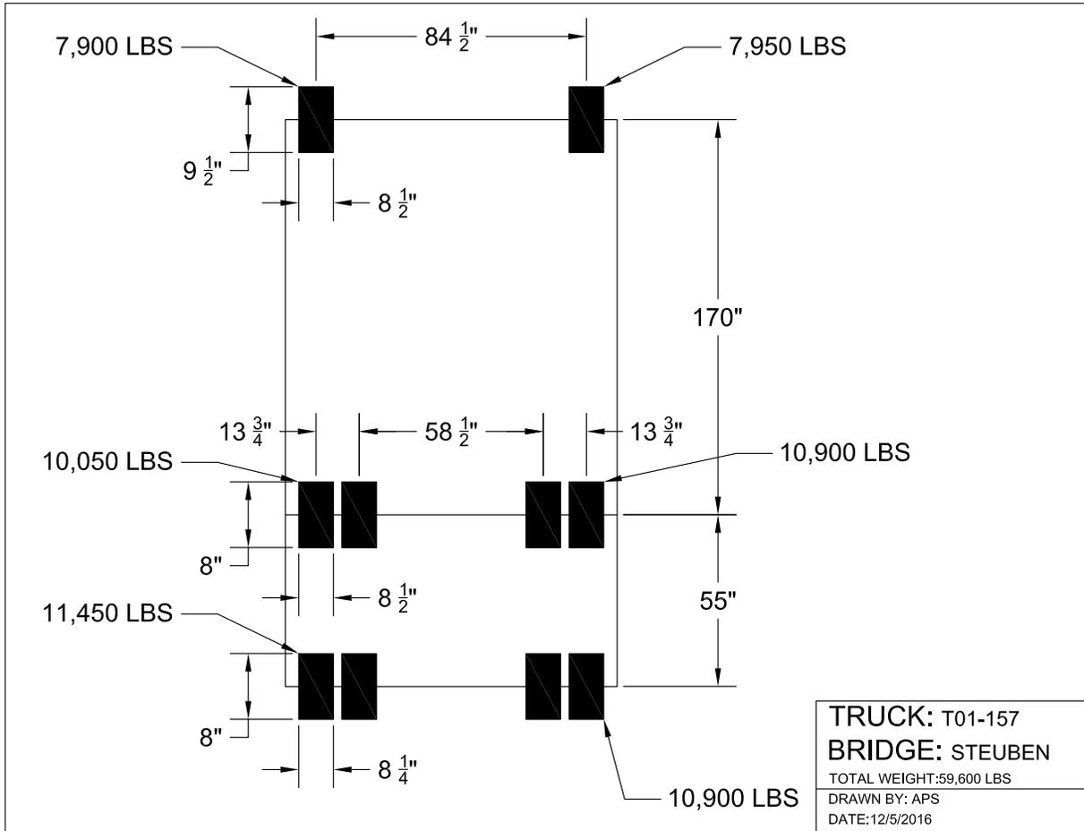
Figure 18: Steuben No. 3067 Truck T01-157 loading
