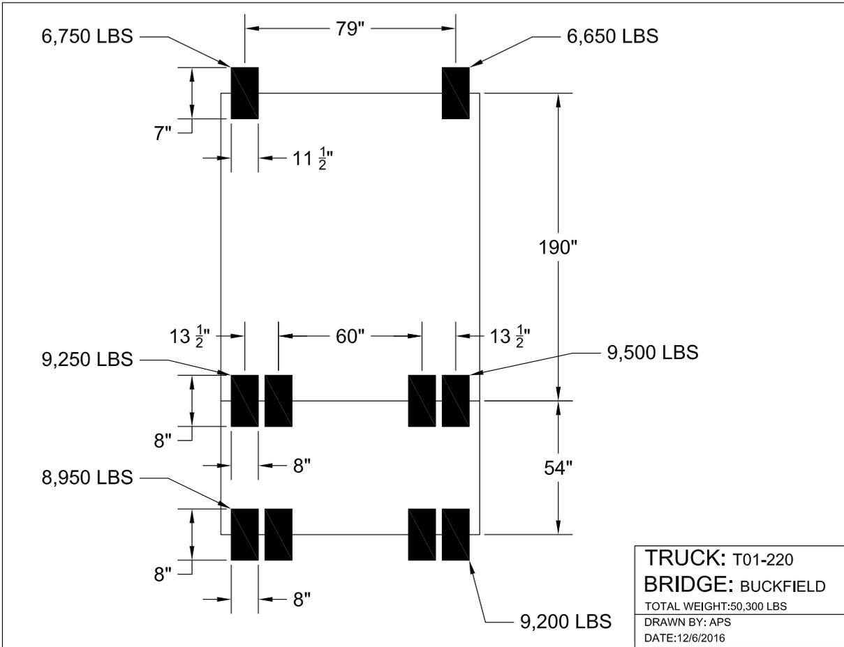
Figure 60: Buckfield No. 5452 Truck T01-220 loading
