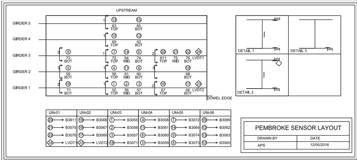
Figure 38: Pembroke No. 3884 sensor layout
