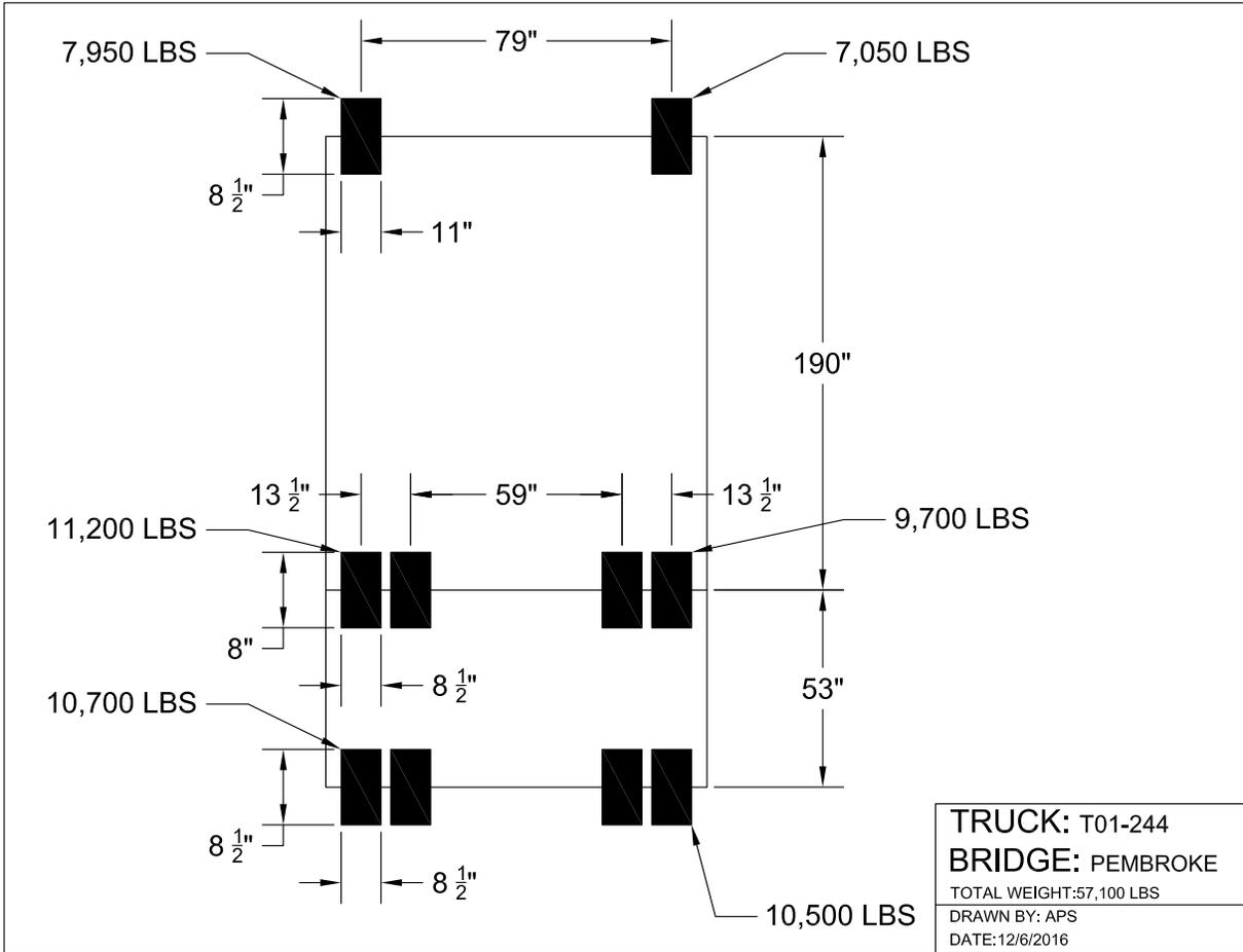
Figure 42: Pembroke No. 3884 Truck T01-244 loading
