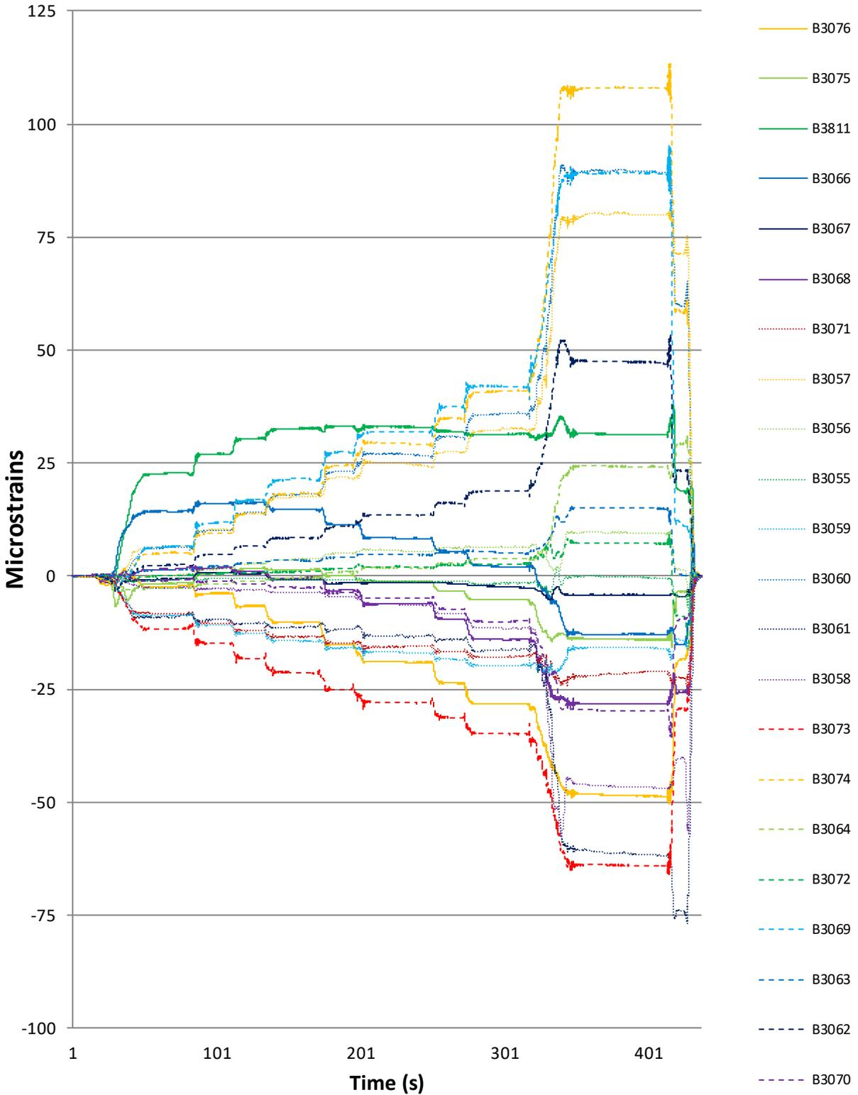
Figure 53: Windham No. 5298 - 2 trucks 2 lanes test 1 strains
