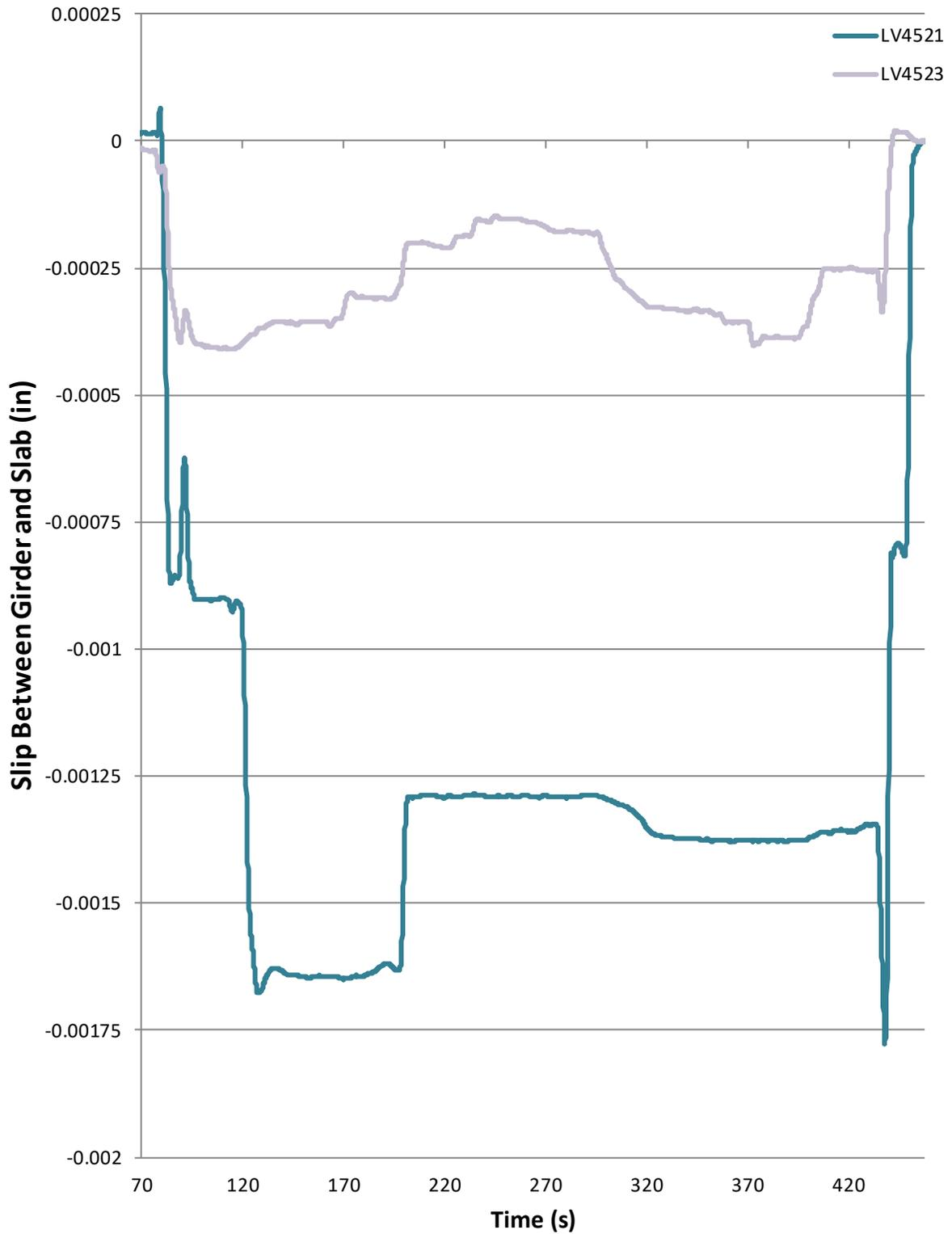
Figure 46: Pembroke No. 3884 - 4 trucks 2 lanes test 2 shear slip
