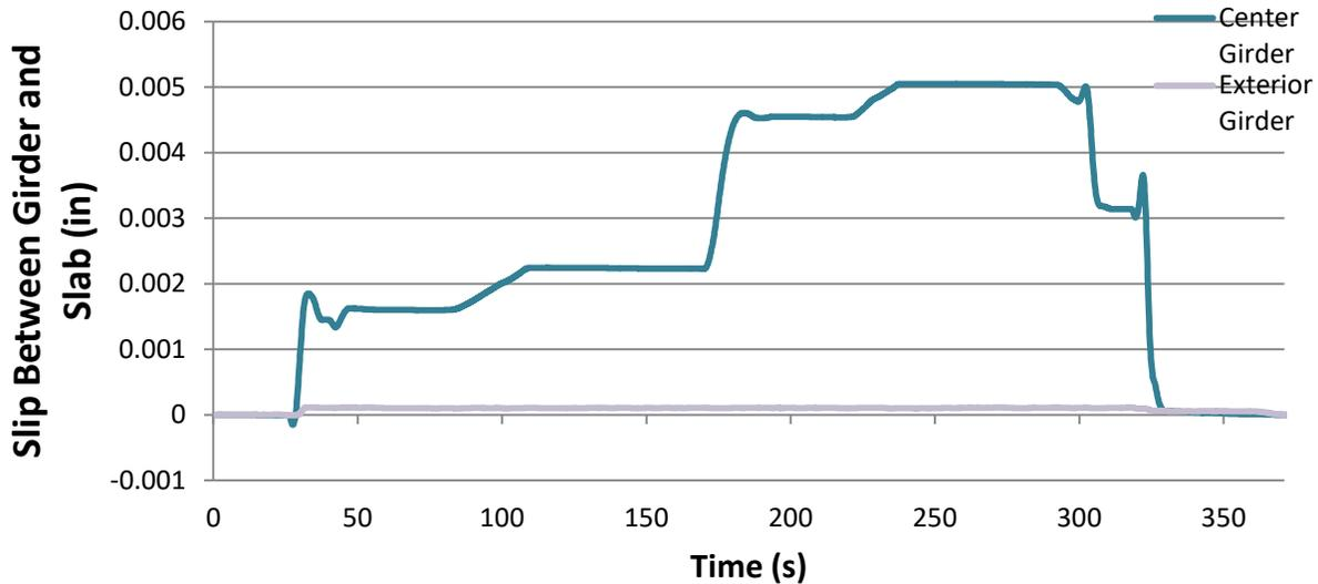
Figure 9: Buckfield No. 5452 - 4 trucks, 2 lanes, test 1, slip between girder and slab
