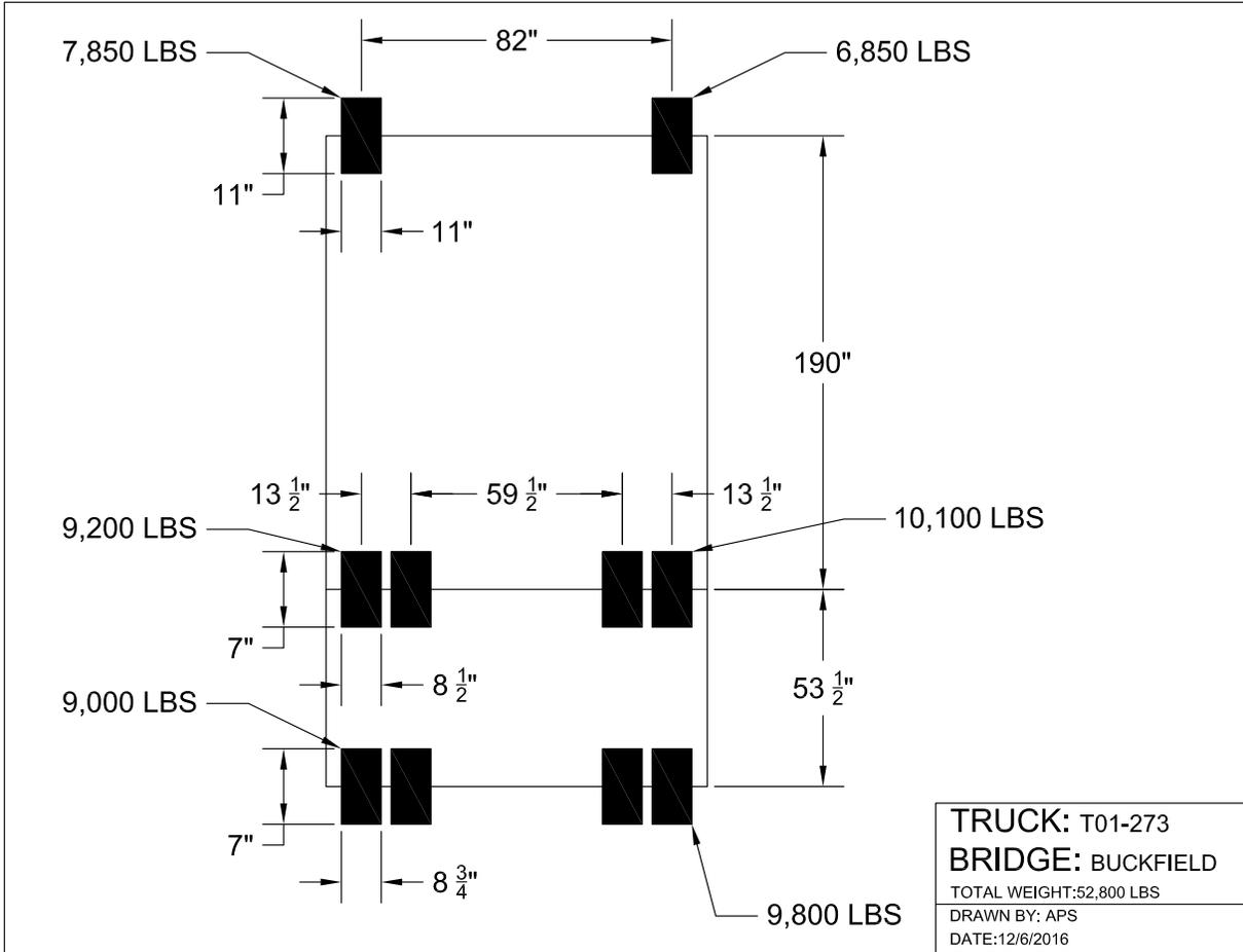
Figure 62: Buckfield No. 5452 Truck T01-273 loading
