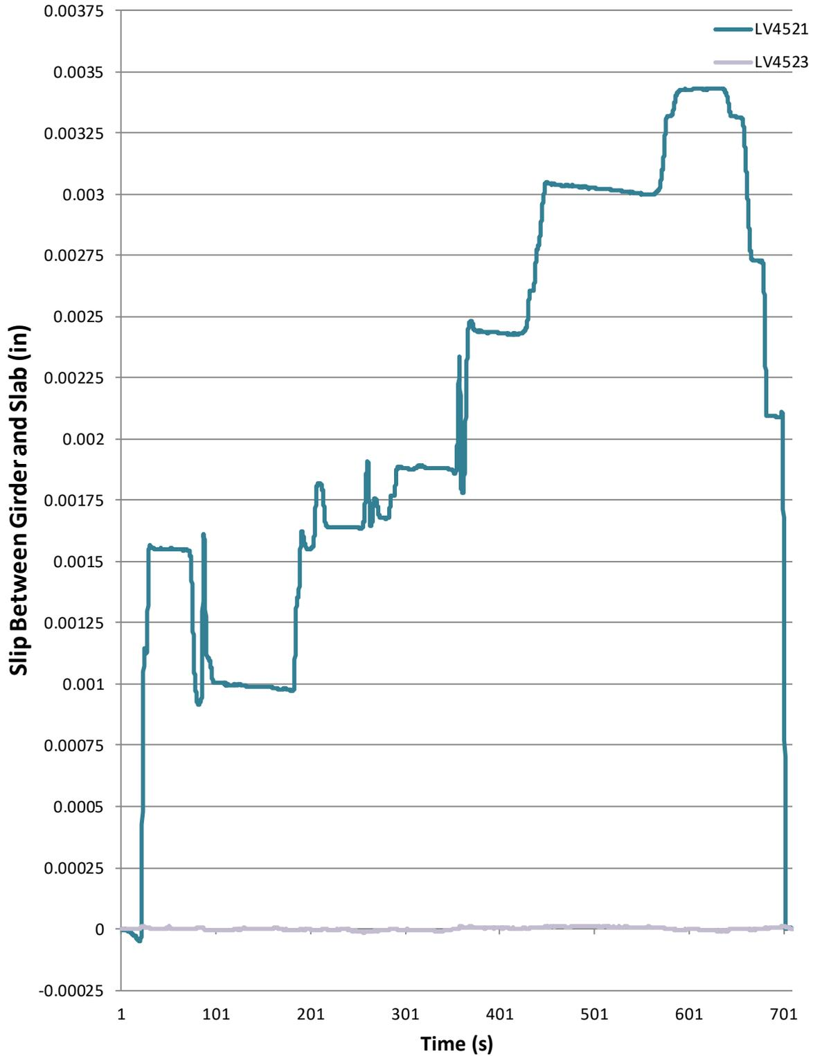
Figure 24: Steuben No. 3067- 4 trucks 2 lanes test 1 shear slip
