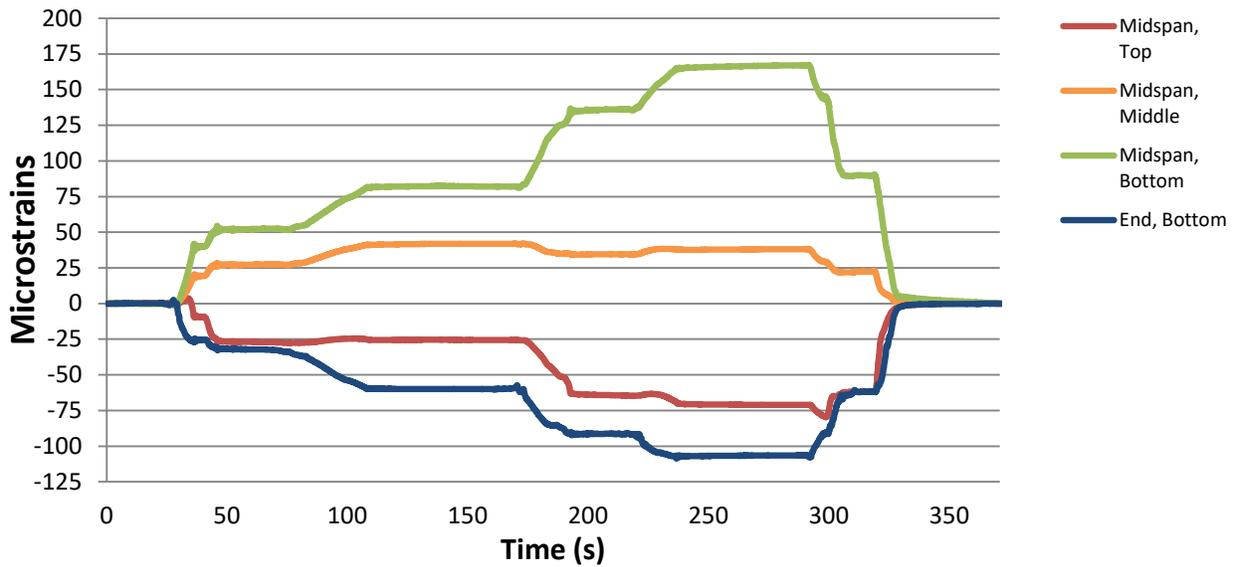
Figure 8: Buckfield No. 5452 - 4 trucks, 2 lanes, test 1, strain in center girder
