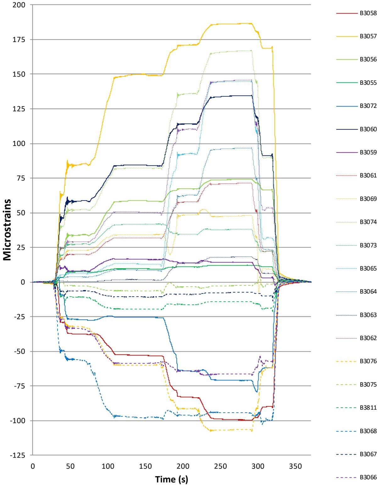
Figure 63: Buckfield No. 5425 - 4 trucks 2 lanes test 1 strains
