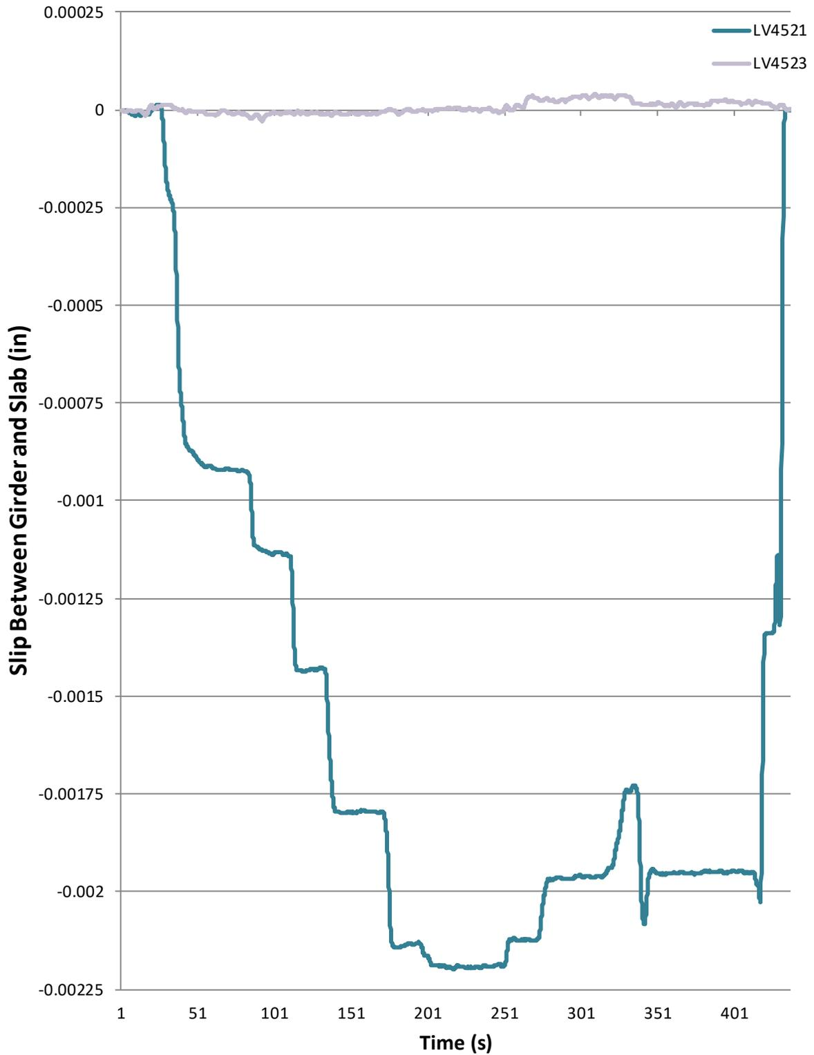
Figure 54: Windham No. 5298 - 2 trucks 2 lanes test 1 shear slip
