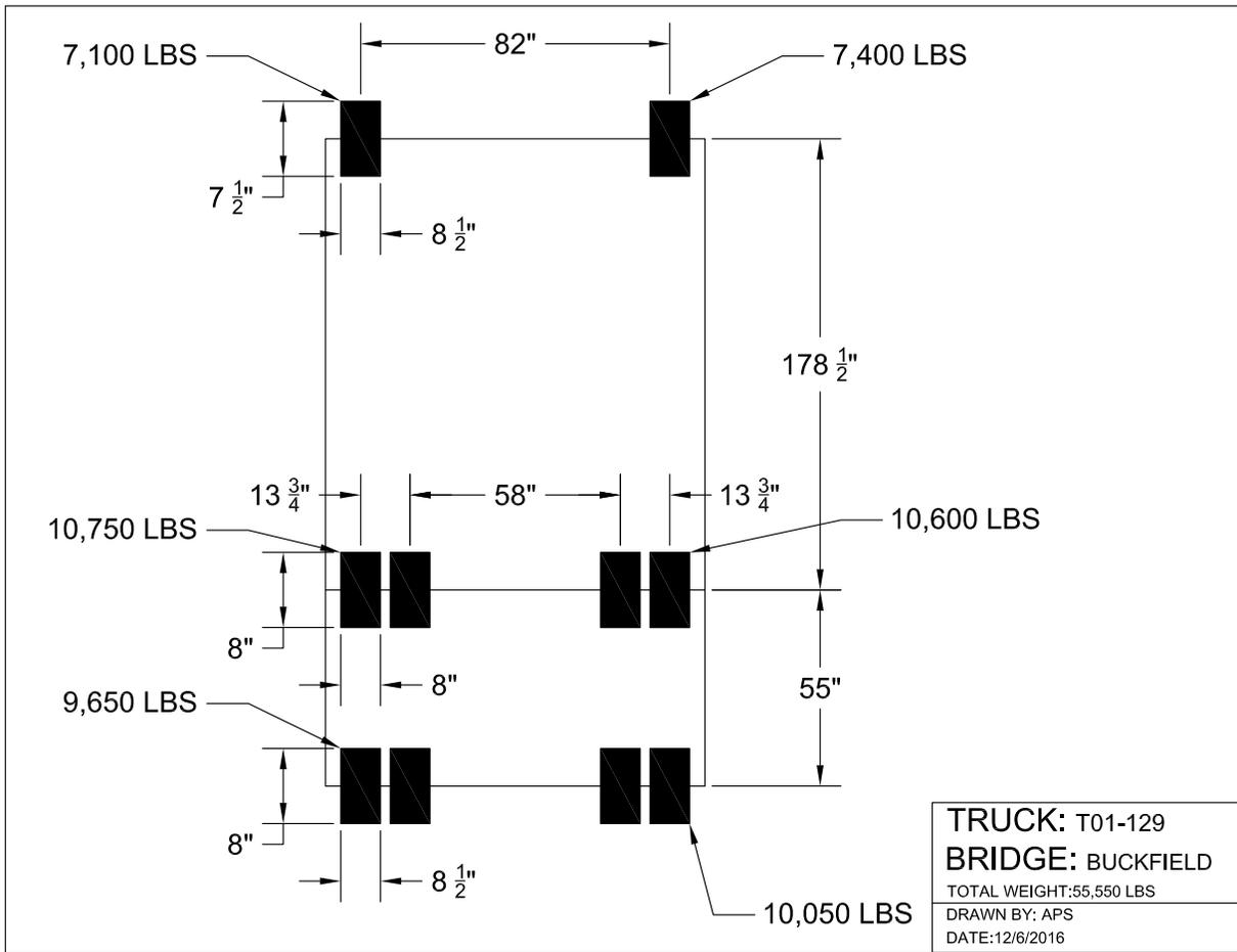
Figure 59: Buckfield No. 5452 Truck T01-129 loading
