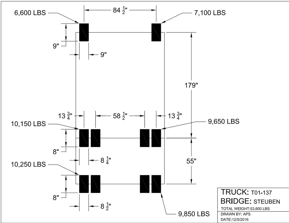
Figure 17: Steuben No. 3067 Truck T01-137 loading
