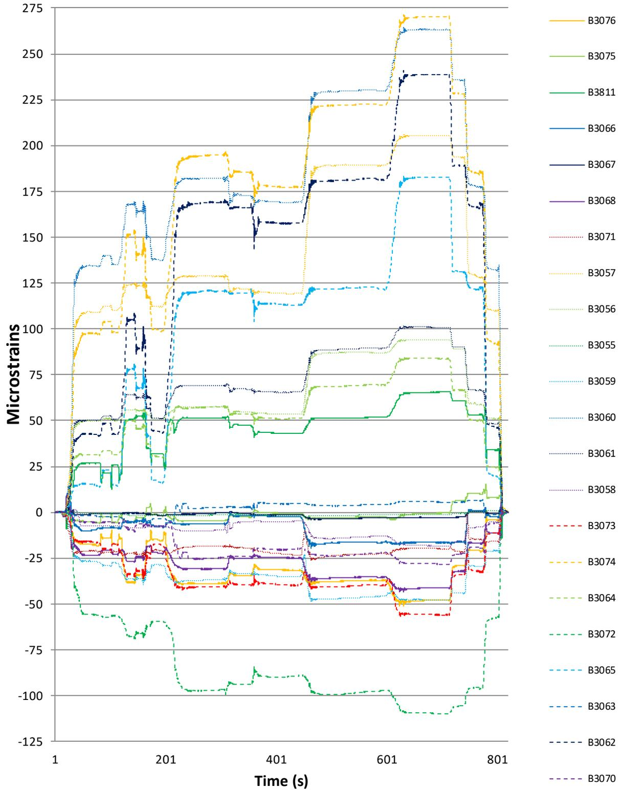
Figure 25: Steuben No. 3067- 4 trucks 2 lanes test 2 strains
