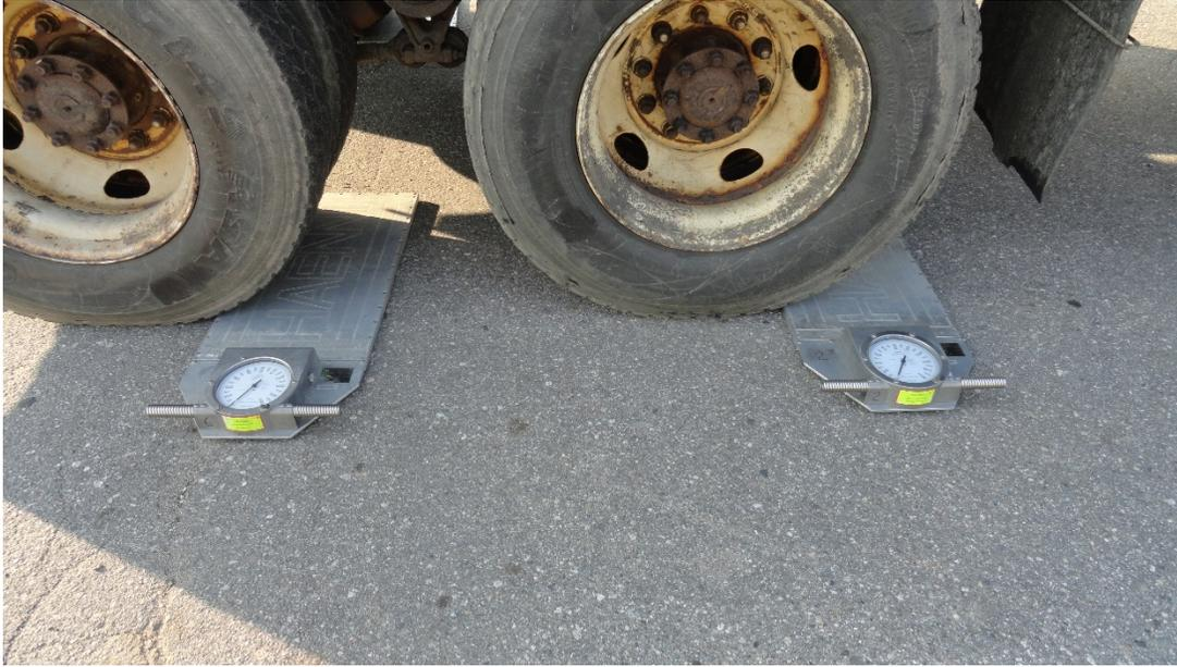
Figure 5: State highway patrol certified portable crane scales used to verify vehicle weight for each test
