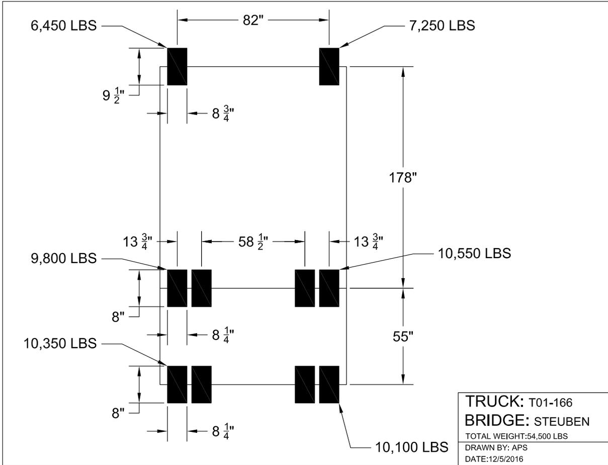
Figure 19: Steuben No. 3067 Truck T01-166 loading
