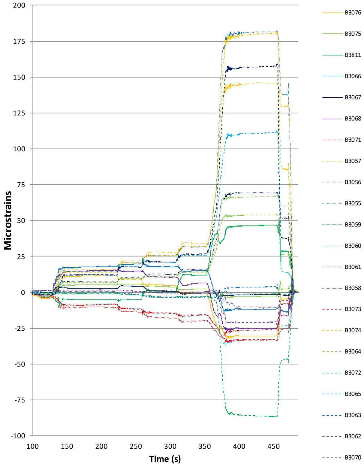
Figure 21: Steuben No. 3067- 2 trucks 2 lanes test 1 strain
