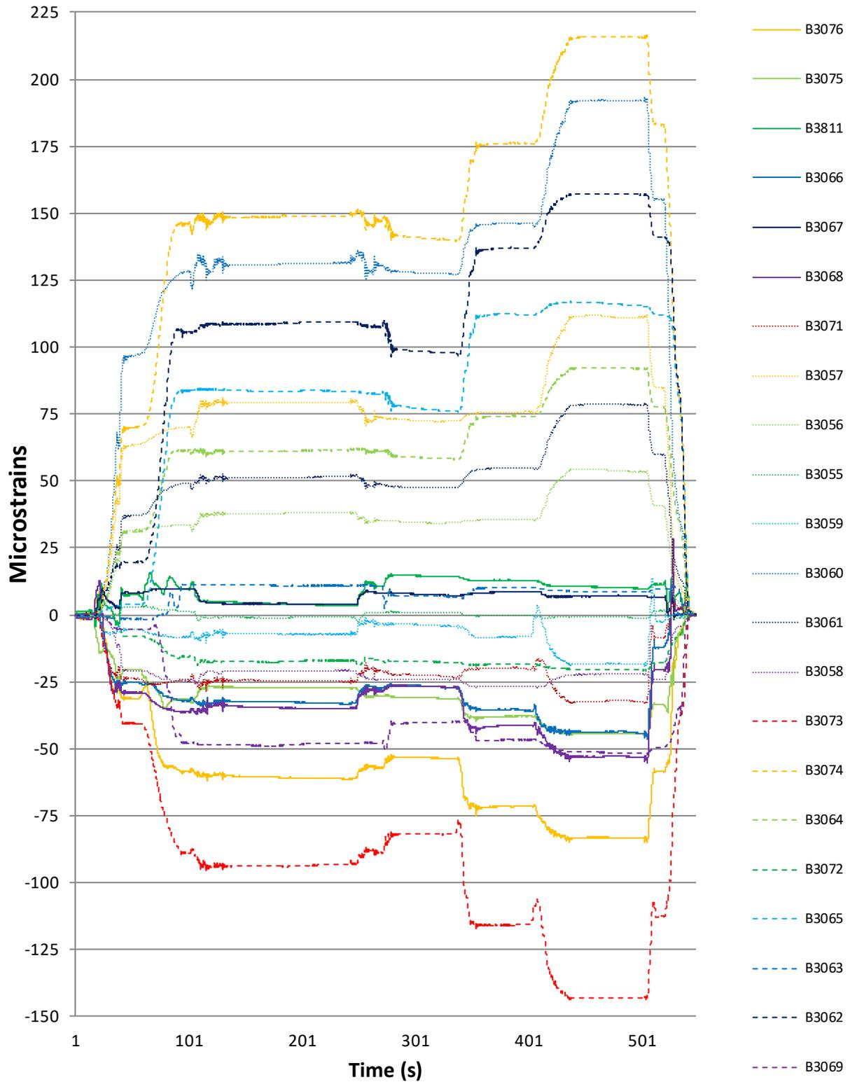
Figure 43: Pembroke No. 3884 - 4 trucks 2 lanes test 1 strains
