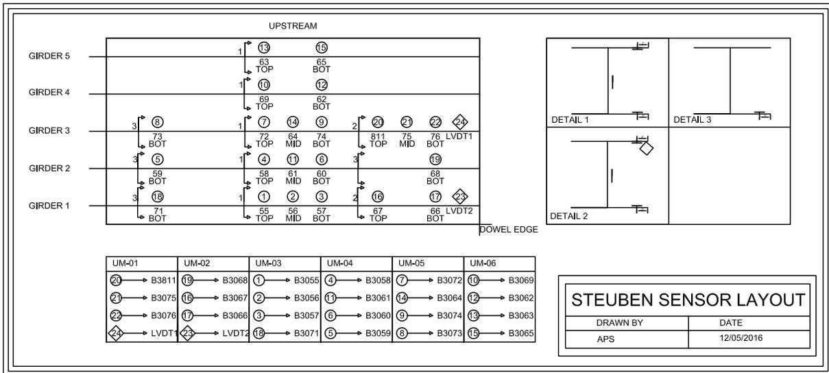
Figure 16: Steuben No. 3067 sensor layout
