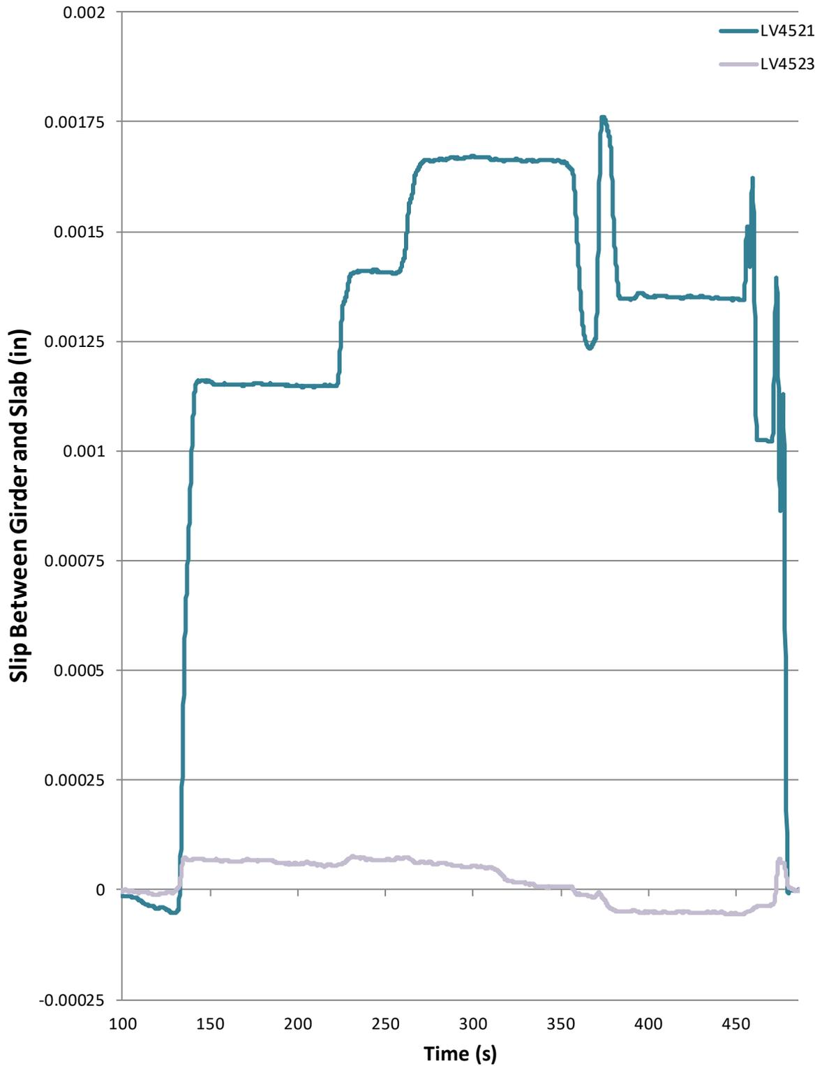
Figure 22: Steuben No. 3067- 2 trucks 2 lanes test 1 shear slip
