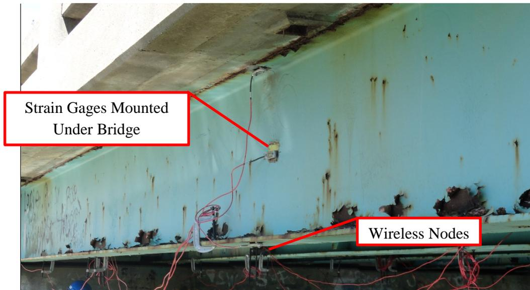
Figure 1: Typical strain sensors mounted under bridge connected to wireless nodes
