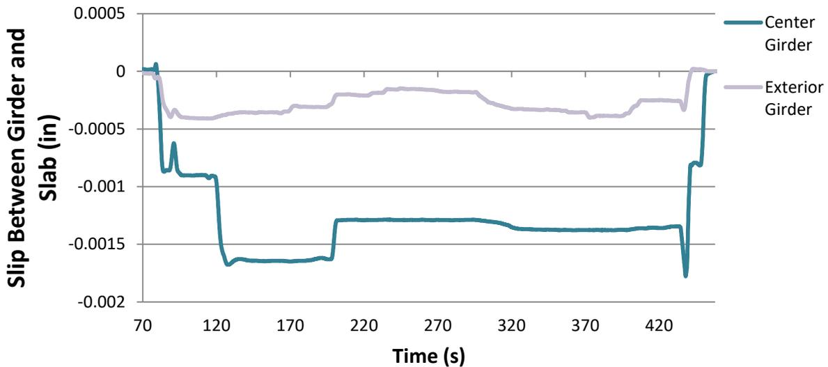
Figure 7: Pembroke No. 3884 - 4 trucks, 2 lanes, test 2, slip between girder and slab
