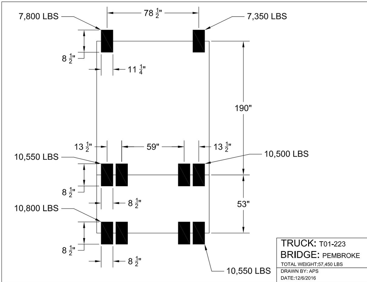
Figure 39: Pembroke No. 3884 Truck T01-223 loading
