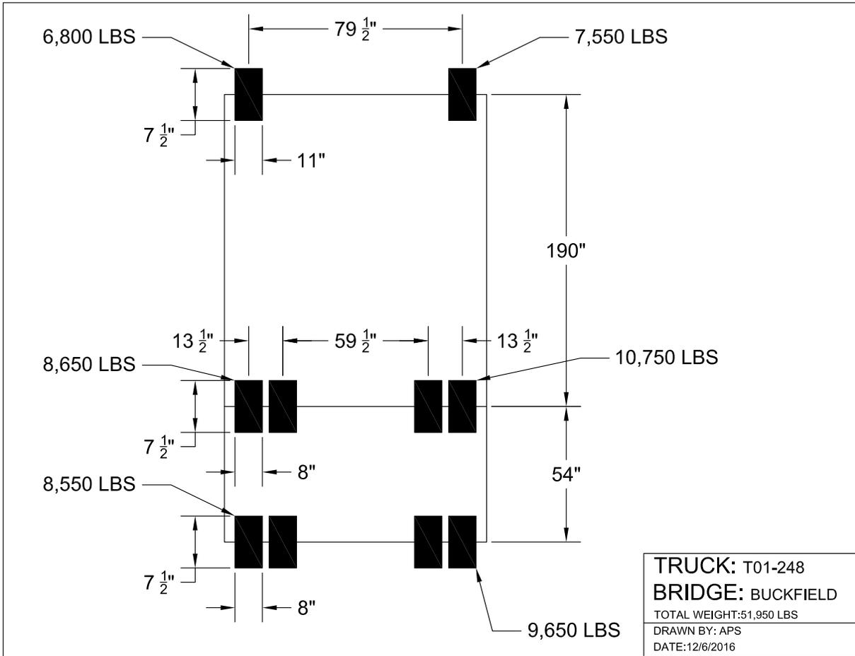
Figure 61: Buckfield No. 5452 Truck T01-246 loading
