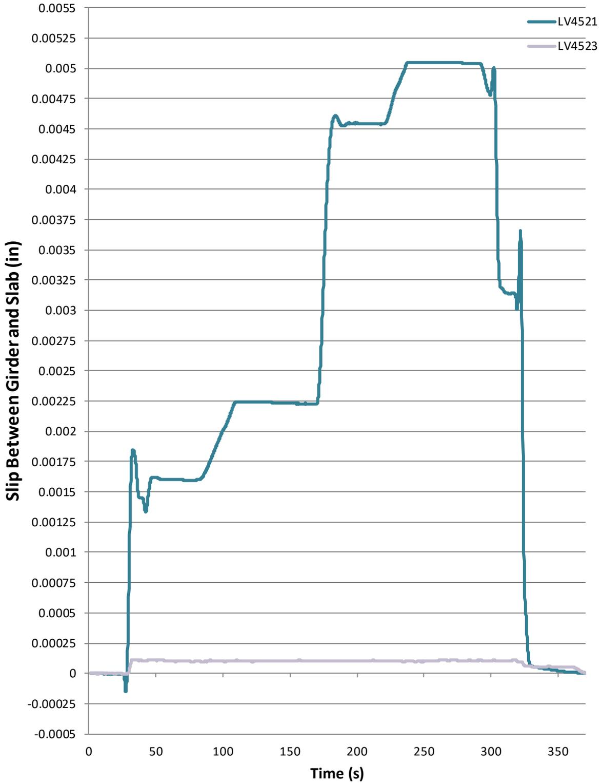
Figure 64: Buckfield No. 5425 - 4 trucks 2 lanes test 1 shear slip
