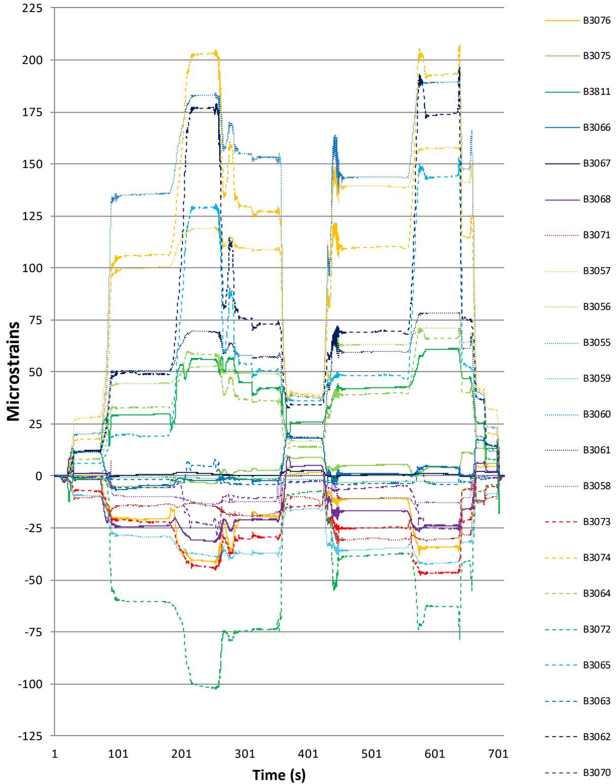
Figure 23: Steuben No. 3067- 4 trucks 2 lanes test 1 strains
