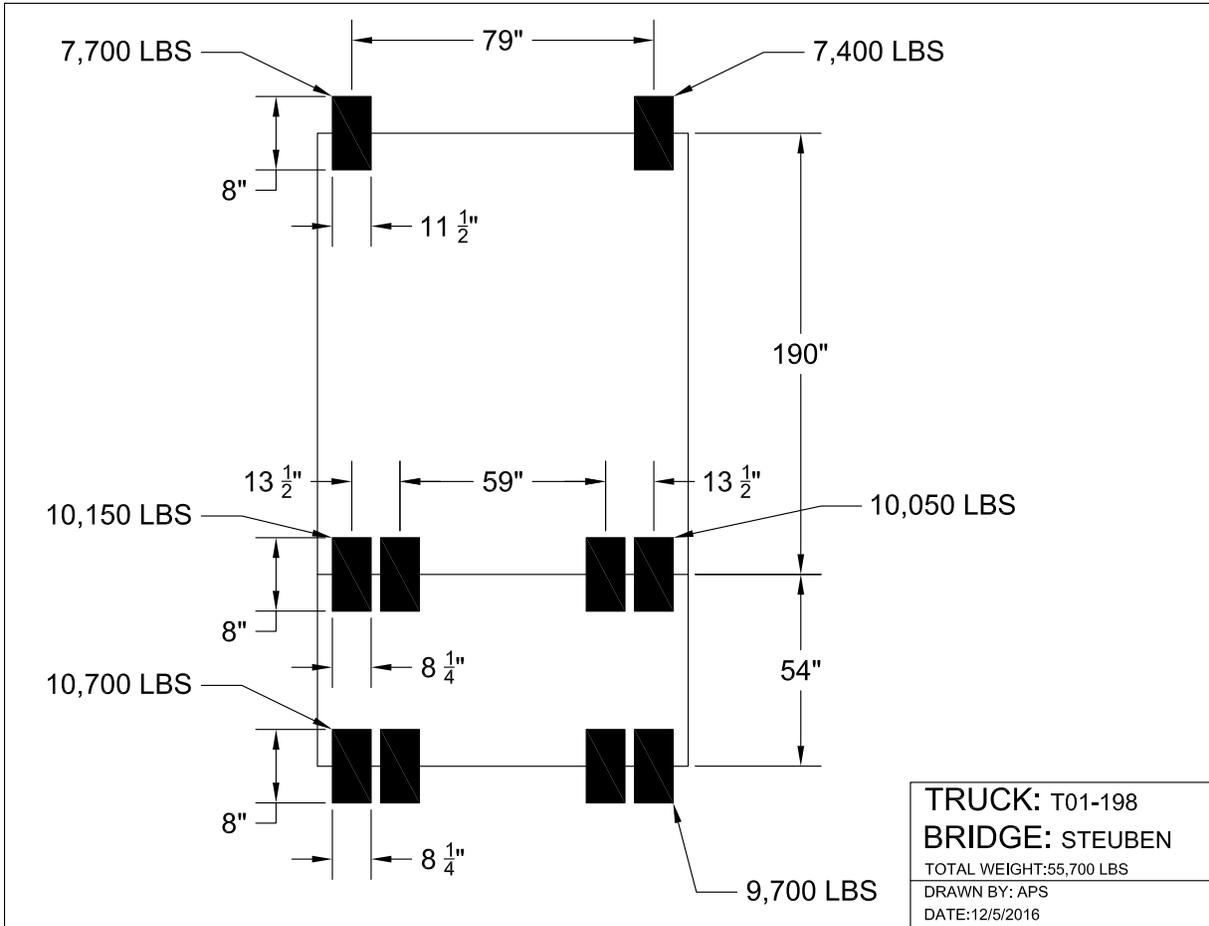
Figure 20: Steuben No. 3067 Truck T01-198 loading
