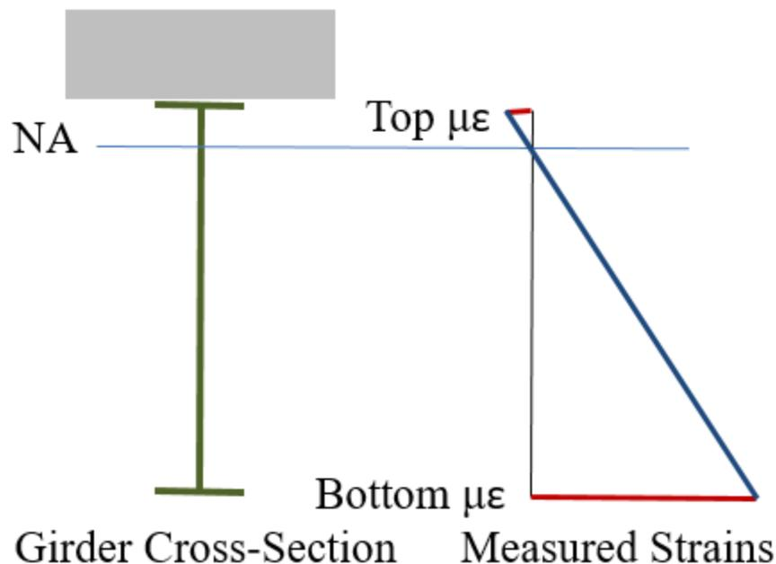
Figure 10: Typical linear strain distribution
