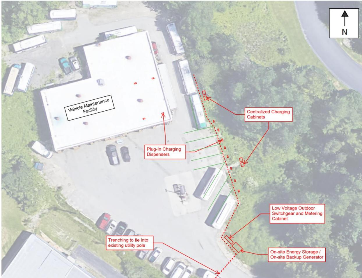
**Figure 13 13 Pomerleau St. Overnight Charger Layout Option**
