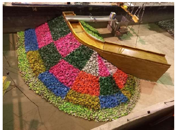
The completed test structure for Test Series A. Different colours were used for the trunk and roundhead areas.
