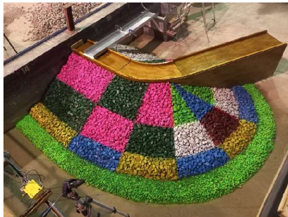
The completed test structure for Test Series B. the same zones were sprayed with different colours to distinguish between the two different test structures.
