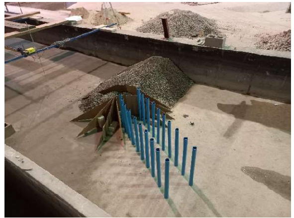
Placement of model core material. All model rock is shaped to the detail included on the templates. PVC pipes were fixed to the model floor to represent piles for the combi wall breakwater
