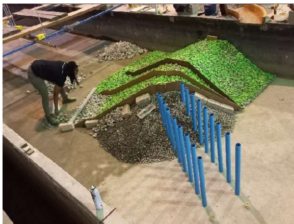
Placement and shaping of model underlayer rock. The upper surface of the underlayer were spray painted green for easy identification if exposed.
