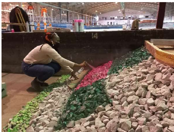
Finishing off the armour rock with different colours of spray paint. Zones were selected based on different areas of the structure.
