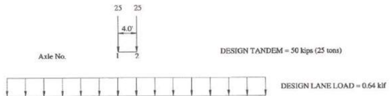
HL-93 Design Tandem with Lane Load
