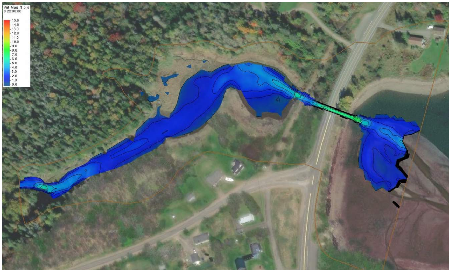
Figure E-3: Q 1.1 , 2% annual chance coastal storm event – Maximum Velocities at Low Tide (ft/s), Proposed Single Span Bridge Structure
