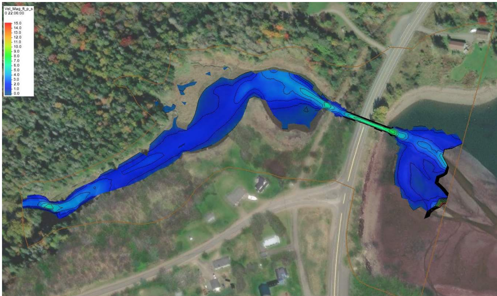
Figure E-2: Q 1.1 , Average Tides plus 4 ft SLR – Maximum Velocities at Low Tide (ft/s), Proposed Single Span Bridge Structure
