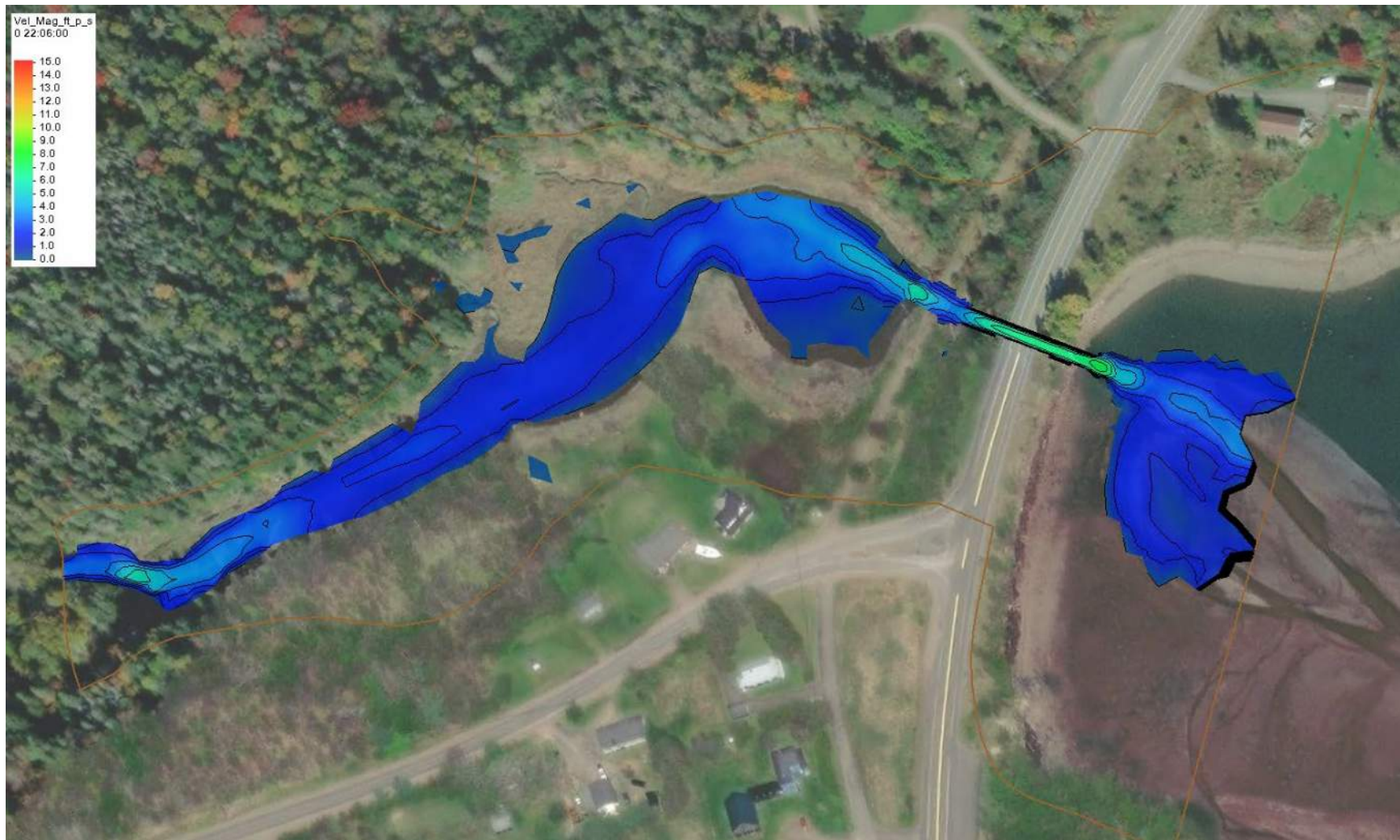
Figure E-4: Q 1.1 , 2% annual chance coastal storm event plus 4 ft SLR – Maximum Velocities at Low Tide (ft/s), Proposed Single Span Bridge Structure
