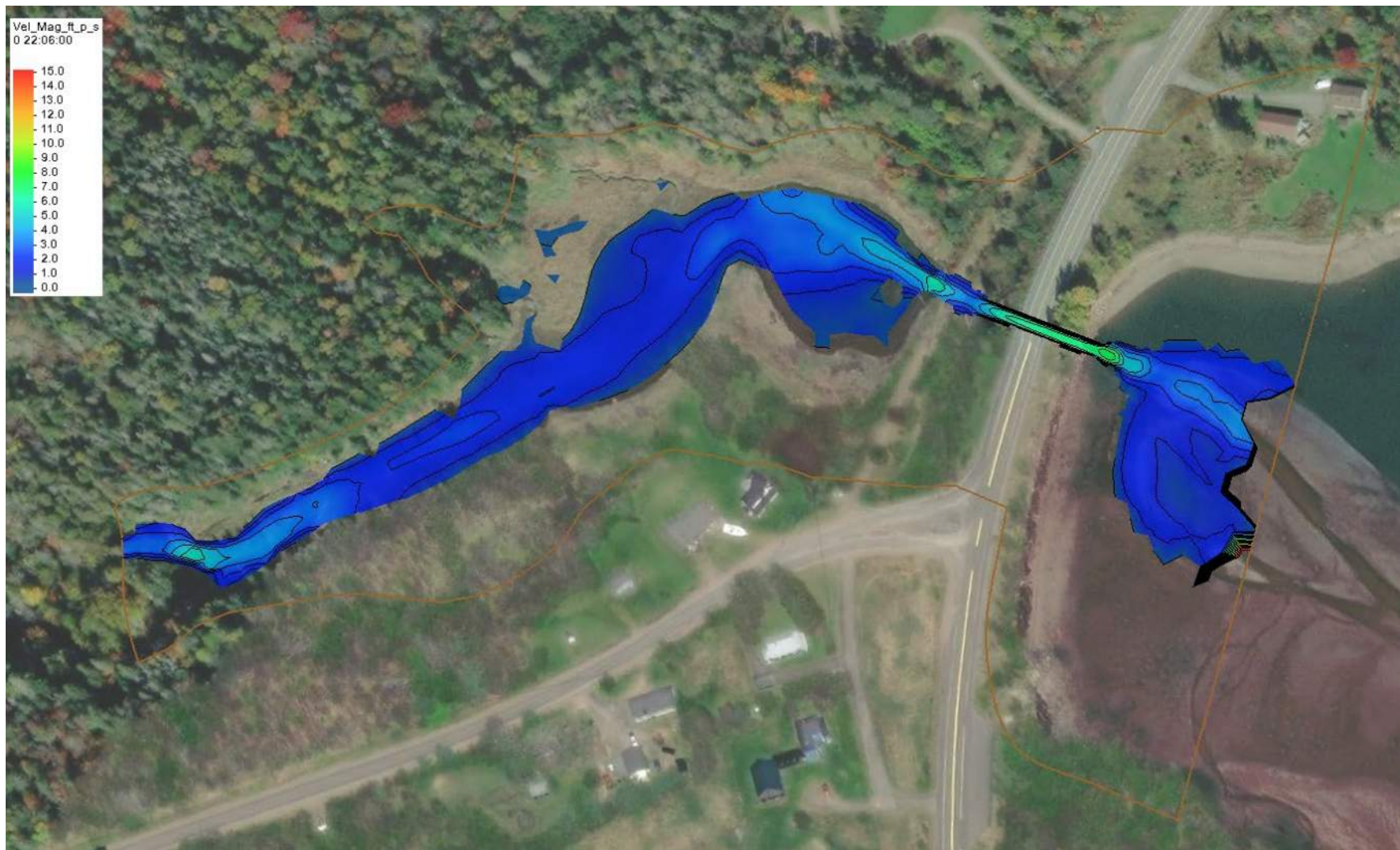
Figure E-1: Q 1.1 , Average Tides – Maximum Velocities at Low Tide (ft/s), Proposed Single Span Bridge Structure
