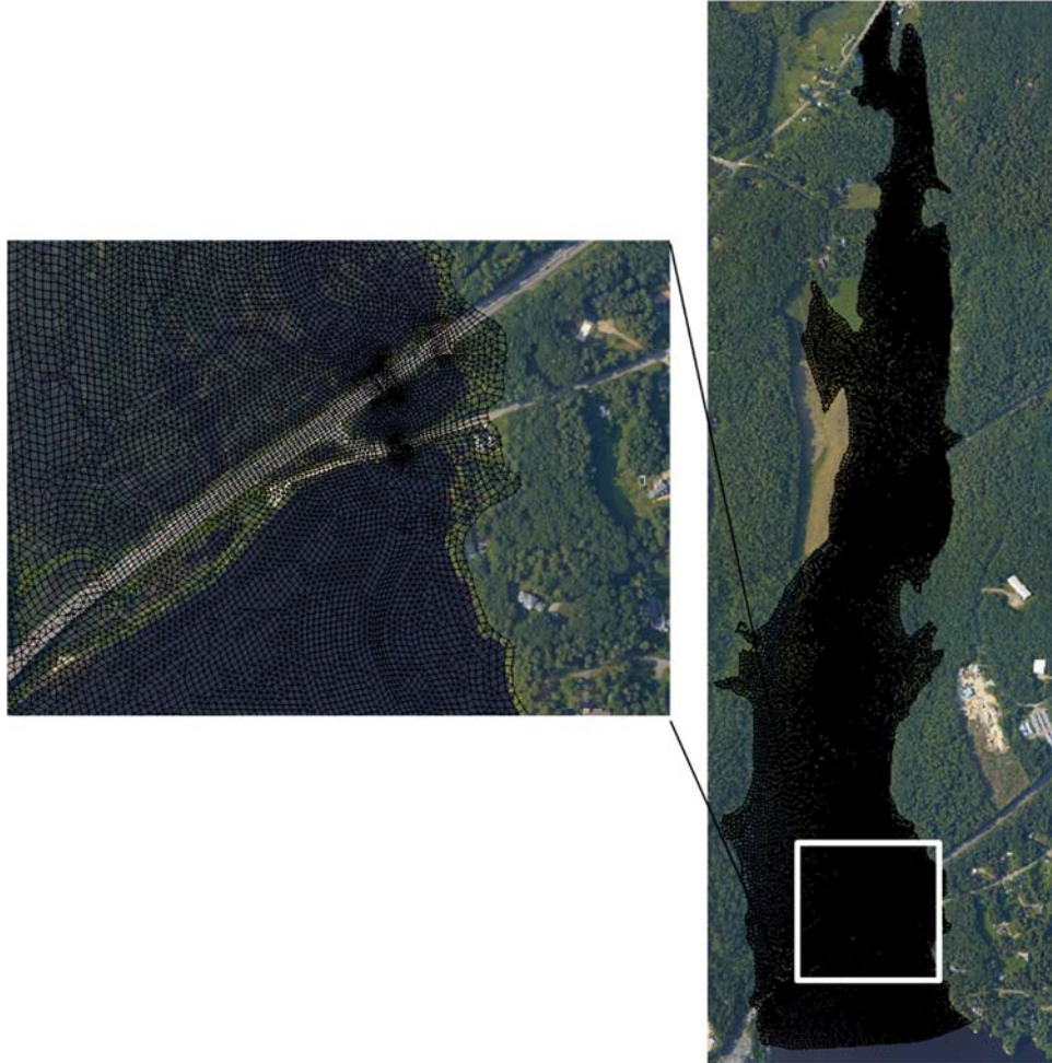
Figure 9 SRH-2D unstructured model mesh for Back River Marsh
