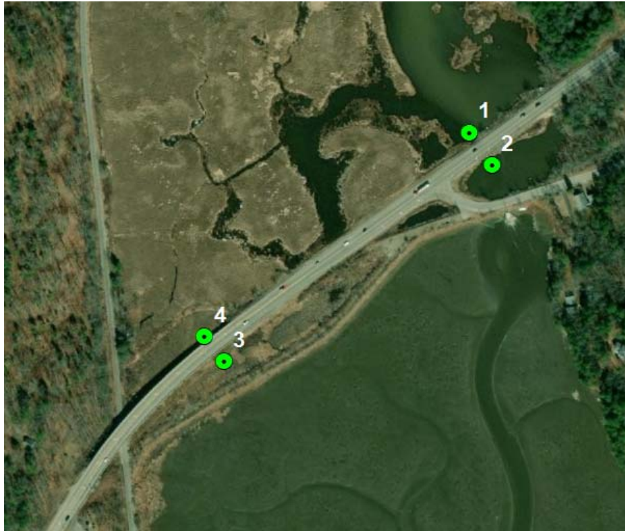
Figure 26 Map of velocity data extraction points for engineering calculations/scour analysis
