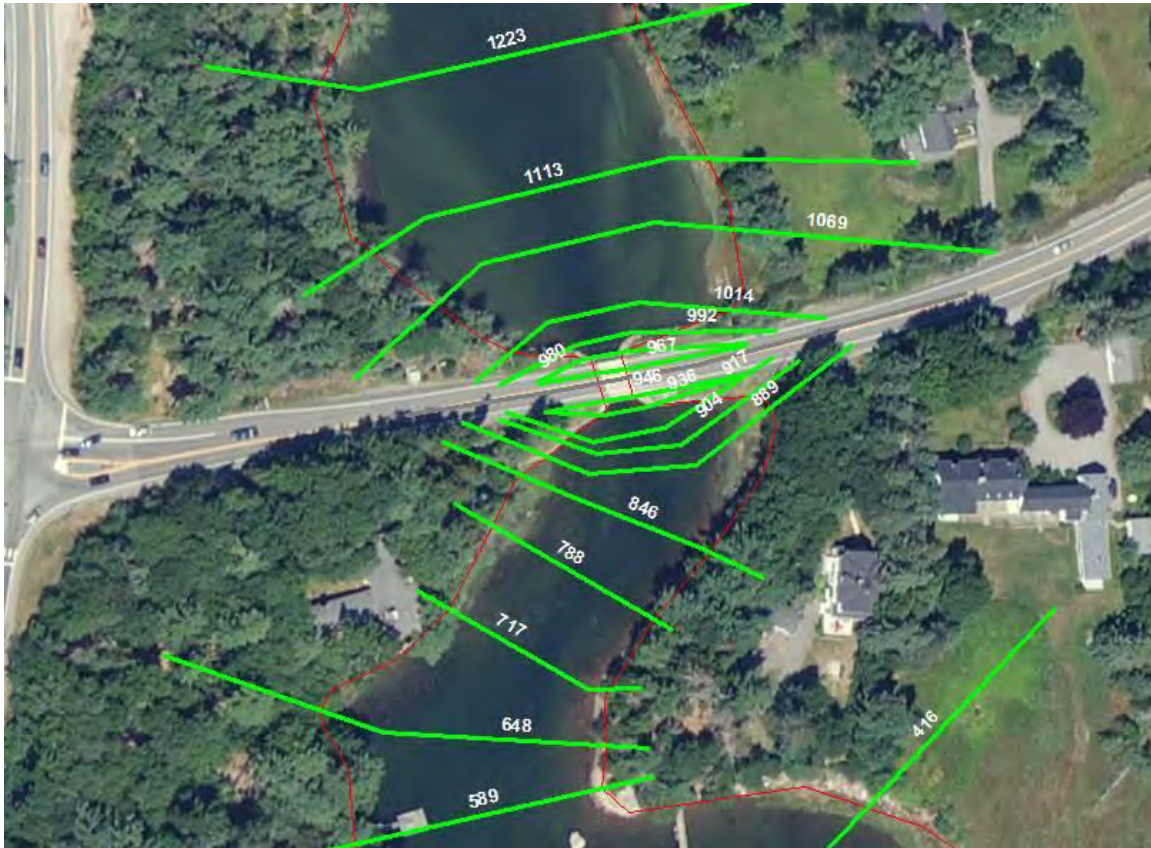
Figure 24: Hydraulic model layout in bridge area
