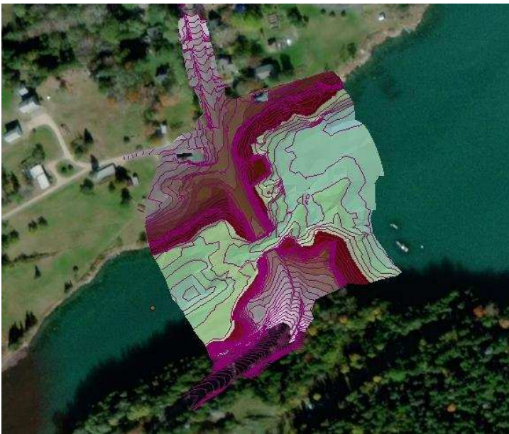
Figure 19. Bottom contours at bridge
