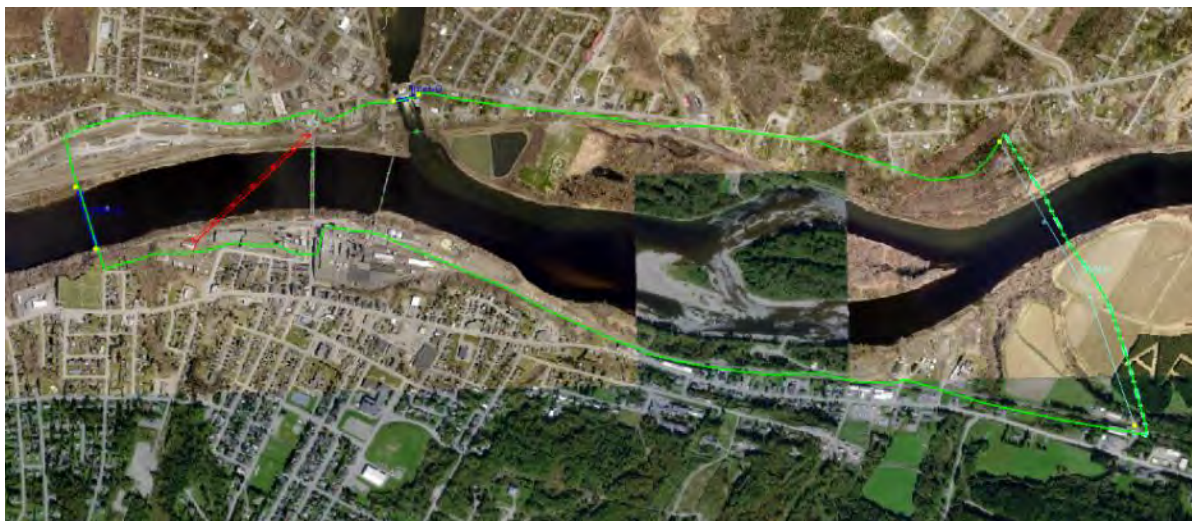
Figure 22. Model domain (green) shows boundaries and bridges. Proposed bridge location is shown in red, existing and utility bridges are shown in aerial photo.
