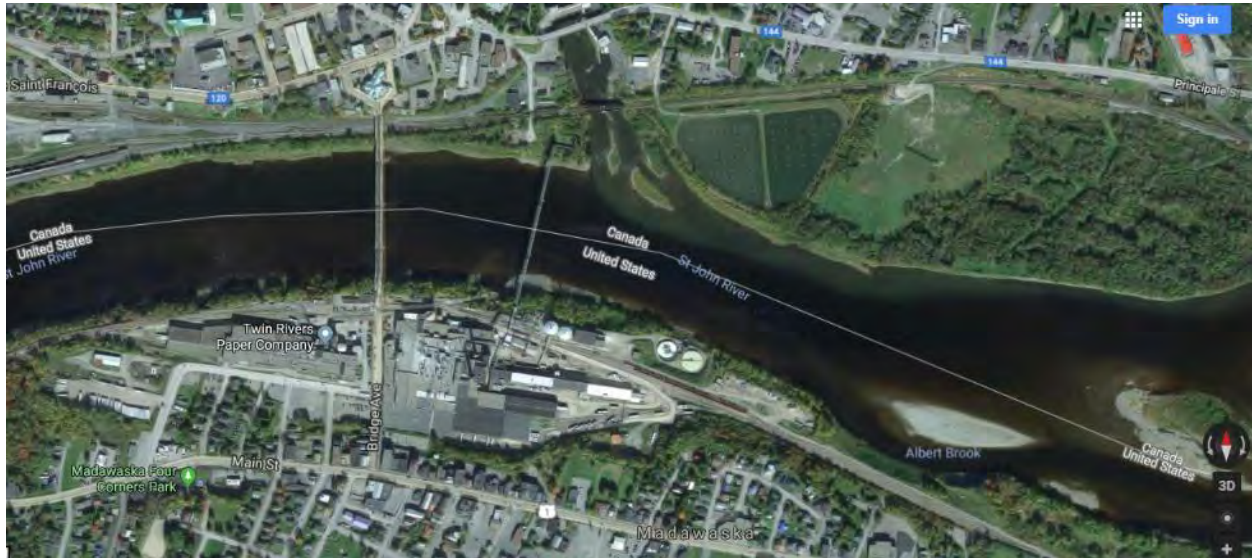
Figure 2 Existing bridge and utility bridge at project site. Note confluence of Madawaska River downstream, existing utility bridge, and several islands in downstream channel.
