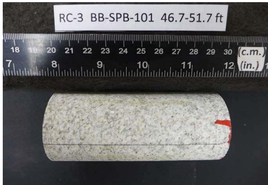
After cutting and grinding
