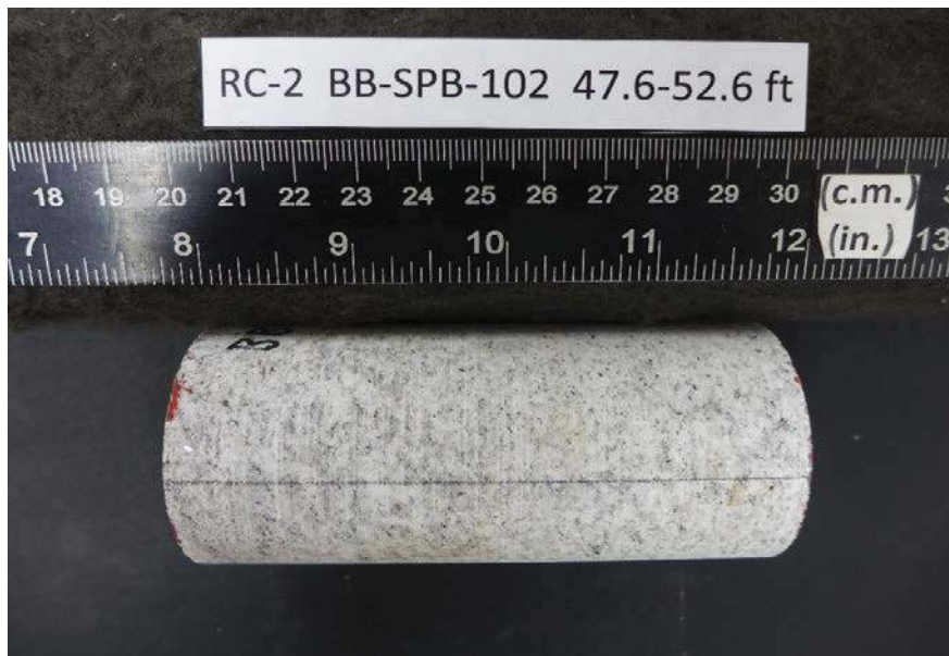
After cutting and grinding
