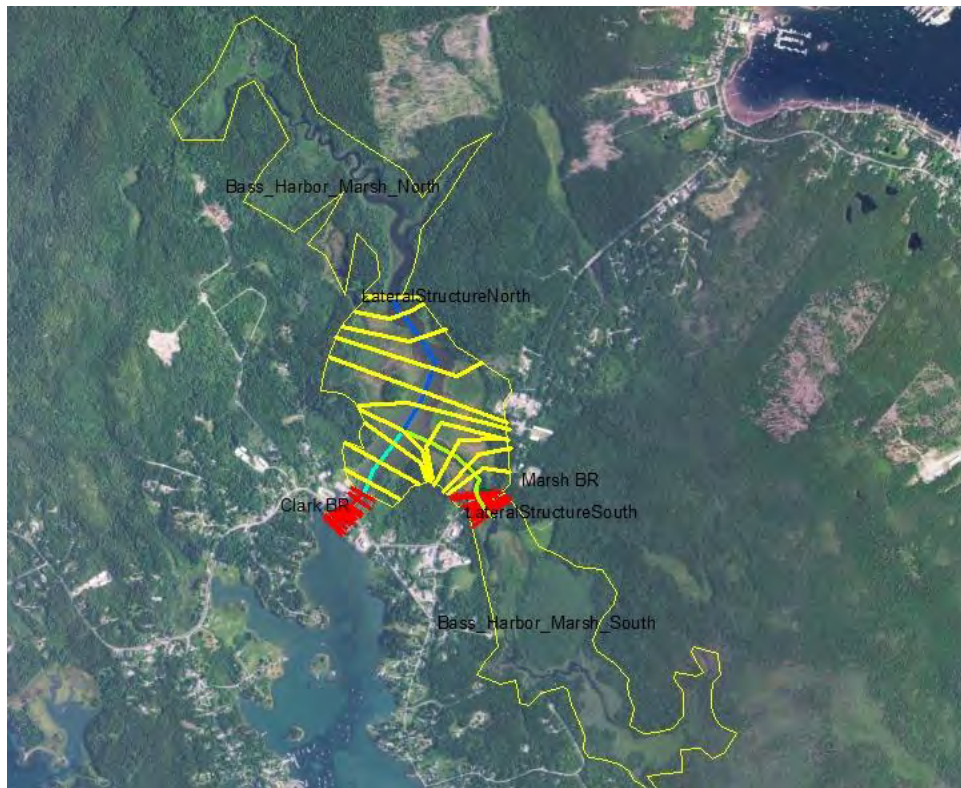
Figure 14: Marsh Bridge HECRAS model setup. Tidal boundary downstream of Clark Bridge. Survey in red at Clark Bridge and Marsh Bridge. Estimated river sections in yellow. Marsh storage areas outlined in yellow.
