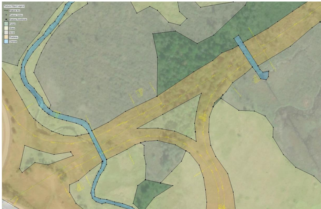
Figure 17: Detailed view of revised material roughness layout at culverts for the proposed condition
