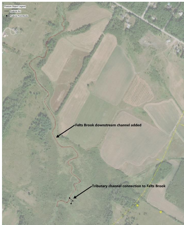
Figure 7: Layout of channels added to LiDAR data
