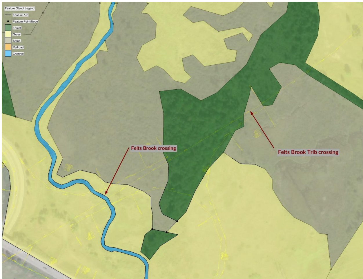
Figure 12: Roughness assignments at the structures for the existing condition
