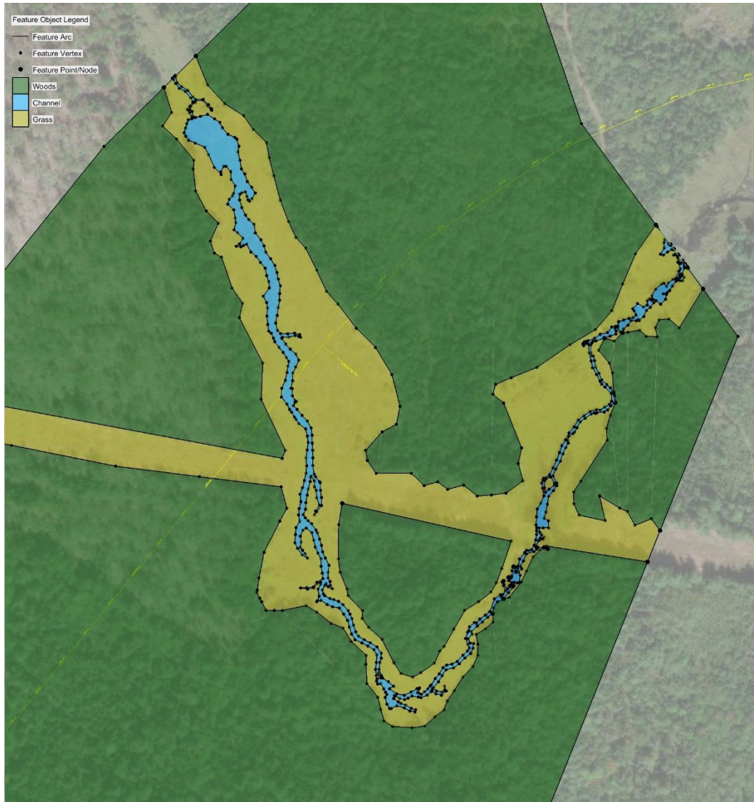
Figure 6: Roughness assignments for the existing model
