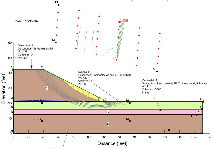
Material #: 5 Description: Bedrock Model: Bedrock Piezometric Line: 1
