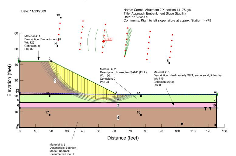
Name: Carmel Abutment 2 14+75 compacted fill.gsz Title: Approach Embankment Slope Stability - Onsite Fill soils compacted
