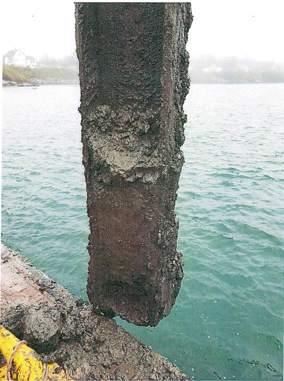
Photo 7: Soil adhered to HP12x53 steel H-pile probe.
