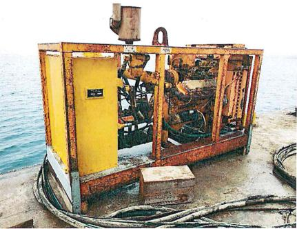
Photo 6: H&M Model 3208T vibratory hammer used to advance HP12x53 steel H-pile probe.
