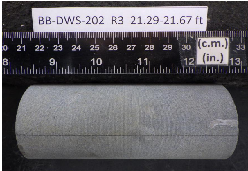
After cutting and grinding
